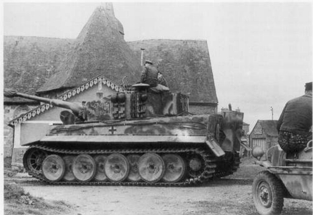
One of the eight Tiger issued to the 1.Kompanie/schwere SS-Panzer Abteilung 101 in January 1944. The Heckzurrung (rear travel lock) on the right rear is just visible and the MP Stopfen (Pistol port) on the left rear of the turret has been deleted. (Bundesarchiv)
