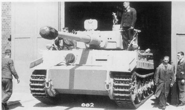
In early May 1943, this new Tiger left the assembly line at the Henschel works in Kassel. The loader's periscope, spare track links on the turret and the Nebelwurfgeräte (smoke candle dischargers) are typical for Tigers produced between March and June 1943. The Tiger is painted in a base coat of Dunkelgelb (dark yellow) (RAL 7028). The outer set of road wheels have not been mounted and narrow transport track is fitted for rail transport. (Author)
