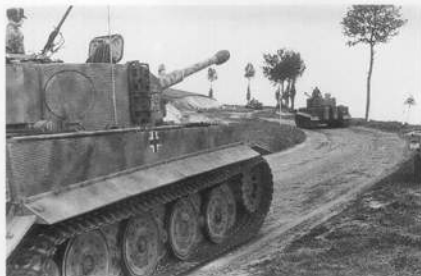
Tigers, tactical numbers 224 and 223 approach the Normandy front. These Tigers were delivered in April 1944 to the 2. Kompanie/sSS-PzAbt. 101. The anti-aircraft machine gun on the commander's cupola is clear. (Bundesarchiv)
