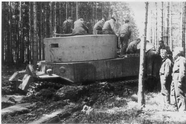
The VK 45.01 (P) was a totally new design, with a new aircooled motors designed by Porsche, Siemens electric drive train and horizontal torsion bar suspension. Despite the clever concept too many components were new and untested. The urgency of the production schedule would not tolerate the problems that occurred with these untested components, therefore, the production was cancelled. (Spielberger collection)
