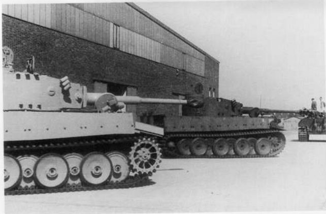
Another new Tiger, the 8th scheduled for completion in May 1943, still has the red oxide primer undercoat. In the distance is a Panther chassis also in red oxide primer. Panthers were assembled alongside Tigers at Henschel for a period in 1943. (Author)
