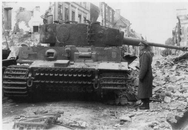
Tiger, tactical number 112, of the 1. Kompanie/sSS-PzAbt. 101 was destroyed during the Normandy battles. Clear in the photograph are features that were introduced after December 1943 and January 1944; the cut out hull side extension which allowed free movement for the shackle, the centre mounted Bosch headlight, the small muzzlebrake, and the chevron faced track. This Tiger has the steel rimmed wheels showing that it was one of the Tigers delivered to the sSS-PzAbt. 101 in April 1944. (Bundesarchiv)
