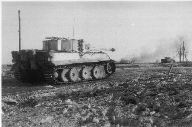
Starting in July 1943 the new turret was introduced. The Prismen-spiegelkuppel (Commander's cupola) was fitted. A M.P. Stopfen (plug type machine pistol port) replaced the M.P. Klappe on the left rear and the extractor fan was moved to an armoured housing on the centre line over the 8.8cm KwK breech. This Tiger was built in July or August 1943 so does not have Zimmerit anti-magnetic coating. (Bundesarchiv)
