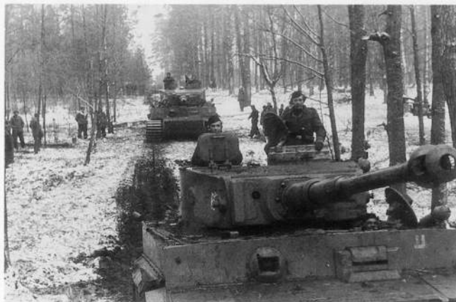
This Tiger is one of the 5 replacements shipped to the 13.Kompanie/SS-Panzer Regiment 'LSSAH' in July 1943. The periscope for the loader and the spare track link holders on the turret were features introduced from March 1943. When the 'LSSAH' returned to the West in July 1943 this Tiger was transferred to 'Das Reich' whose symbol is on the left side of the superstructure front. (Bundesarchiv)
