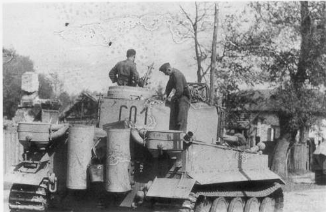
The 11.Kompanie/Panzer Regiment 'Grossdeutschland' received 14 Tigers in early July 1943. The two holes in the alignment plate for the cranked inertia starter show that a Maybach HL230P45 motor is fitted and the Fgst Nr is above 250251. The three companies of the III. Abteilung/Pz.Rgt. 'GD' used the letters A, B and C as the first digit of their tactical numbers. (Bundesarchiv)
