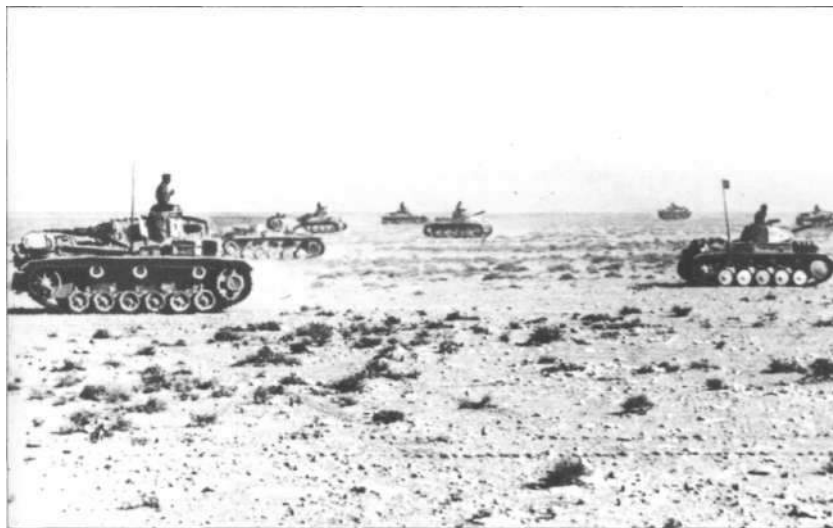
Mk IIIs moving forward towards the battle at Solium. The original armour of the Mk III was found to be incapable of offering protection against the 2-pdr during the French campaign and was steadily improved, both in production (to a maximum of 90mm) and in the field, with pieces of plate and spare track. The L/42 gun was only a low-velocity weapon but fired a useful high-explosive round and outranged the 2-pdr. (IWM MH5588)
