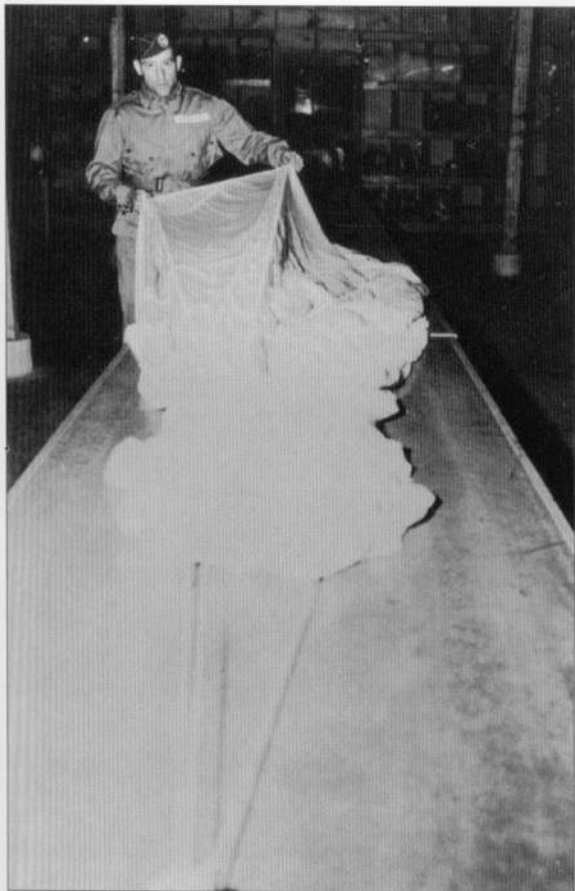
An instructor spreads out a chute in the packing shed, demonstrating to paratroopers the proper way to pack it. The shot bag just visible in the foreground holds the parachute lines straight and prevents them from tangling as the chute is packed. (Airborne & Special Operations Museum, Ft. Bragg, NC)
