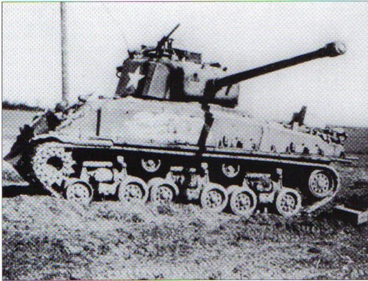
Abrams' third tank during the European campaign was this M4A3E8 named Thunderbolt VII, seen here in the spring of 1945 after it has been modified with appliqué armor. Abrams had a .30 cal. machine gun added in front of the cupola that was easier to use than the awkwardly located .50 cal. machine gun. (Patton Museum)
