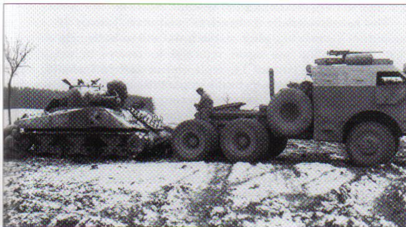
The attack to relieve Bastogne was costly, with the 4th Armored Division losing 49 medium tanks during December 1944. Here, a M26 'Dragon Wagon' tractor is used to recover a M4 knocked out by two anti-tank gun rounds that had penetrated the side near the star marking. (NARA)
