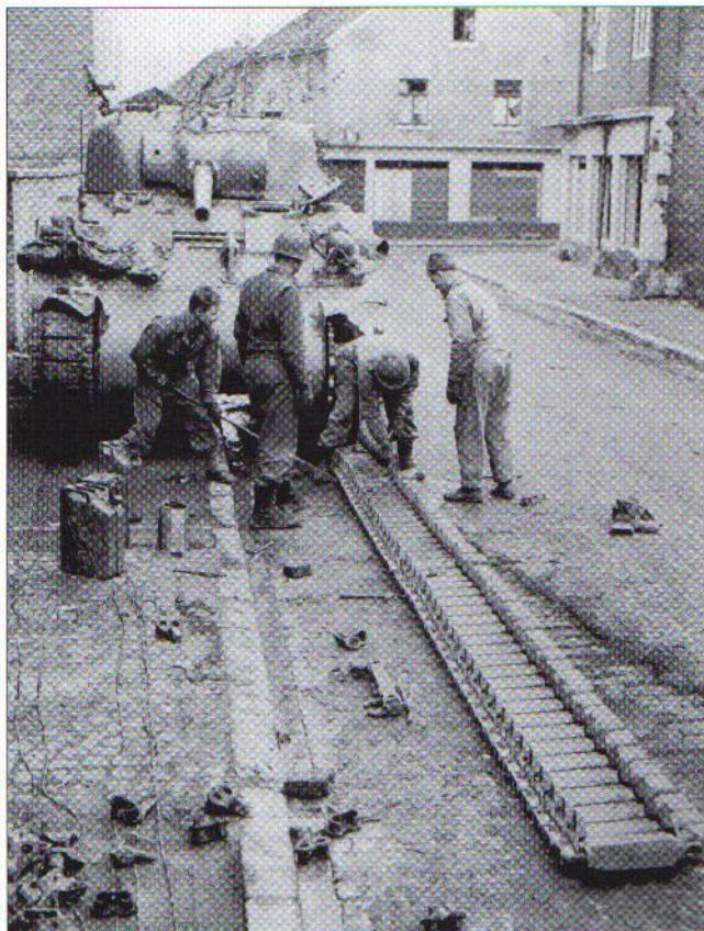
The wet autumn of 1944 and the accompanying mud forced the adoption of extended end connectors to M4 medium tanks to improve their traction. Here, the crew of a M4 medium tank have already removed the left track of their M4 tank and replaced the normal end connectors with the wider 'duck-bill' extended end connectors while in Baesweiler, Germany on December 5, 1944. (NARA)
