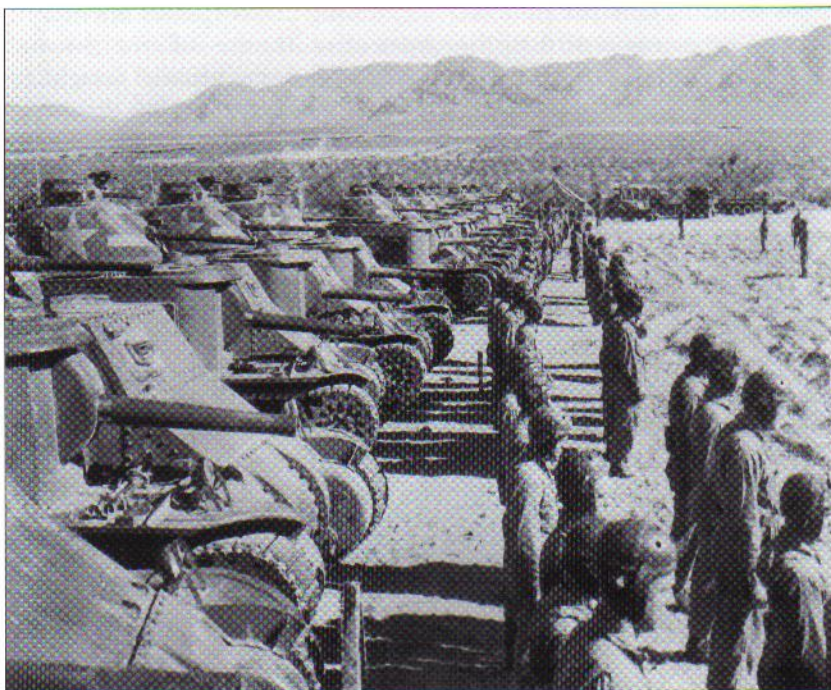
Most of the initial armored divisions spent time at the Desert Training Center in the Mojave Desert in southern California in 1942 and 1943 to conduct large-scale training and exercises. The medium tank companies were equipped with the M3 medium tank like these, but they were gradually replaced by the M4 medium tank starting in 1942. (NARA)
