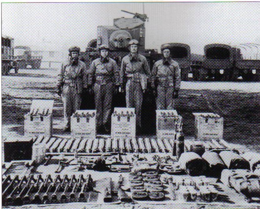
A tank crew from the 2nd Armored Division pose for a photo in front of their M3 light tank at Fort Benning, Georgia in 1942 with all the vehicle stowage and ammunition displayed. This provides some idea of the considerable amount of equipment and stores carried even in a small vehicle like the M3 light tank. (NARA)
