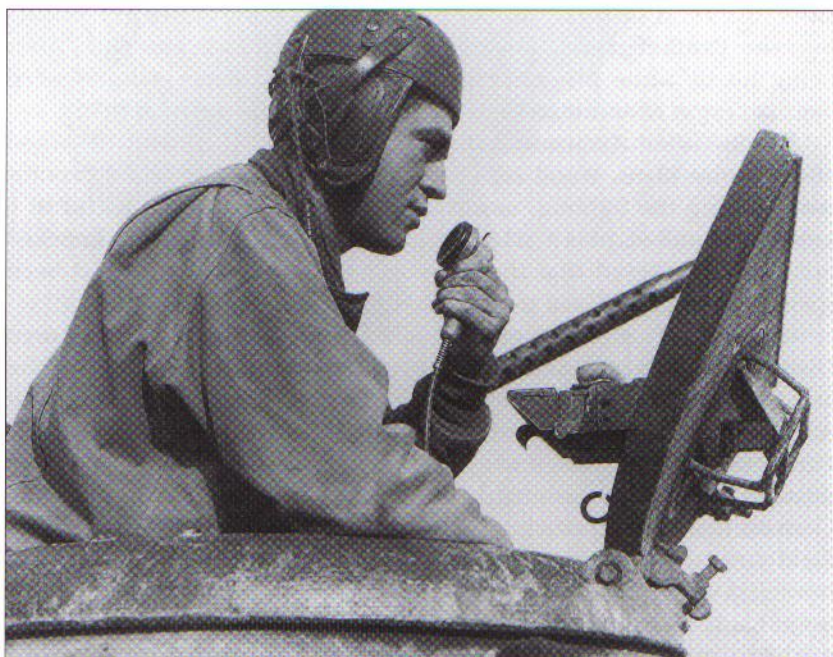
Capt. J. F. Brady was a company commander of Co. A, 35th Tank Battalion, 4th Armored Division and is seen here on October 2, 1944 talking with his crew over the vehicle microphone. In front of him is the periscopic sight, his only means of vision when the hatch was closed. (NARA)
