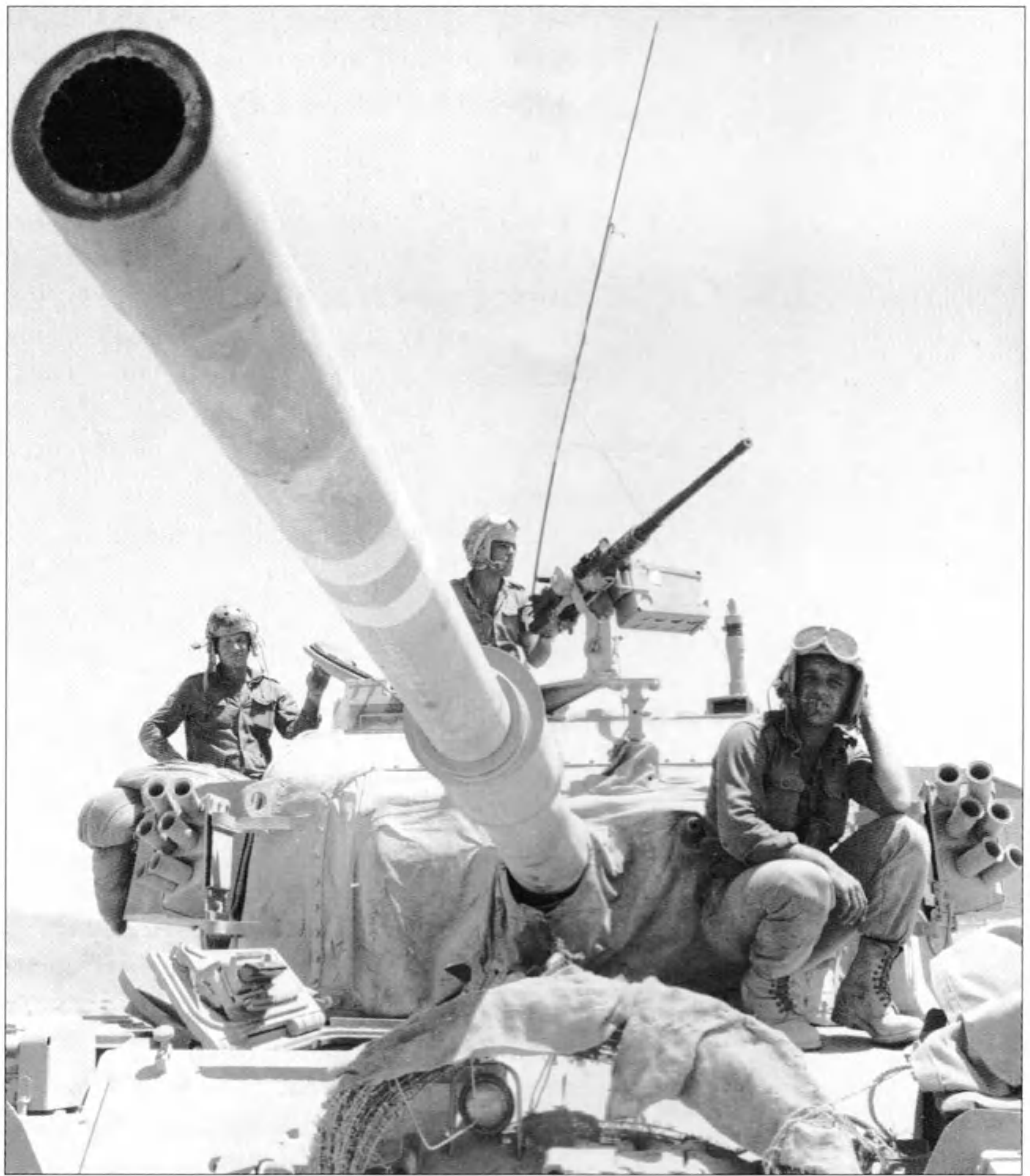
The first major modification to Israeli Centurions was the fitting of the L7 105mm gun in place of the 20-pounder. It proved decisive during the stunning victory in the Sinai in the Six Day War of June 1967. Here, the crew of a Centurion Mark 5 make their final preparations just days before the outbreak of war. (IDF)
