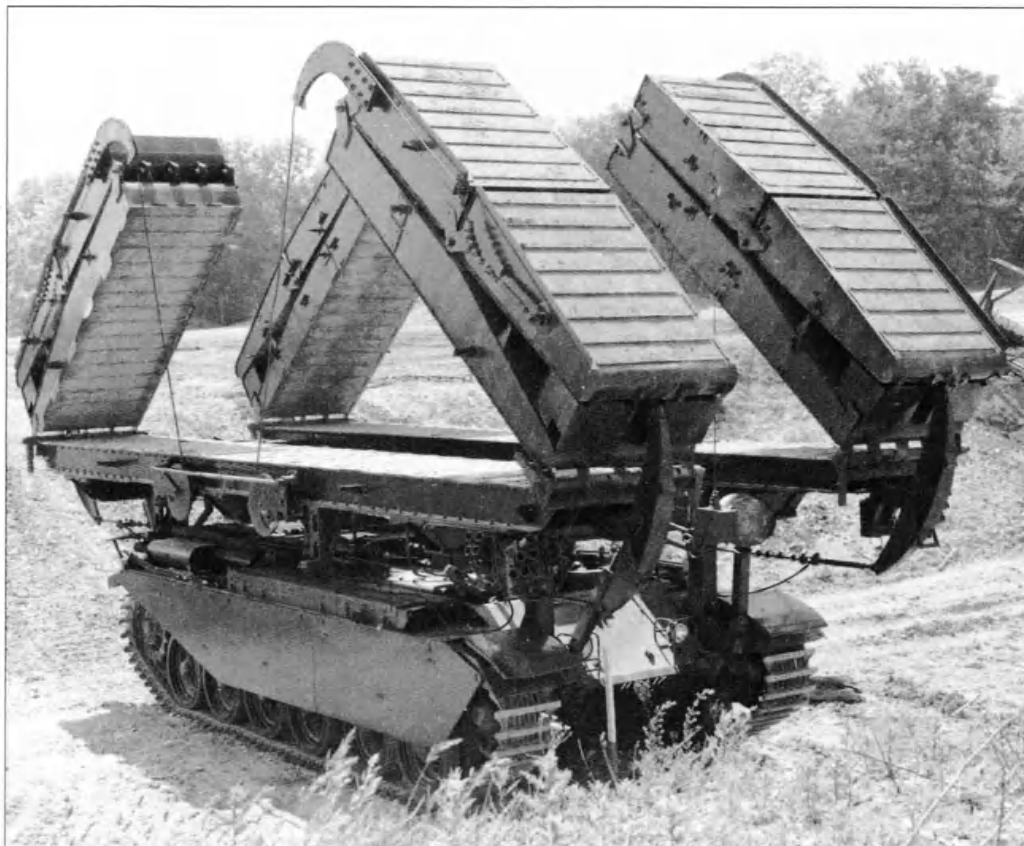
A Centurion ARK deploys its ramps to form a 75-foot-long bridge across a wide anti-tank bridge. By acting as a central pier in this way, the ARK also forms a means for tanks to negotiate obstacles such as steep-sided earth banks or sea walls.
