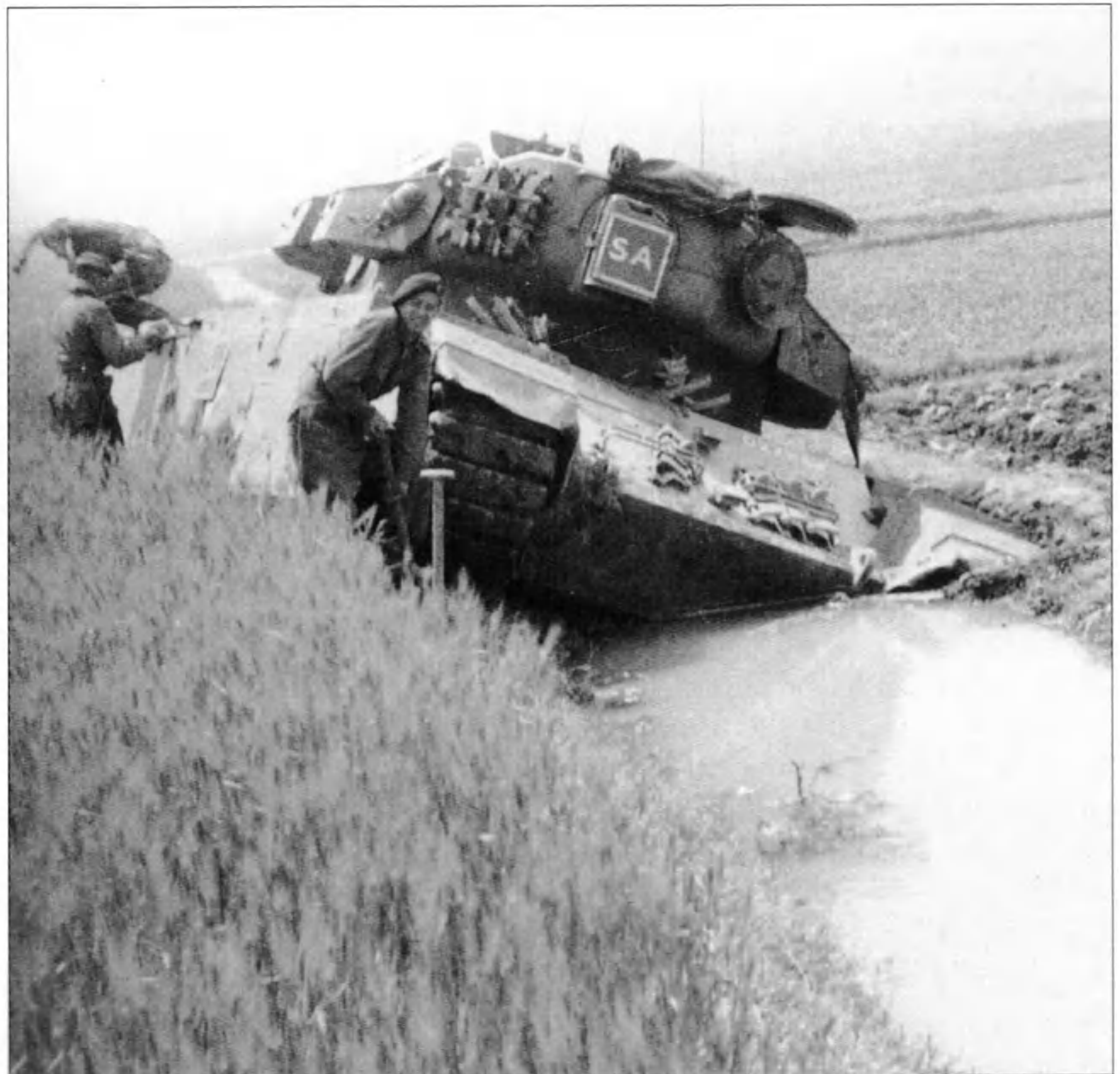
The Korean terrain was totally inhospitable to armoured operations with chains of rugged mountains interlaced with raging rivers, while any flat ground was used for the cultivation of rice. All proved extremely difficult to negotiate on foot let alone on tracks. Of all the obstacles, the glutinous rice paddies were a constant hazard for the tanks such as this bogged Centurion Mark 3 of B Squadron Headquarters Troop, 8KRIH.
