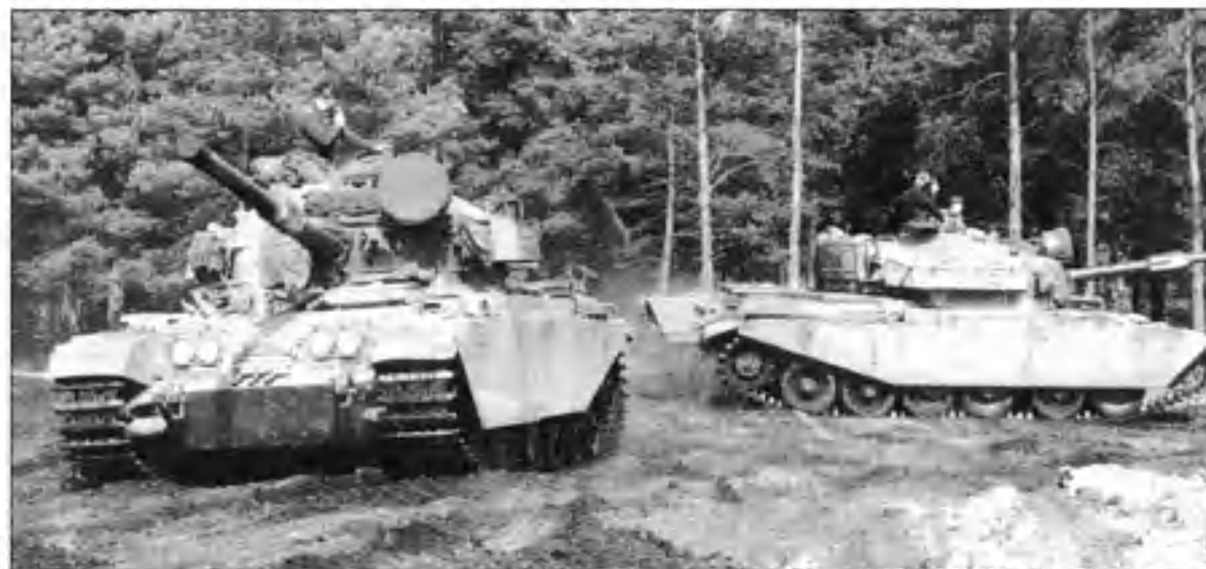
The final model of Centurion that began as a Mark 3 was the Mark 11. It featured all the progressive improvements that were applied to the Centurion gun tank during its many years of service with the British Army including up-armouring; up-gunning; night fighting equipment; ranging gun; and an auxiliary fuel tank for increased operational range. These Centurions belong to the 4th Canadian Mechanised Brigade Group during an exercise in West Germany in 1966.
