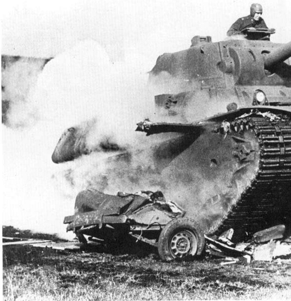
Right The Heavy Tank M6A1, weighed 56.48 tons was armed with a 3 inch gun also a 37mm and four MGs. It was never used in action and in December 1944 the series was declared obsolete. (TM)
