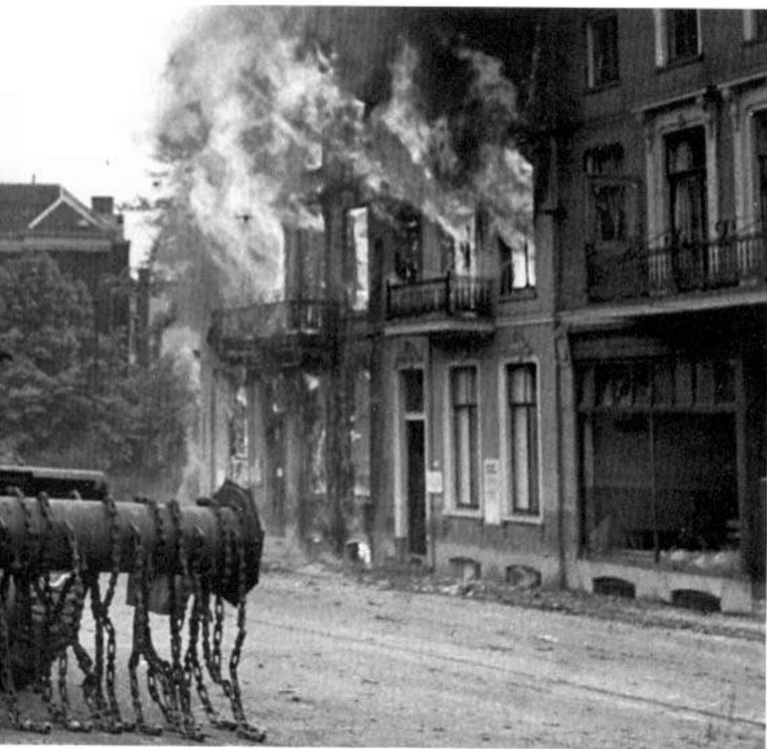
Left: The most successful type of minefield gapping equipment was the British Sherman Crab also operated by US troops. It had forty-three flailing chains on a rotor which beat the ground just ahead of the tank, exploding mines. (TM)
