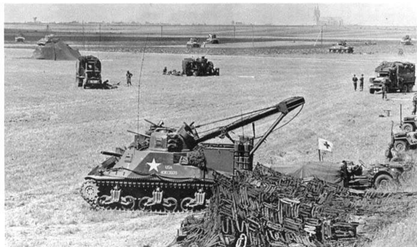
Above A tank unit base, belonging to 7th Armored Division, near Chartres, France, 18 August 1944. Note the M31B1 Tank Recovery Vehicle (based on the M3 medium tank), the medical post, various echelon vehicles, plus well-spread out Shermans in the background. (TMA)
