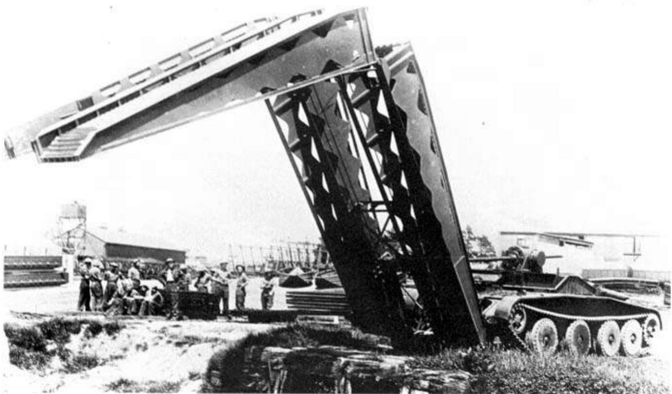
Below: A Covenantan bridgelayer launching its 30ft folding bridge. They were used mainly for training and development work, but a few were used by the Australians in Burma, 1942. (TM)
