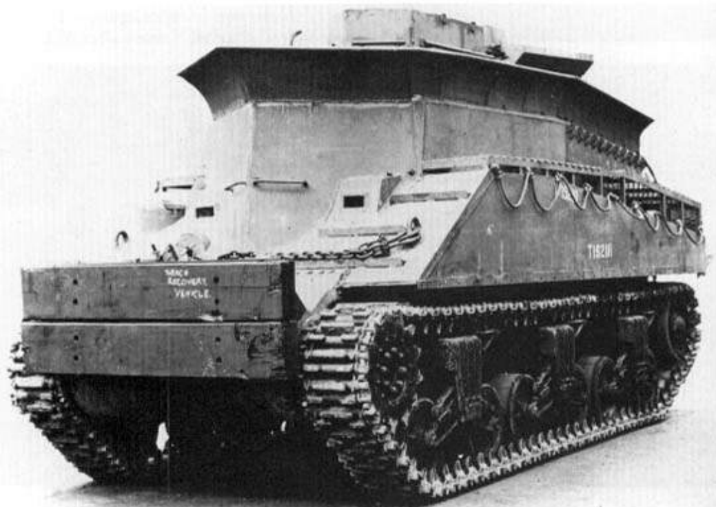
Right: Beach Armoured Recovery Vehicle (BARV). This was a British adaptation of the Sherman ARV Mk I, for use on beach landings. Over 50 were delivered by D-Day and proved to be most useful rescuing swamped vehicles. (TM)
