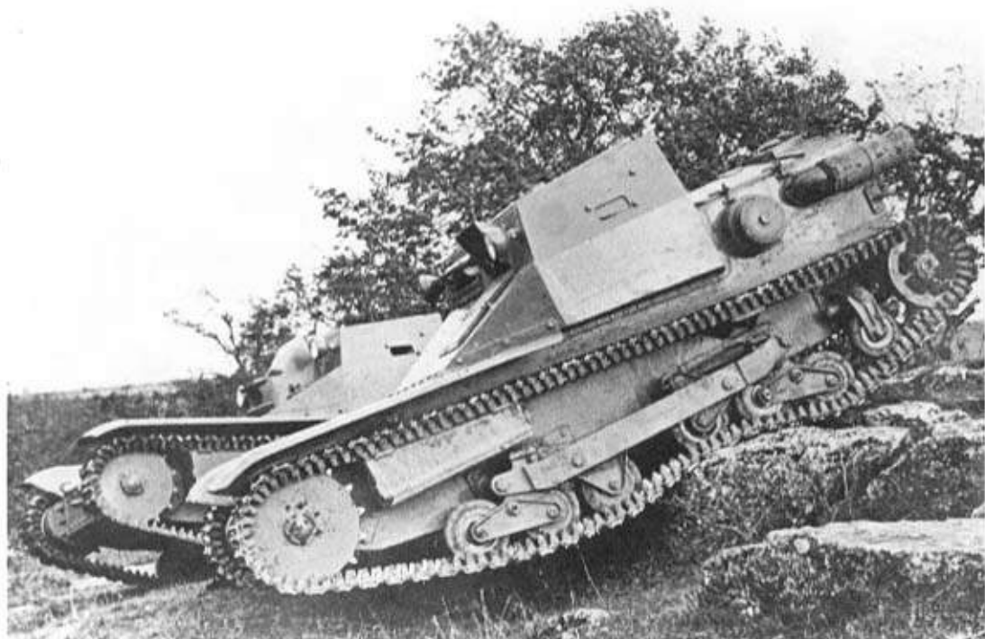
Left: The CV33 (Carro Veloce) was based upon the Vickers Carden-Loyd which the Italians were given a licence to manufacture from 1929 onwards. Various models of this 3.25-ton two-man tankette were produced over the years. (TM)
