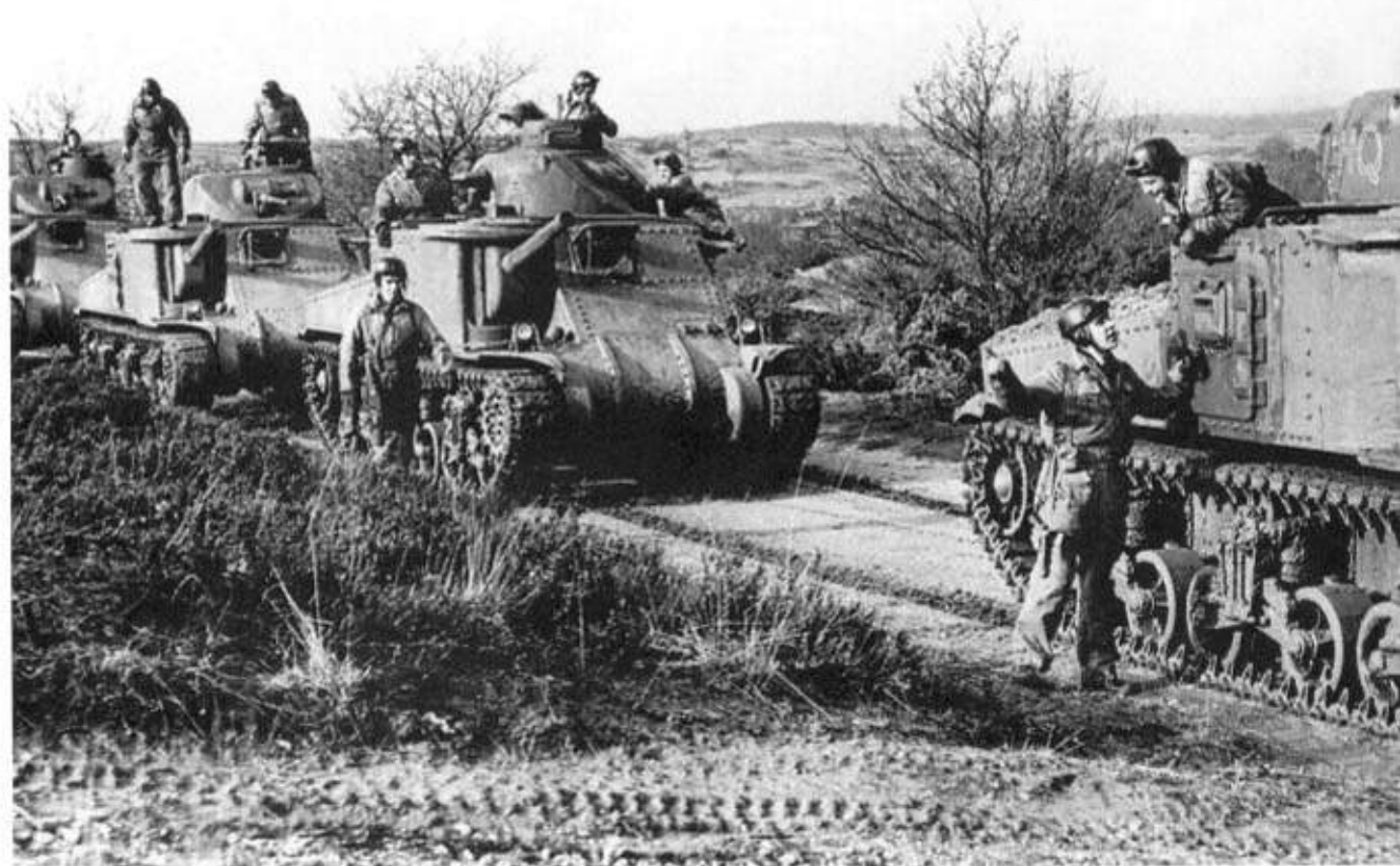
Above: A column of M3 medium tanks on training in Britain. These are the General Lee version, with the commander's cupola, rivetted hull, side doors and powered by a Wright radial engine. They first entered service in April 1941. (TM)
