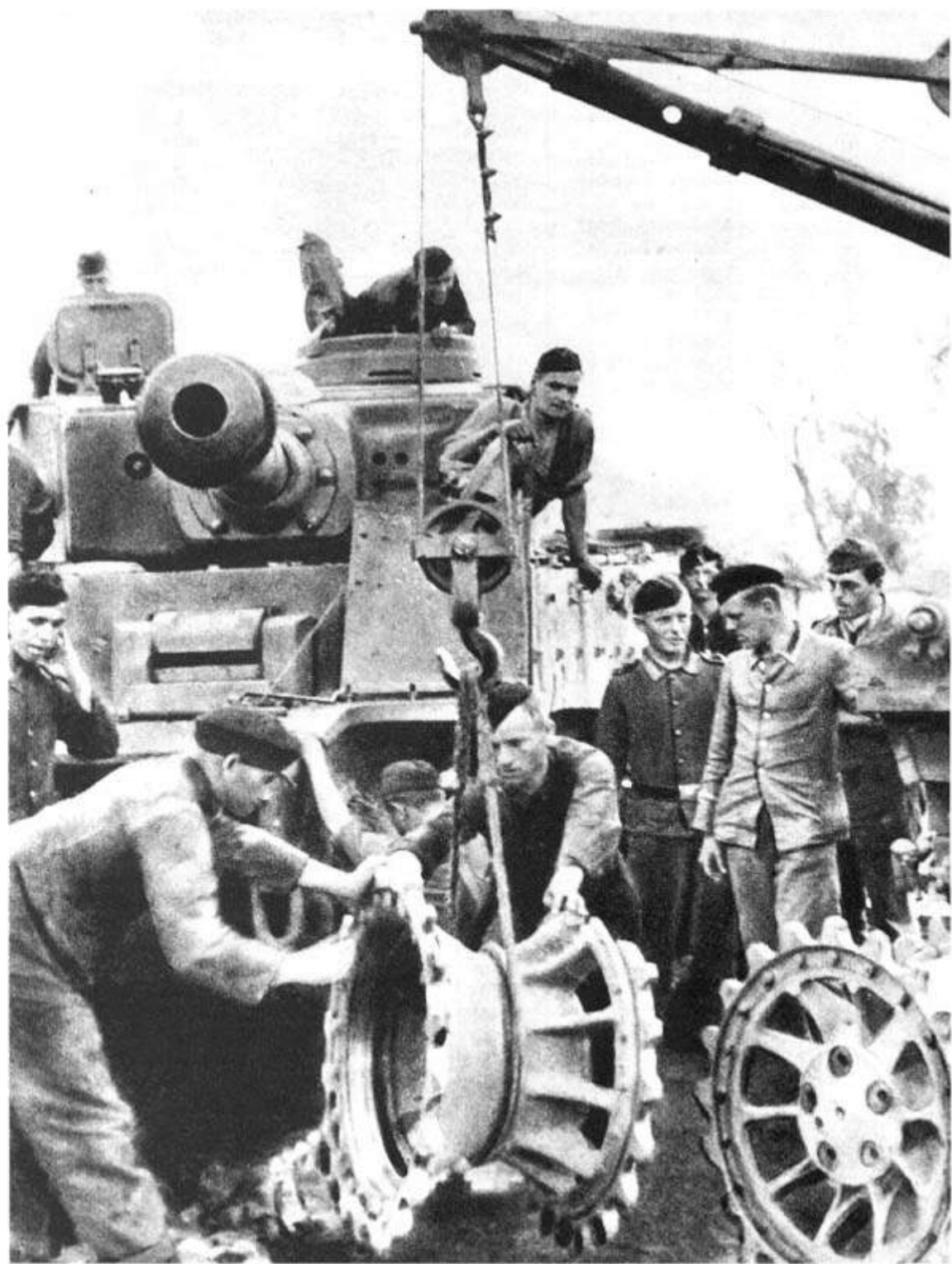
Fitters at work changing a drive-sprocket on a PzKpfw VI Ausf E, Tiger. (GF)
