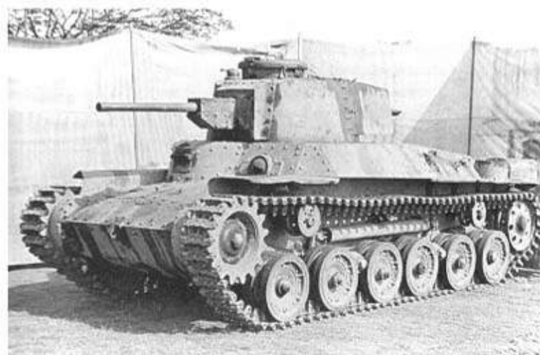
Below: Medium tank Type-97 SHINTO CHI-HA was developed from the original Type-97 CHI-HA. The 15.8 ton four-man tank entered service in 1942. (TM)
