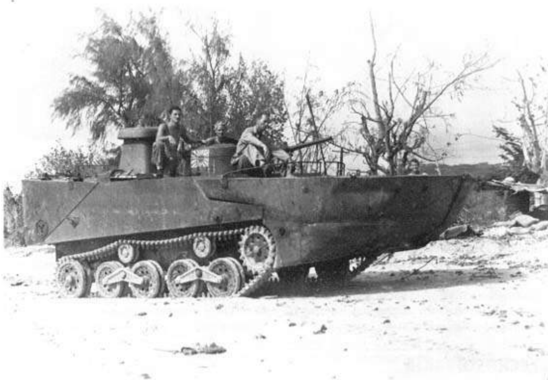
Above and left Amphibious Tank Type-3 KA-CHI, was based on the CHE HE medium tank. It weighed nearly 29 tons, complete with detachable pontoons. This captured Type-3 is crewed by American servicemen. (TM)
