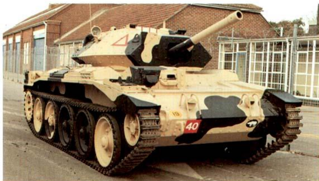
Above: Cruiser Tank Mark V, the Covenanter (A13 Mk III), was a good looking tank with a low silhouette but was a poor performer, being only ever used for training. (TM)
