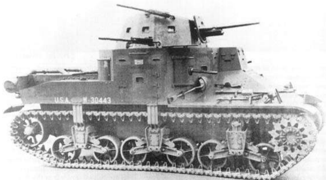
Right: A T5 phase III medium tank, photographed at Rock Island Arsenal, 1938. This was the prototype of the standard production M2 medium tank, forerunner of M3 and M4. (TM)
