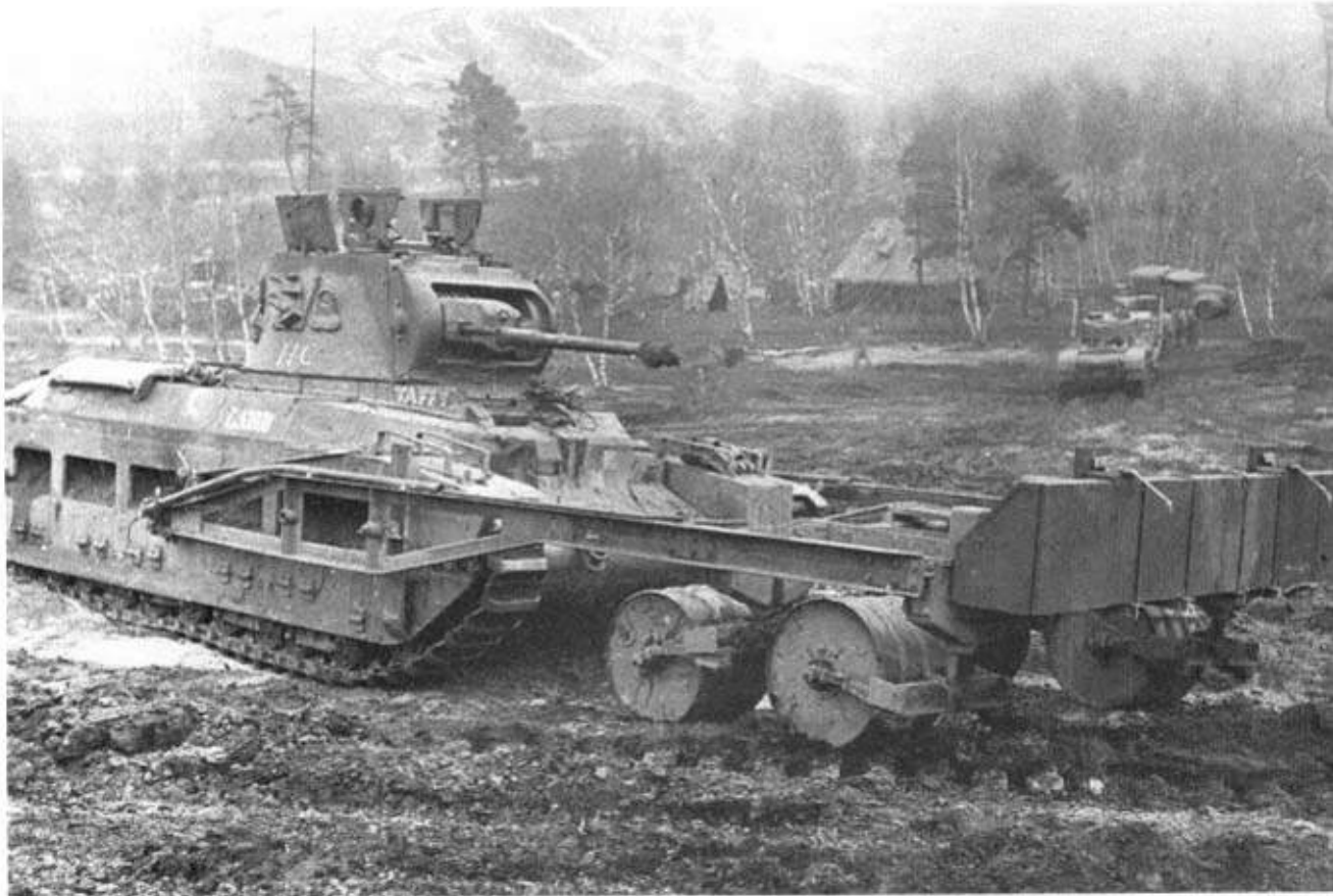
Above: Matilda II, pushing Heavy Carrot mine clearing device – a 600lb demolition charge carried in front of AMRA and detonated remotely from the tank. Photographed at the Obstacle Assault Centre. (TMO)
