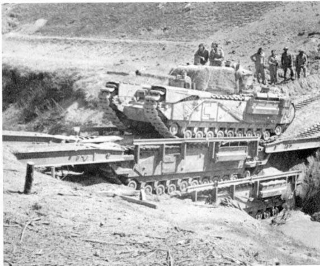
Left: Two Churchill Mk I ARKs in a deep gully, one on top of the other, so as to bridge the gap. ARK could also be used to assist tanks to surmount other obstacles, like seawalls - a lesson learnt at Dieppe, France 19 July 1942. (TM)
