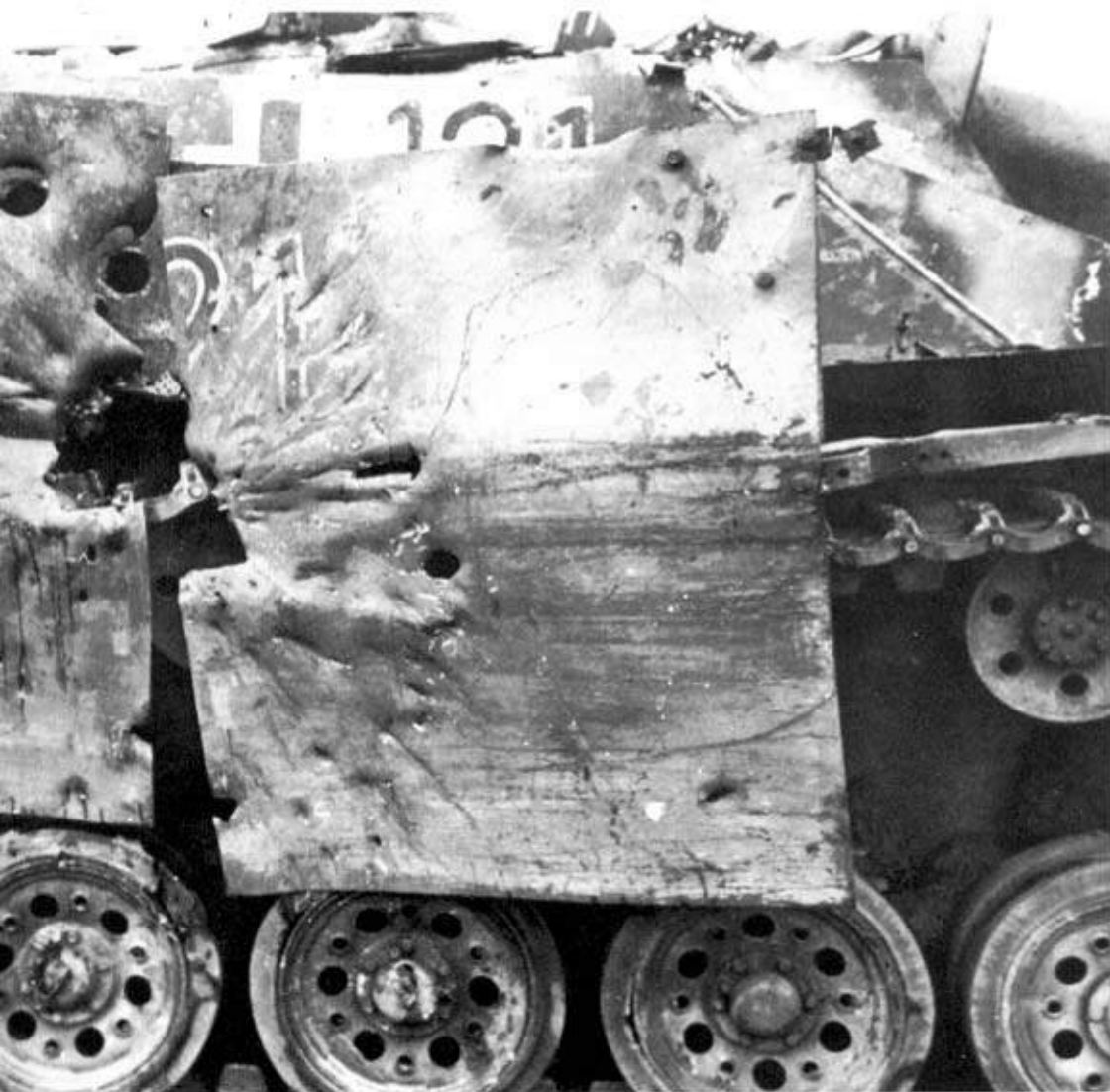
Left: A graphic impression of a strike on the bazoooka protection plates of this StuG 40. (TM)
