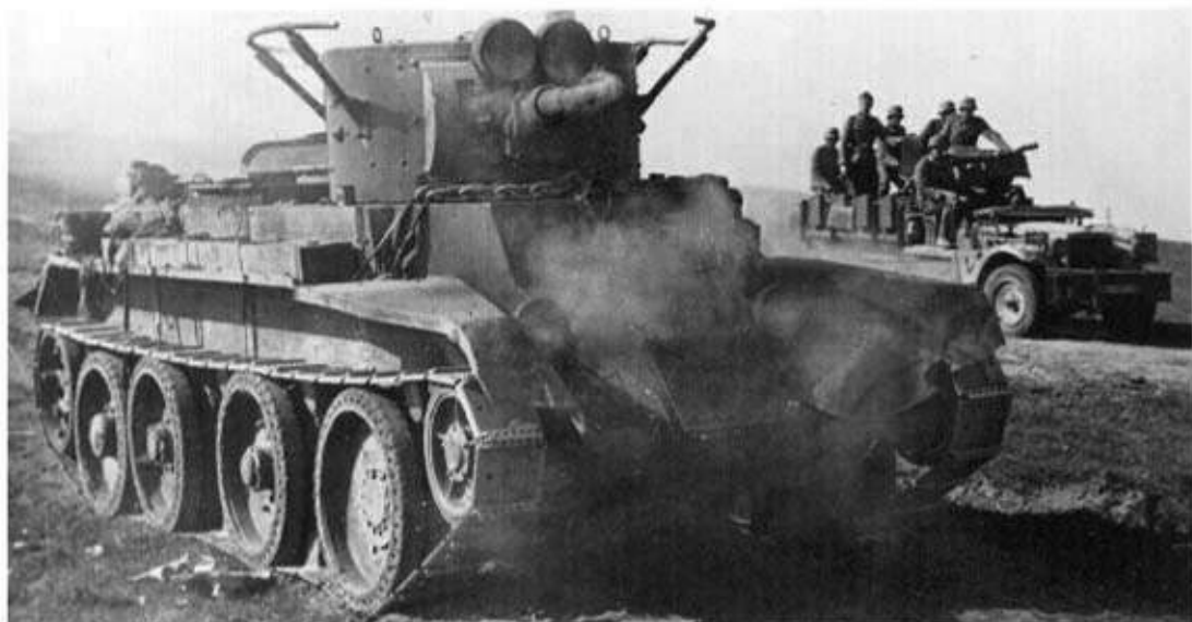
Right: The Commander's version of the BT-7-V was fitted with a very conspicuous frame aerial around the top of the BT-5(V) turret. In the background are German troops on board a Einheits Lkw 6x6 truck. (T.M.)
