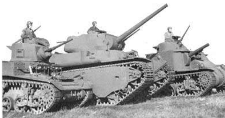
Above This interesting line-up compares an M6 heavy tank with the M3 light tank and M3 medium tank. Despite its size and gun power the M6 did not impress the Armored Force. (TM)
