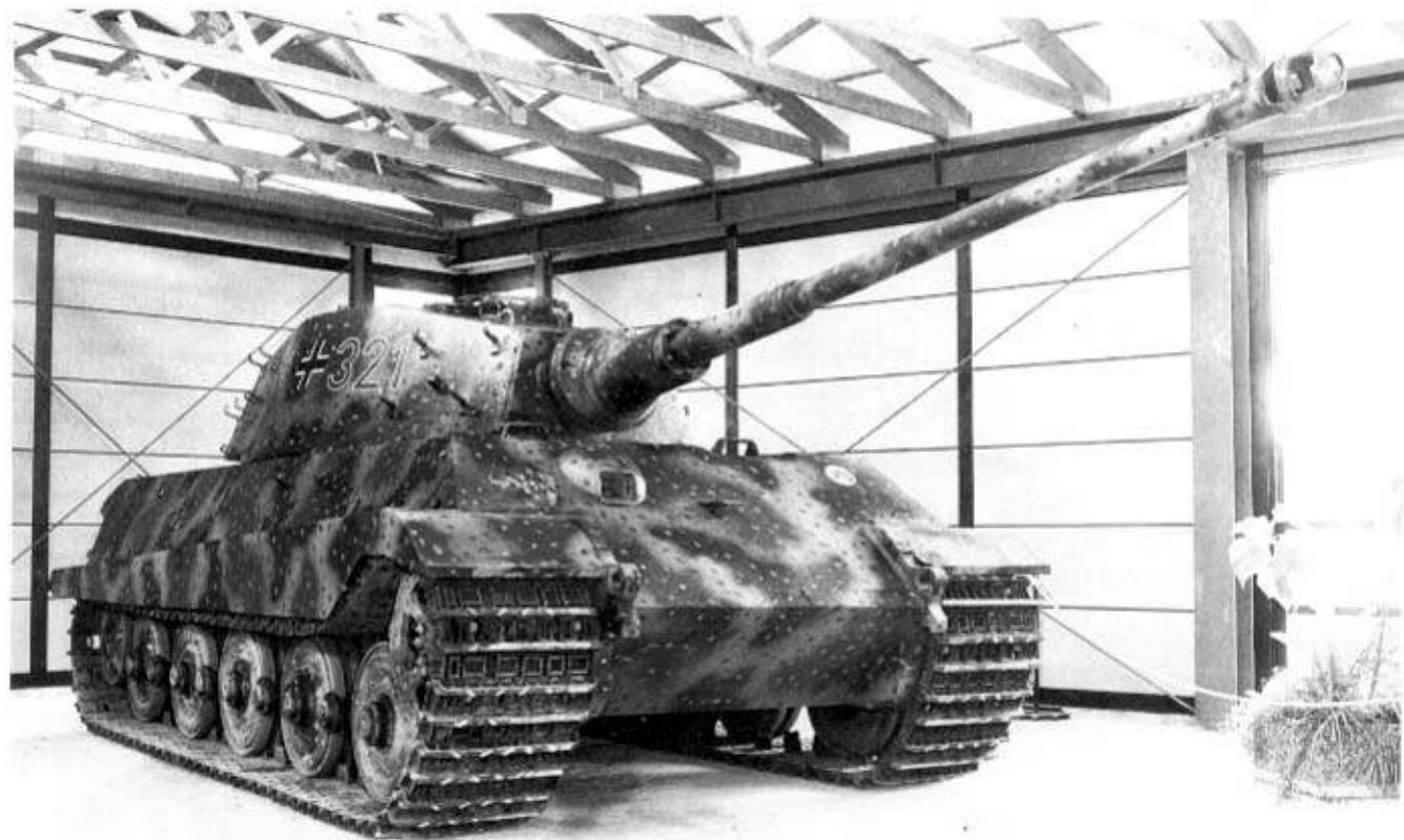
Above: Another immaculate tank from the Panzermuseum in Germany. This is the Tiger II, the production model with the Henschel turret.
