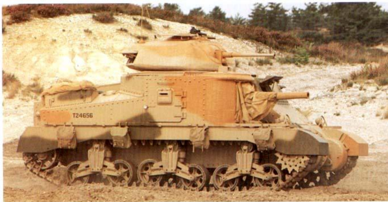
Above: M3 General Grant in desert camouflage. Note the canvas dust cover over the sponson-mounted gun's mantlet. (TM)
