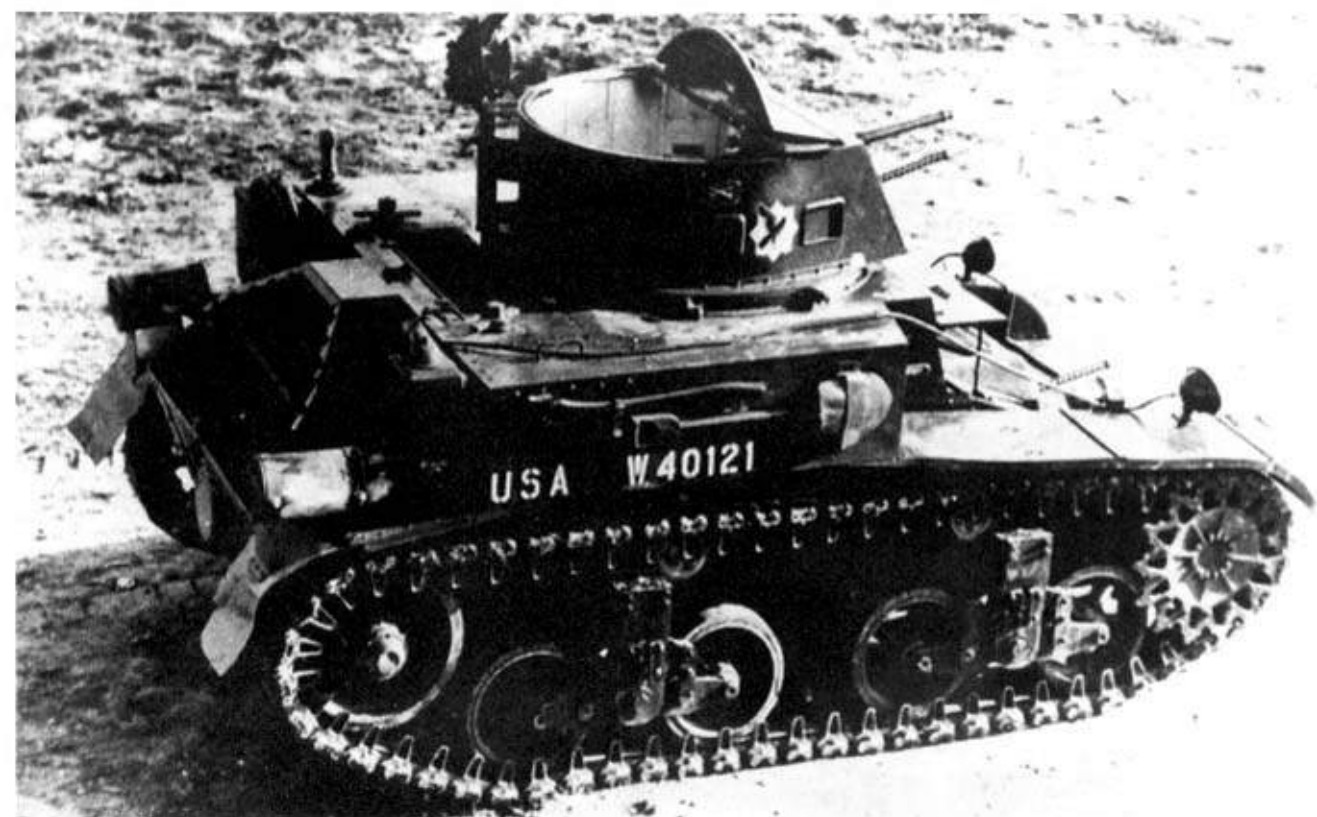
Above: The Cavalry Combat Car M1, shown had one turret instead of two as on the light tank. This example is from the 1st Cavalry Regiment of the 7th Cavalry Brigade, 1939. (TM)
