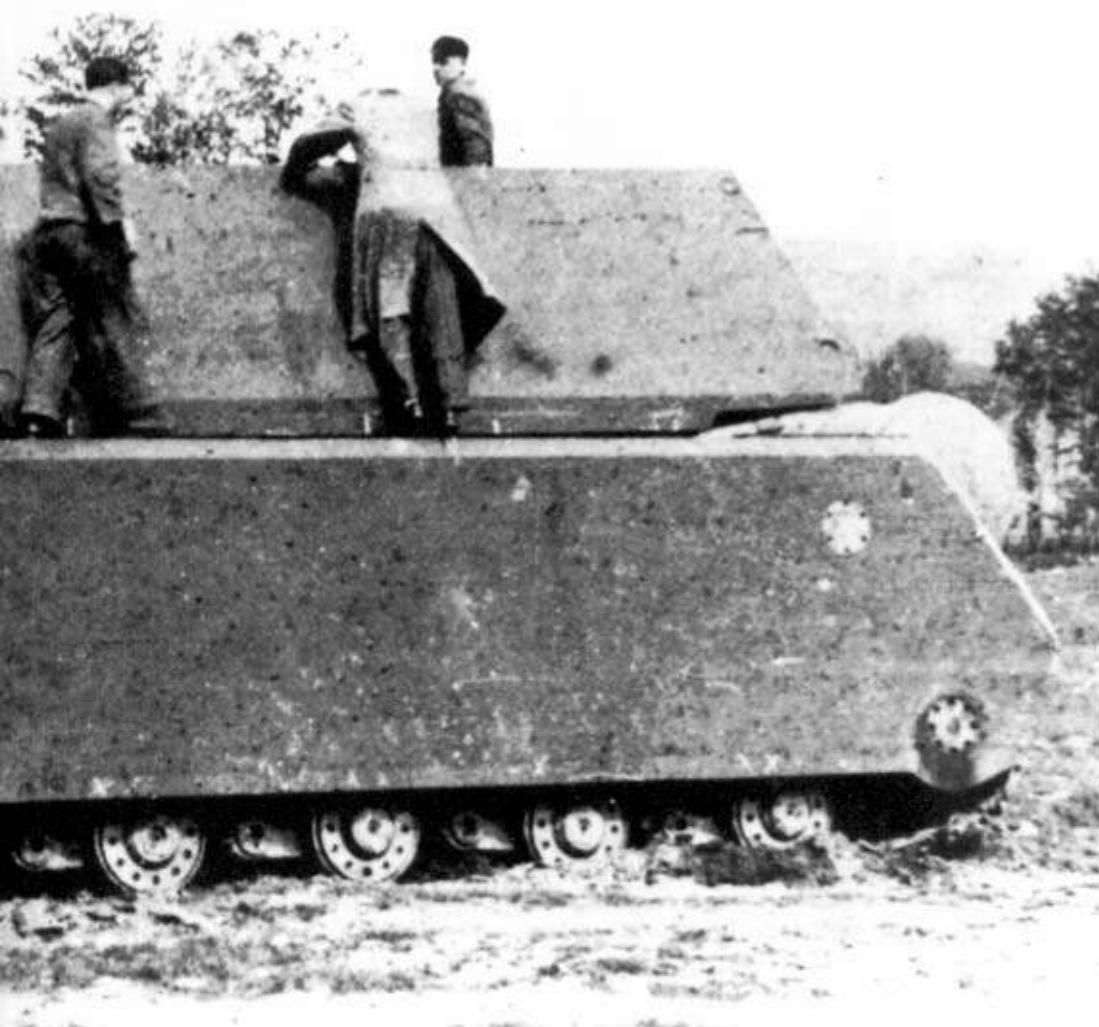
Left: Maus, the 188ton 'super-heavy tank' never saw operational service. Two prototypes were built and nine more were in production when the war ended. The only remaining Maus is in the Russian Tank Museum at Kubinka, near Moscow. (TM)
