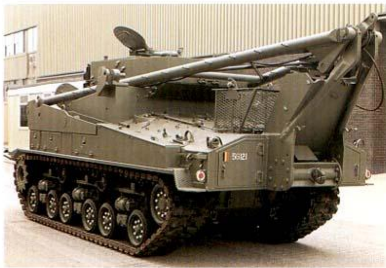
Above: Sherman M32 Tank Recovery Vehicle, was equipped with a jib and a powerful 60,000lb winch. It also mounted an 81mm mortar, so that a smoke screen could be created as cover for operations (not fitted on this vehicle). (TM)
