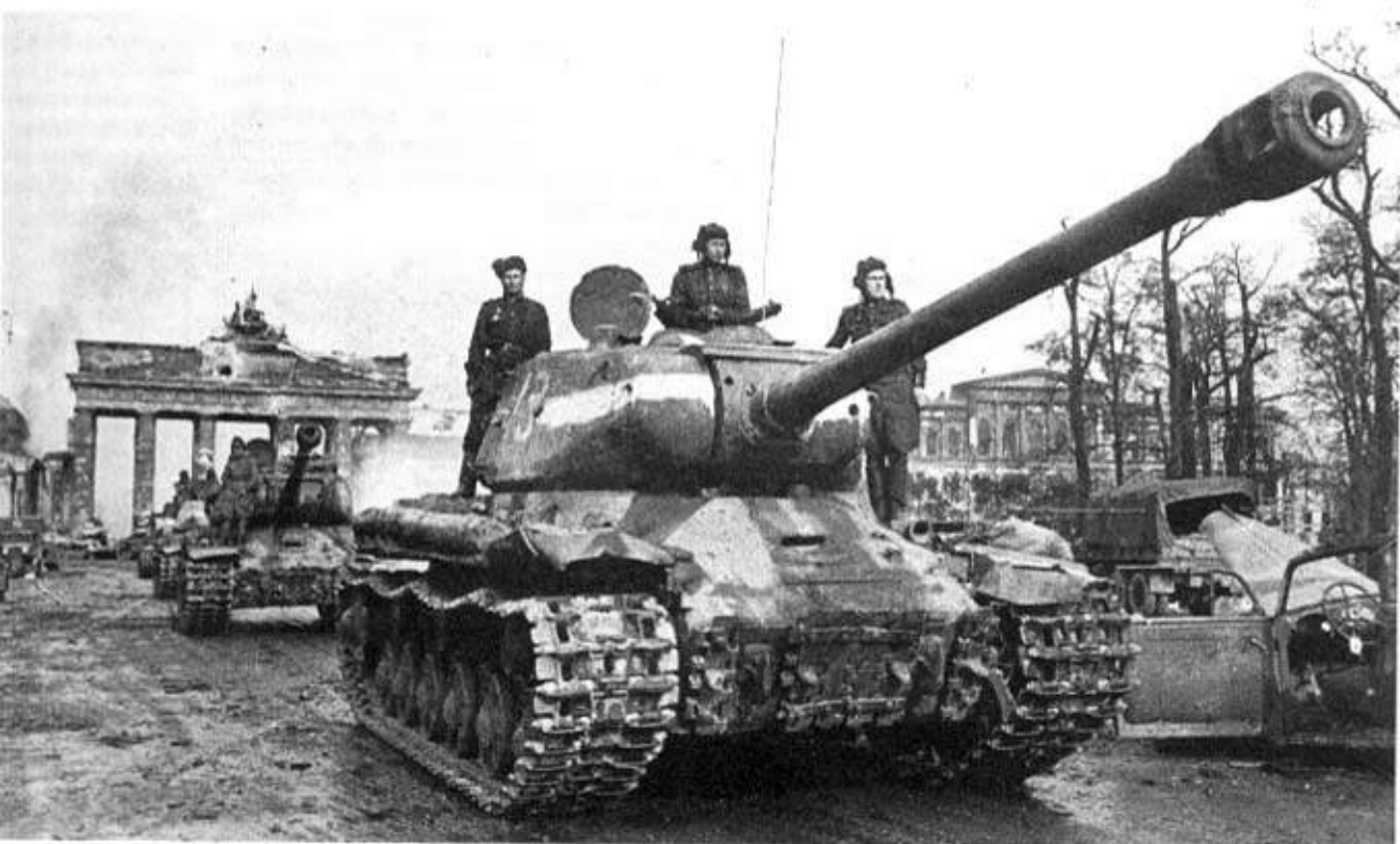
Below IS-2, the improved version of the IS-1, was the major production model, 2,250 being built. Photographed near the Brandenburg Gate, Berlin, 1945. (GF)
