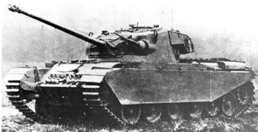
Right: The A41 Centurion Mk I was the first of a highly successful line of medium gun tanks which continued for over 25 years. Armament is a 17 pounder gun and a 20mm Polsten cannon (only fitted to pilot models, later a co-ax BESA MG was fitted). (TM)
