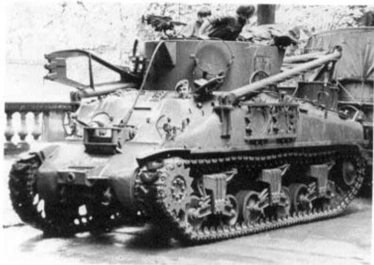
Above: A well restored example of a late production M32B1, Sherman Tank Recovery Vehicle. (TM)
