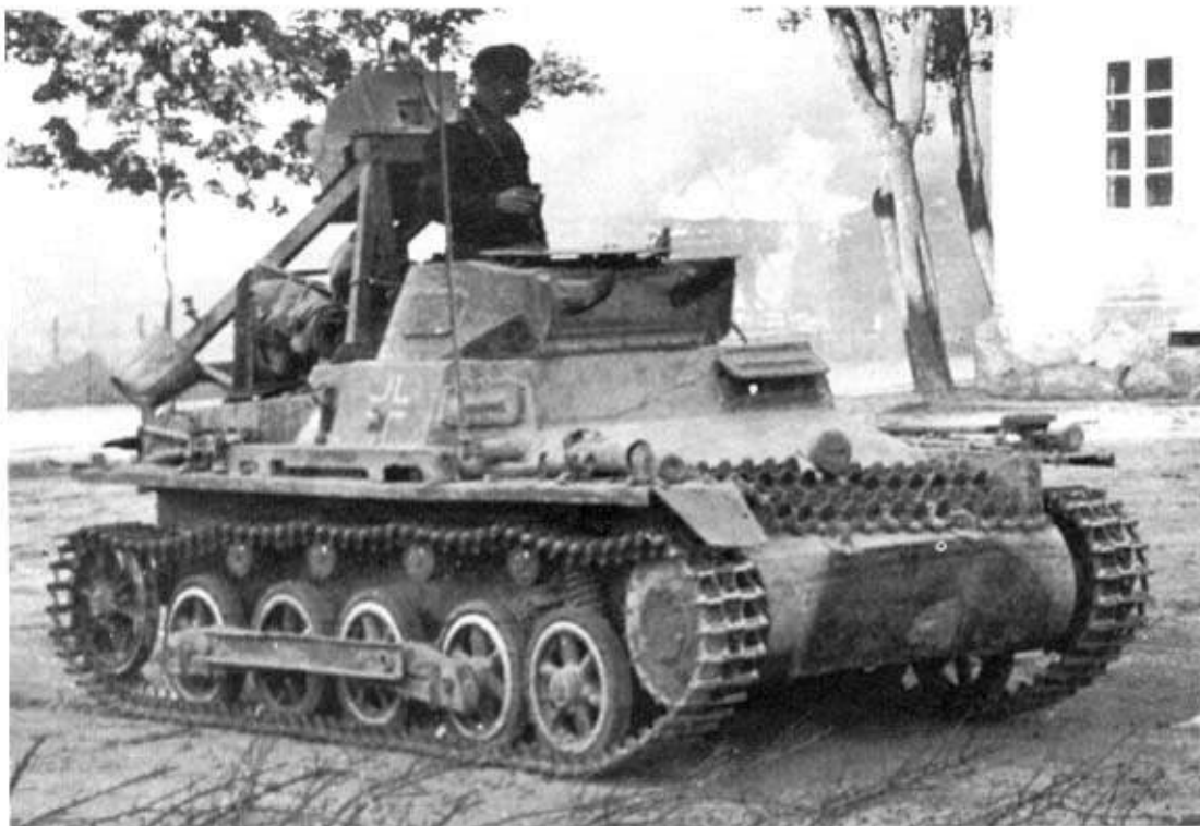
Left: Ladungsleger auf PzKpfw I Ausf B , demolition laying version of the PzKpfw I. The demolition charge was released down a chute at the rear of the tank. (TM)
