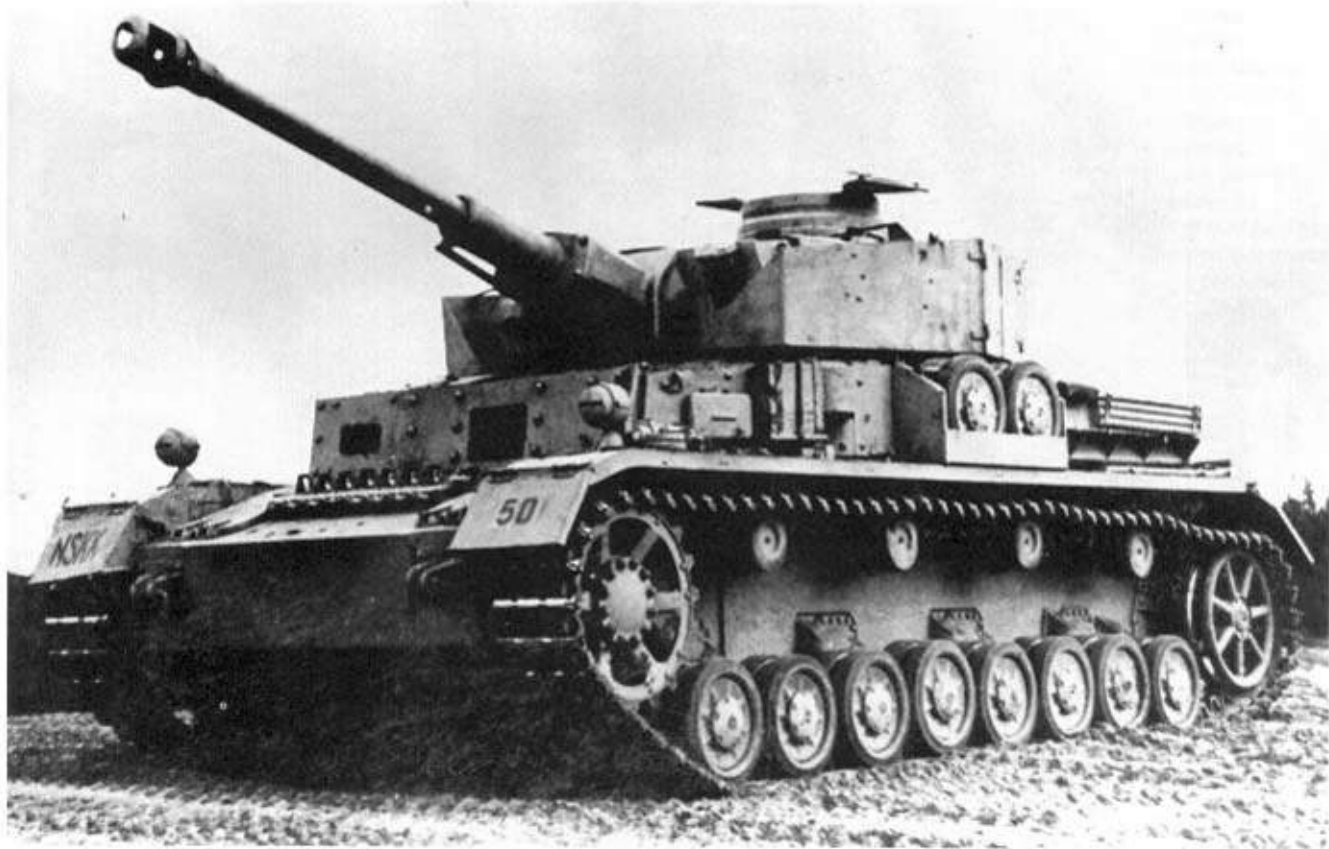
Above: This up-gunned PzKpffw IV Ausf D is fitted with a 75mm KwK L/48 gun and also additional spaced armour around the sides of the turret. (TM)
