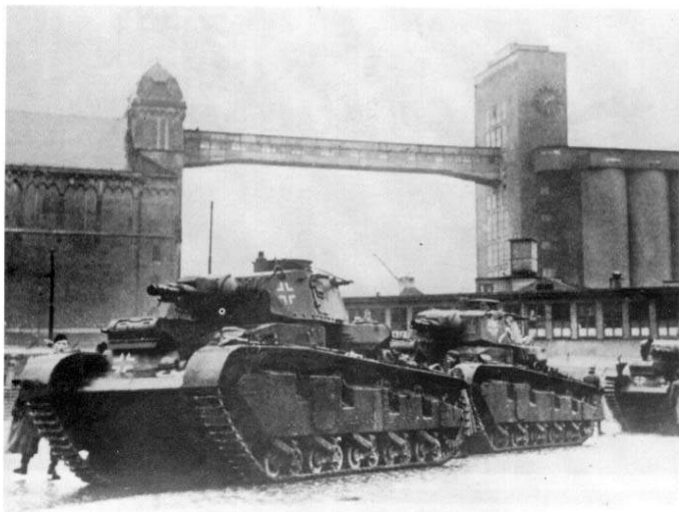
Above: The Neubaufahrzeug medium tank (sometimes known as PzKpfw VI) was ordered from Rheinmetall in 1933 and was to be the first German multi-turretted medium tank. Two prototypes and three experimental vehicles were produced. The latter were sent to Norway in April 1940, where they were used in action, one being destroyed. Photographed in Oslo, 1940. (TM)
