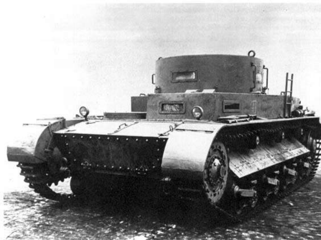
Far left below: This modified version of the VK2001 (Rh) , built by Rheinmetall Borsig AG in 1935, was a direct successor to the Bataillonführerswagen . Also it was the predecessor to the PzKpfw IV series, which became the backbone of the Panzerwaffe, remaining in production from 1935 until March 1945. (TM)
