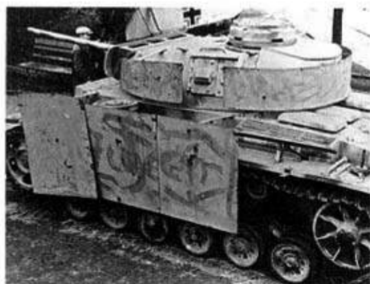
Left: Additional spaced armour fitted to the turret and sides of a PzKpfw III. This was designed as extra protection against attack by HEAT weapons such as the American Bazooka and the British PIAT. (TM)
