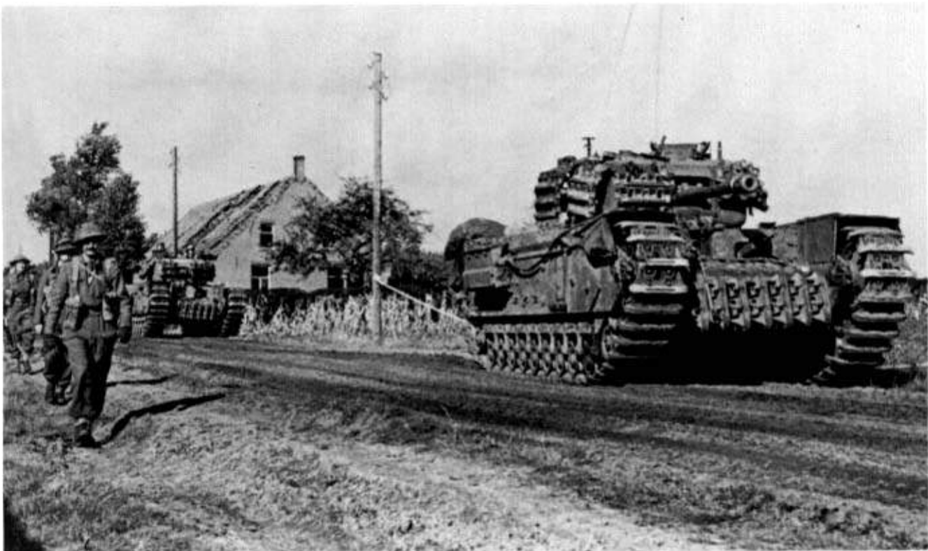
Above: Churchill Mk VIs of 4th Battalion Grenadier Guards and accompanying infantry of 1st Battalion Suffolks advance through a Dutch village, 1944. Note the extra armoured protection by adding trackplates to the front glacis and turret. (TM)
