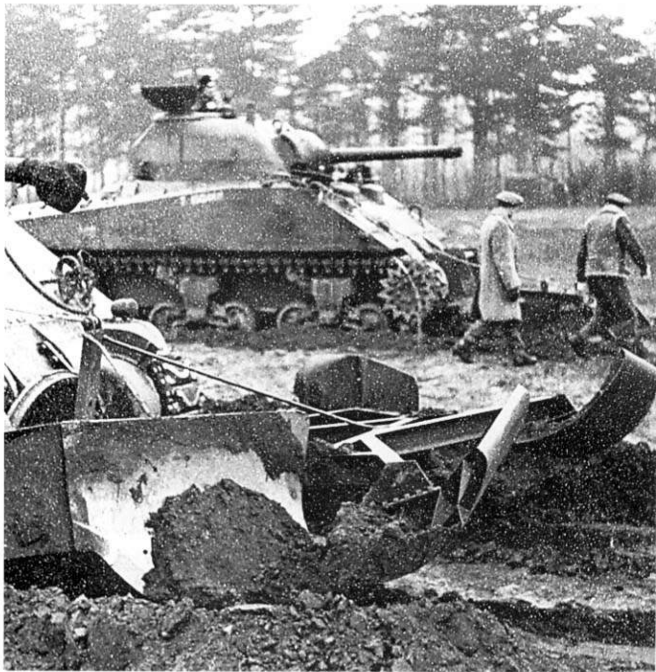
Above: The British-invented Bullshorn Plough had one ploughshare fitted ahead of each track. They were used by the 79th Armoured Division on the Normandy beaches, 1944. The photograph is of the equipment on trials in a snow storm. (TMA)
