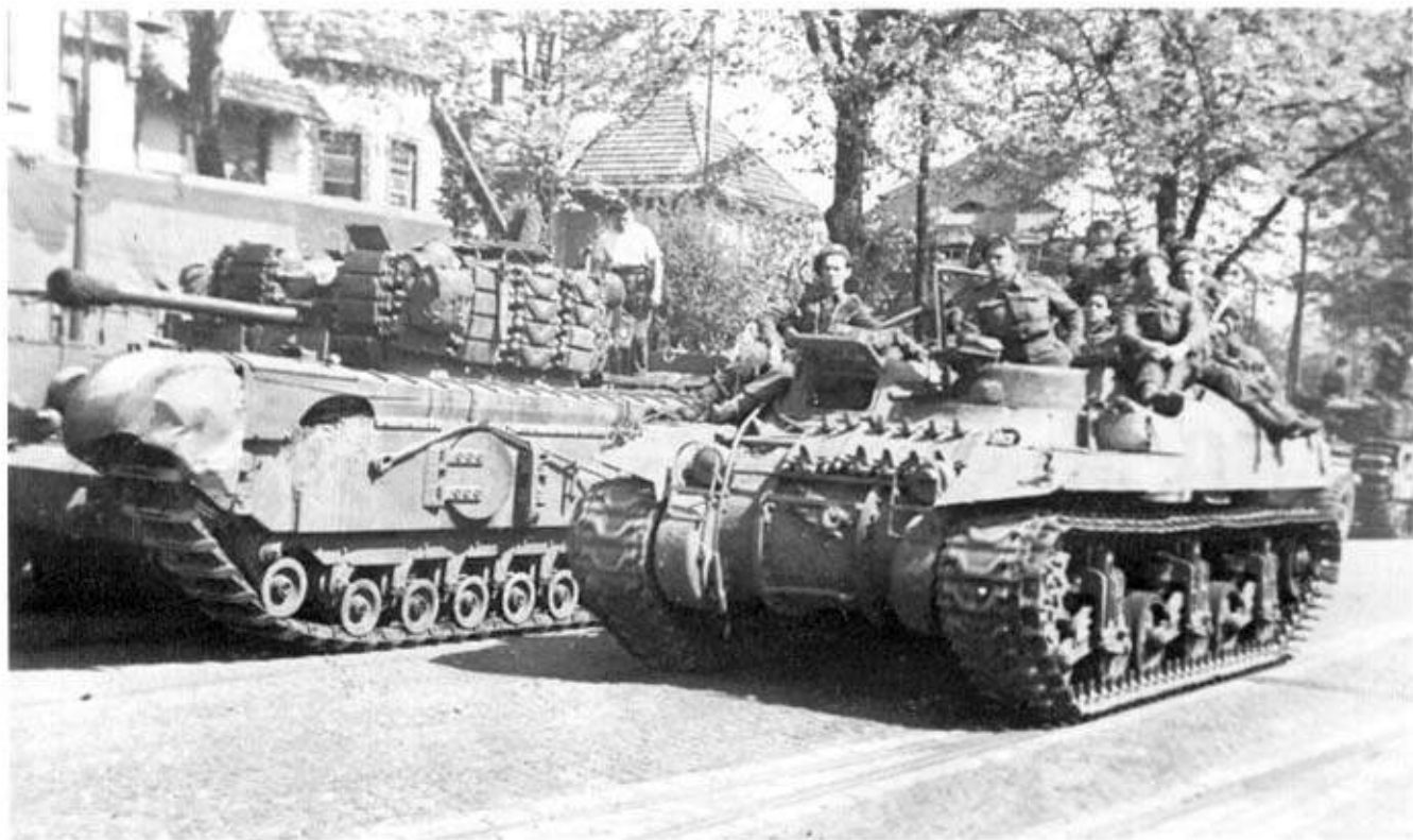
Above: A heavily laden Ram Kangaroo APC passing a well-protected Churchill. The Kangaroo was a stripped out Ram and could carry a full infantry section of eleven men and their equipment. (TM)
