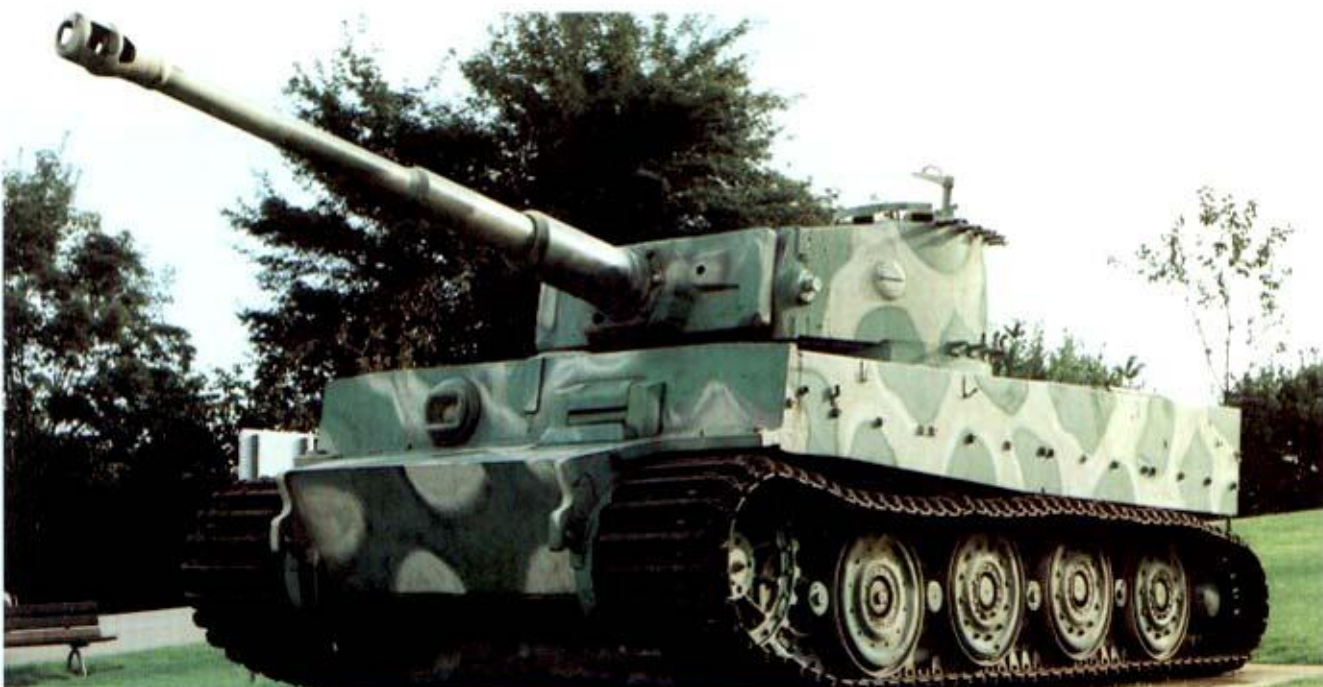
Below: The awe-inspiring front view of a Tiger I, its 88mm gun capable of defeating 90mm of armour plate at 2,300 metres. Tiger carried 92 rounds of mixed ammunition (AP & HE) for its main gun. (TM)
