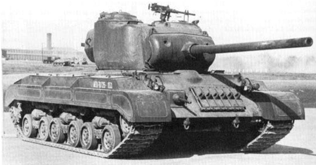
Right The T25 pilot Number 1 was tested at APG in late January 1944. It had HVSS suspension and a 90mm gun mounted in a large turret. It was dropped in favour of the T26. (TM)
