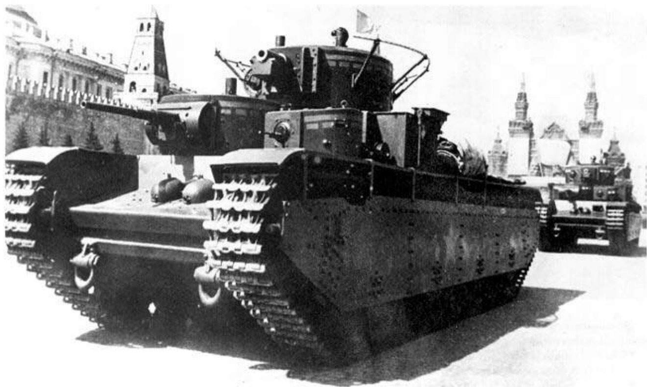
Above: The T-35 heavy tank weighed 45 tons, the main turret mounting a 76.2mm howitzer, while two of the four sub-turrets had 37mm guns and two machine guns. Shown is the commander's version in a parade on Red Square, Moscow. (MM)
