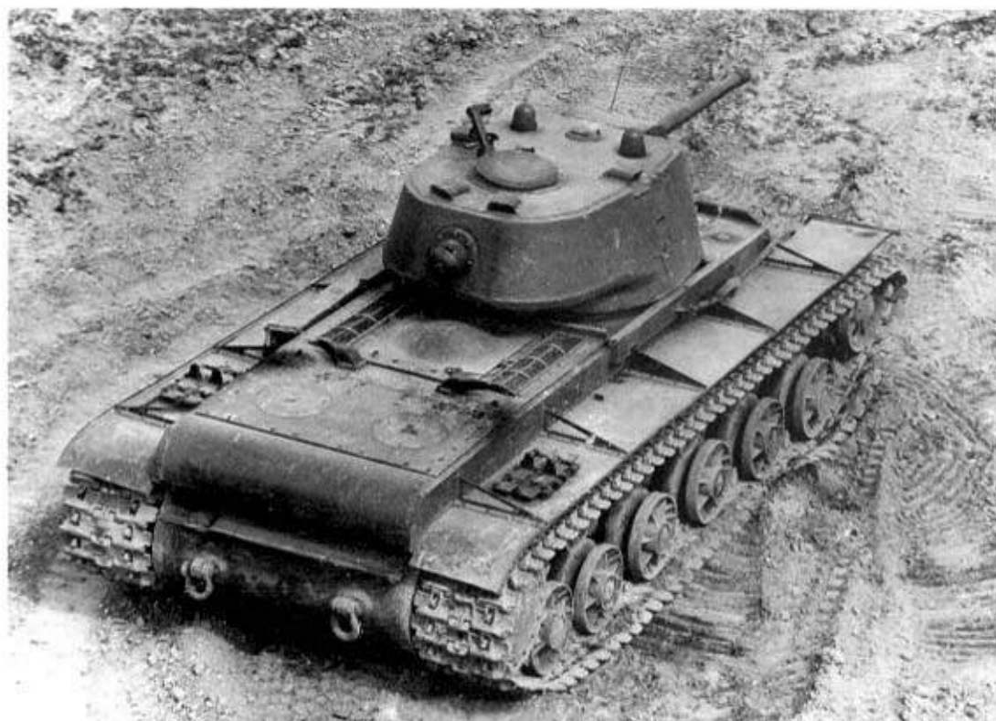
Left. The KV-1 was based closely on the T-100/SMK heavy tanks, but with only one turret, mounting a 76.2mm L/40 gun. There were a number of versions, weighing from 46 to 47 tons, depending upon armour thickness. This is a KV-1B, which had extra armour on the front and sides.
