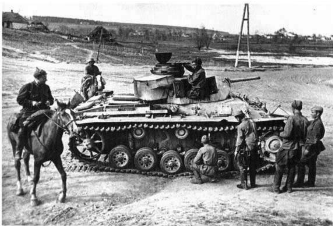
Left: Soviet troops inspecting an abandoned PzKpfw III Ausf J, in June 1942. The Ausf J still mounted the 50mm gun, but had thicker armour front and rear than previous models. (TM)
