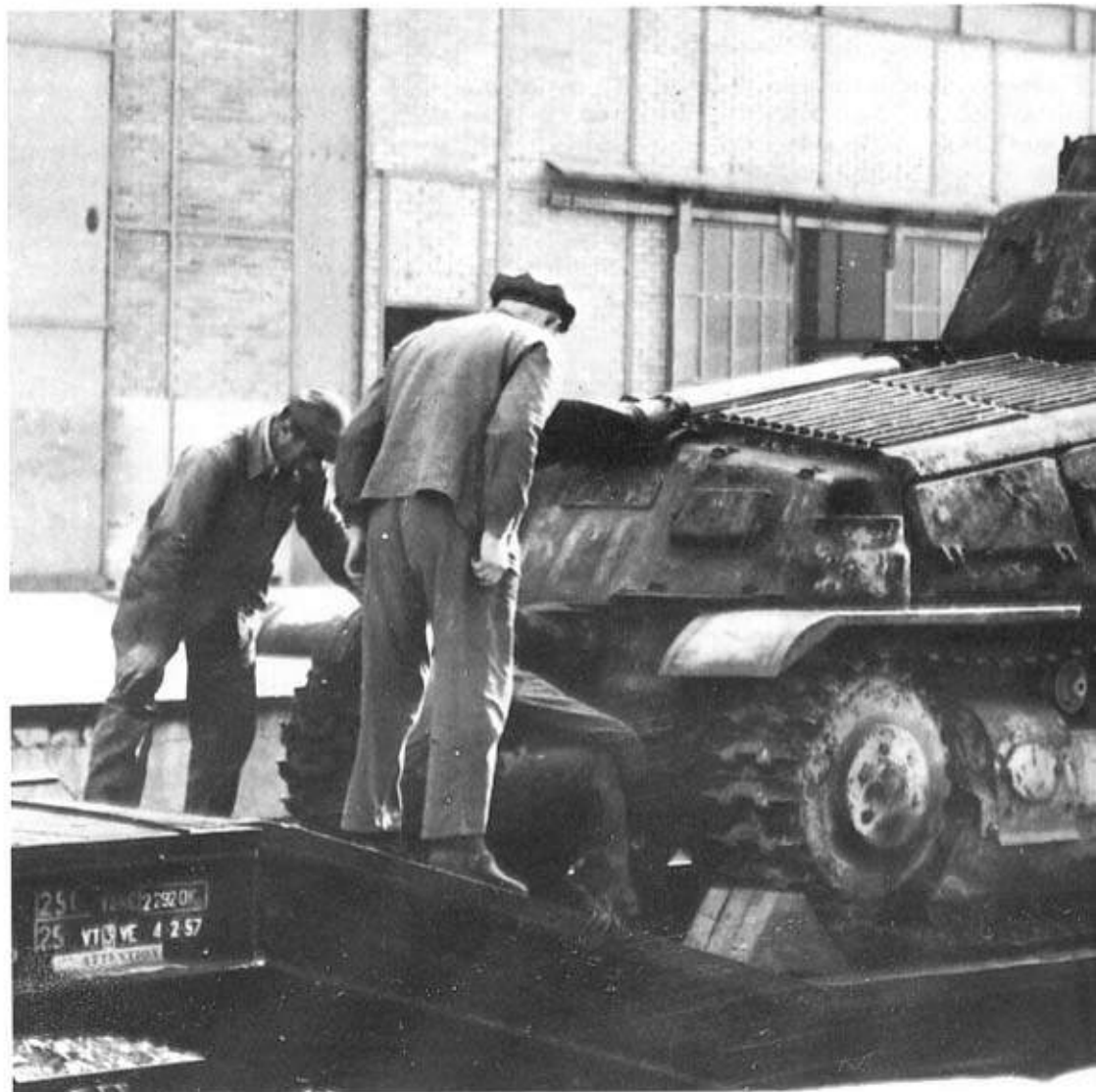
Right: A Char S 35 Somua medium tank being chained down on a railway flatcar by French workmen. The Somua was one of the best French tanks, being better than most of its German contemporaries. Captured S 35s were used by both German and Italian forces. (TM)
