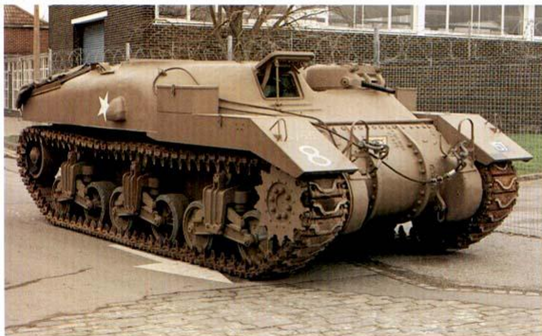
Above: Sherman M32 Tank Recovery Vehicle, was equipped with a jib and a powerful 60,000lb winch. It also mounted an 81mm mortar, so that a smoke screen could be created as cover for operations (not fitted on this vehicle). (TM)
