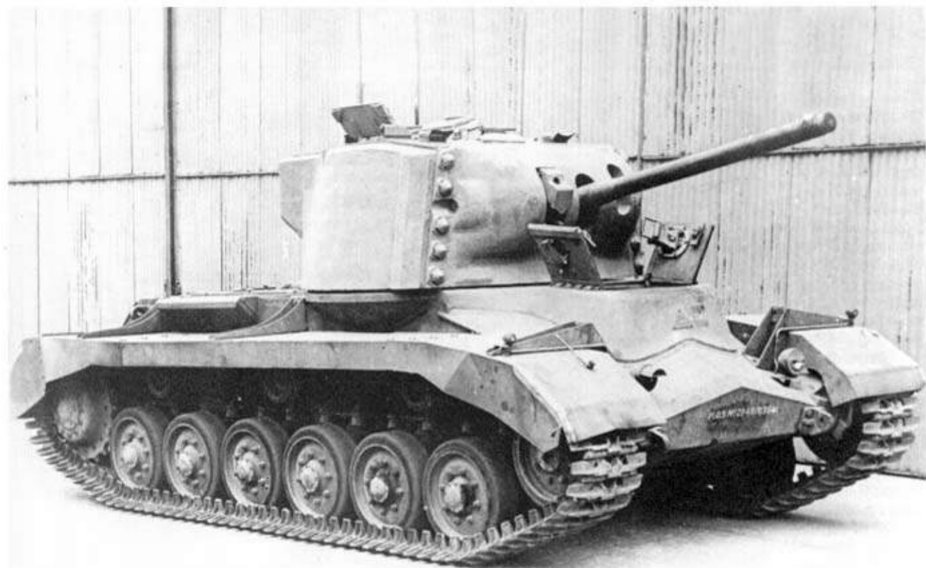
Above: The 27ton A38 Valiant was designed as an improved version of Valentine, but was 10 tons heavier. Underpowered it never entered production, being cancelled in 1945. The surviving A38 is in the Tank Museum, Bovington. (TM)
