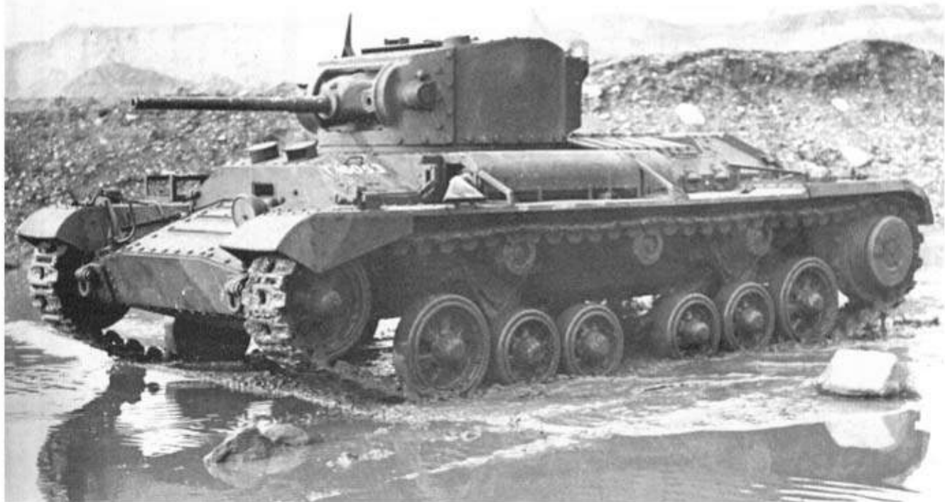
Above: Valentine Mk I was the first model of the Infantry Tank Mk III and mounted a 2 pounder gun and co-ax BESA MG. Photographed on trials in Britain, 1939. (TAM)
