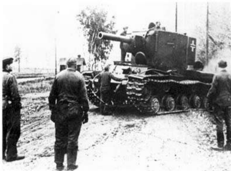
Below. The KV-2A was the close support version mounting a 152mm howitzer in a large, slab-sided turret. It weighed 53 tons. (TMA)
