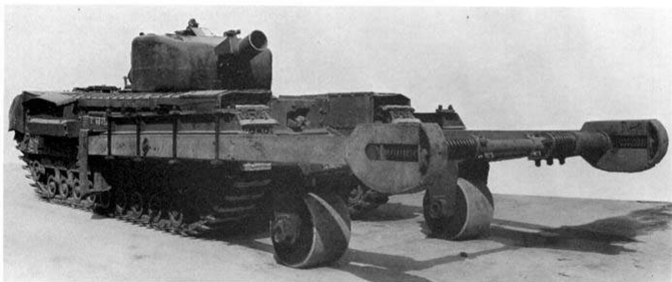
Below: Churchill AVRE fitted with CIRD (Canadian Indestructible Roller Device). (TM)
