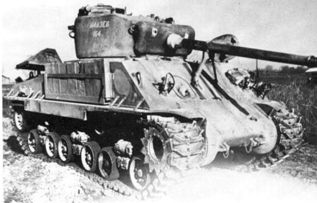
Right: This M4A3E8 was one of a number of models used to test out the new Horizontal Volute Spring Suspension system (HVSS), which was a significant improvement over the old vertical volute spring (VVS) type. (TM)
