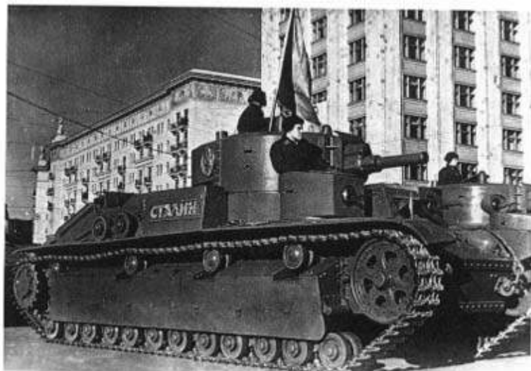
Above: The T-28 medium tank was designed as the Red Army's answer to the German Nbz, British A1E1 and French Char de Rupture . The 1938 version shown mounted the new 76.2mm L/10 gun. (TM)
