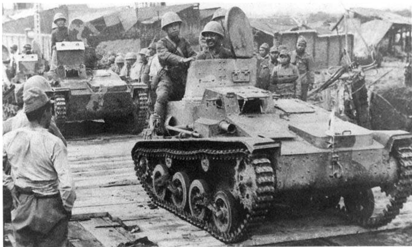
Above: The 3.5 ton Type-94 TK tankette was developed from the Vickers Carden-Loyd Mk VI, but with a small turret mounting a single 7.7mm machine gun. (TM)
