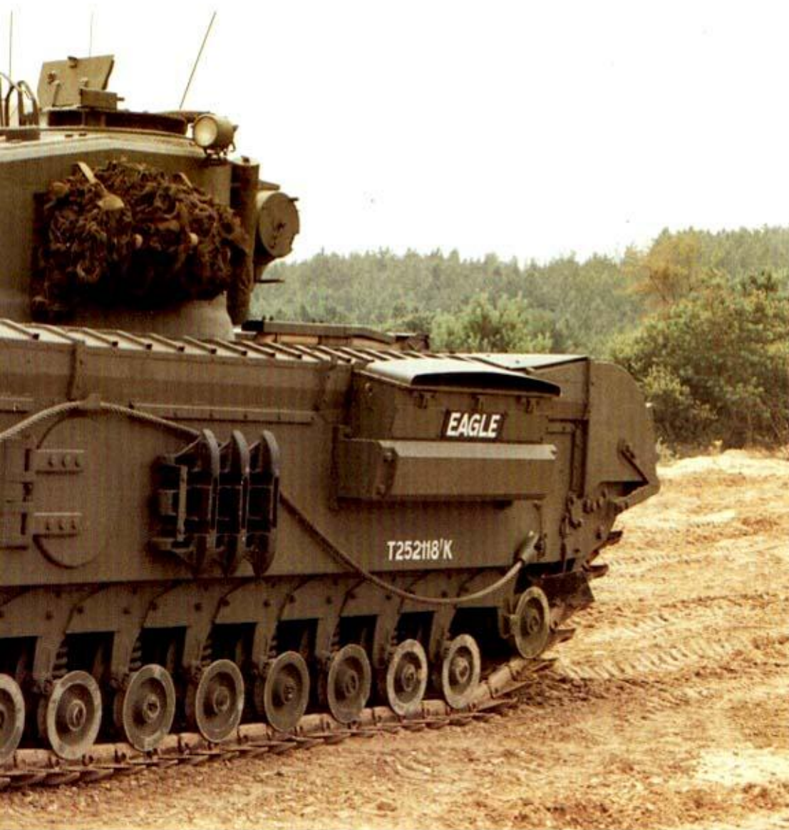
Left: The Infantry Tank Mk IV was named the Churchill after the great wartime Prime Minister Winston Churchill. There were eleven Marks of Churchill, the Mk I mounted a 2 pounder gun in the turret and 3 inch howitzer in the hull. From Mk III onwards it was armed with a 6 pounder and from Mk VIII with a 75 mm gun. (TM)
