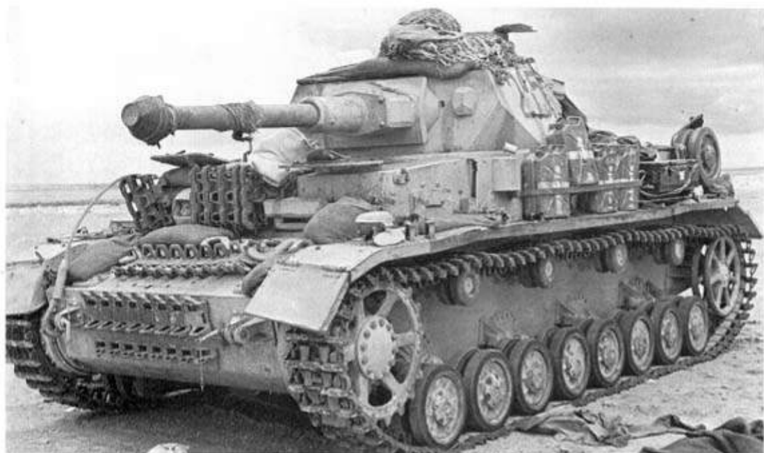
Above: This up-gunned PzKpffw IV Ausf D is fitted with a 75mm KwK L/48 gun and also additional spaced armour around the sides of the turret. (TM)
