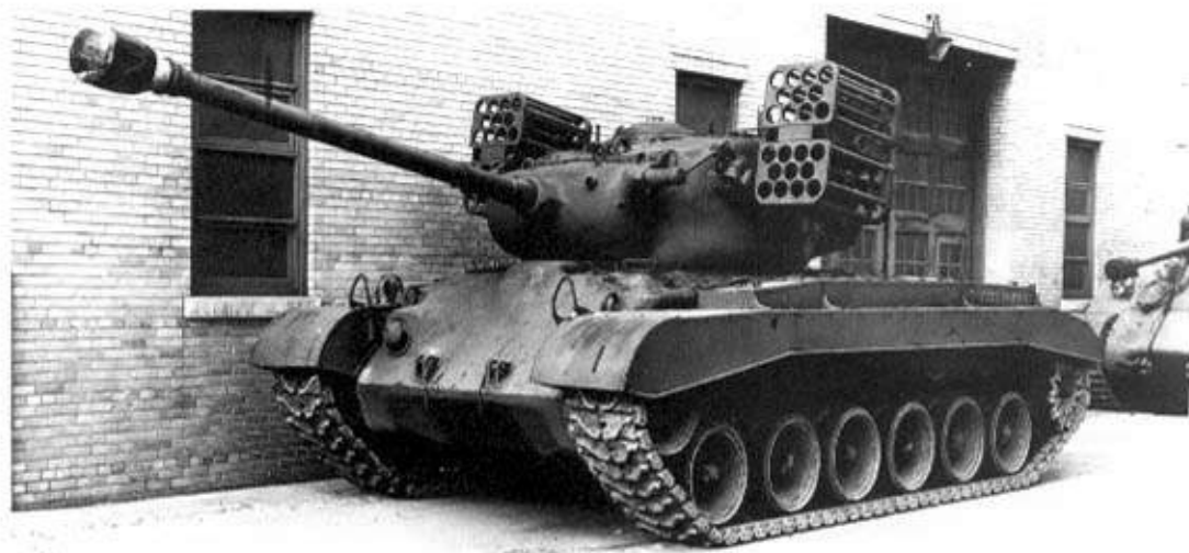
Left: Pershing with the T99 multiple rocket launcher. This was tested in 1945 and could fire forty-four 4.5in rockets from the jettisonable launcher frame. (TM)
