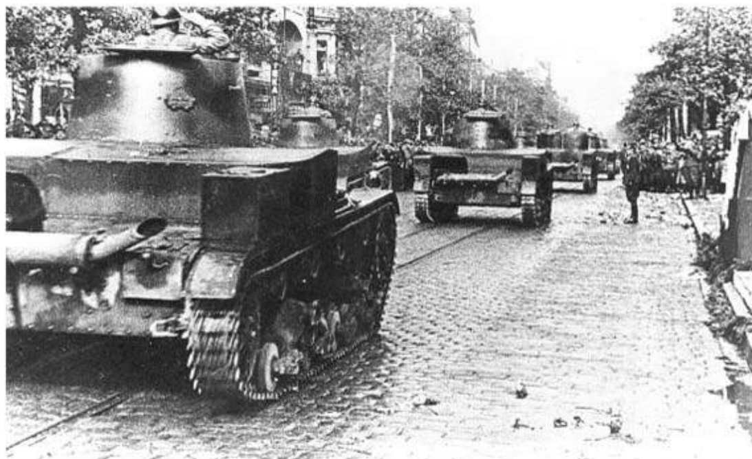
Left: Polish 7-TP light tanks were developed from the British Vickers 6 ton Mk E. Those leading the parade are the twin turret model, while the tank nearest the camera has a single turret. (TM)
