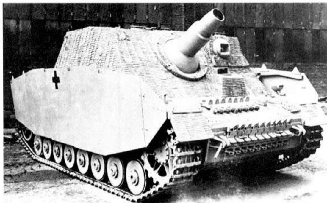
Left: Sturmpfanz IV Brummbär (Grizzly Bear), 150mm assault howitzer on a PzKpfw IV chassis. Just under 300 were produced and rushed to the Eastern front to take part in the Kursk offensive in 1943. (TM)
