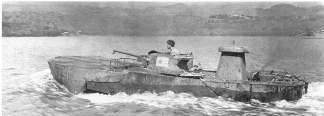
Above and left Amphibious Tank Type-3 KA-CHI, was based on the CHE HE medium tank. It weighed nearly 29 tons, complete with detachable pontoons. This captured Type-3 is crewed by American servicemen. (TM)
