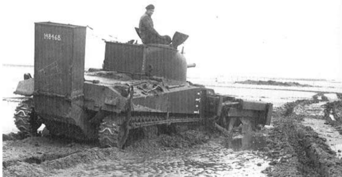
Right: A Sherman Crab MK II of 30 Armoured Brigade, 79th Armoured Division, on a Normandy beach. Of the 30 deployed twelve were destroyed. Note the engine wading breather at the rear. (GF)
