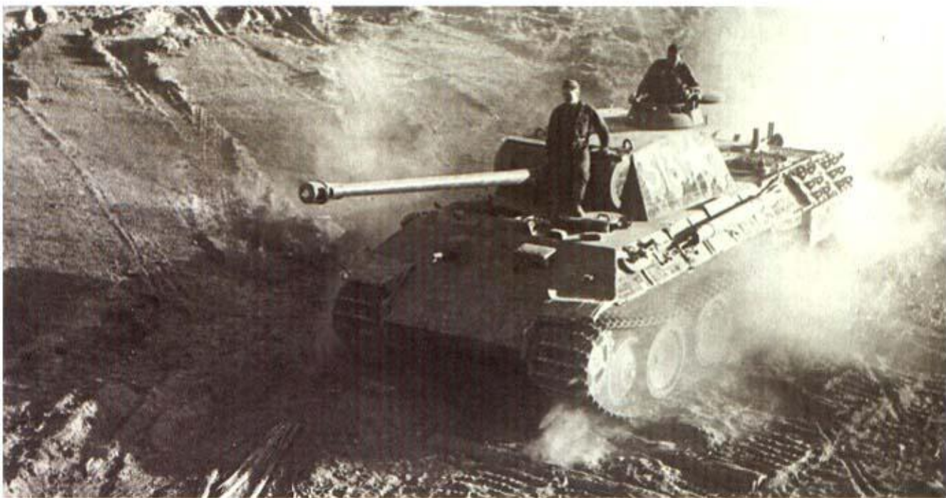
Above: This Panther, PzKpfw V Ausf A has been captured undamaged by the Red Army and is being driven at speed (possibly on test) - its top speed was just under 29mph. (TMS)
