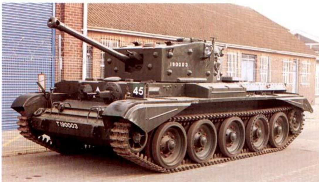
Right: Cruiser Tank Mk VIII, Cromwell (A27M) was light, fast and well armed with a 75 mm gun. British units brought back from the Middle East for D-Day, such as 7th Armoured Division, did not immediately like them, preferring their old Shermans. (TM)
