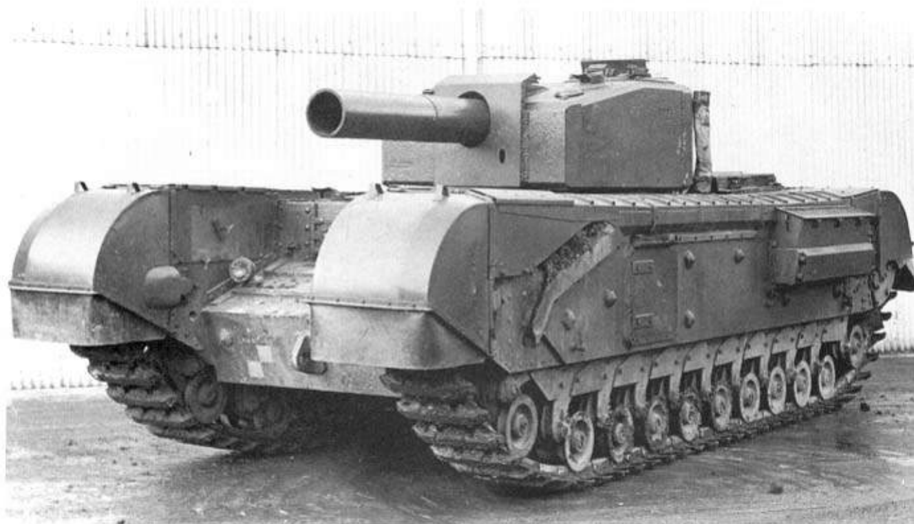
Above Ardeer Aggie, an experimental vehicle based on Churchill Mk III fitting a more powerful Petard mortar. (TM)
