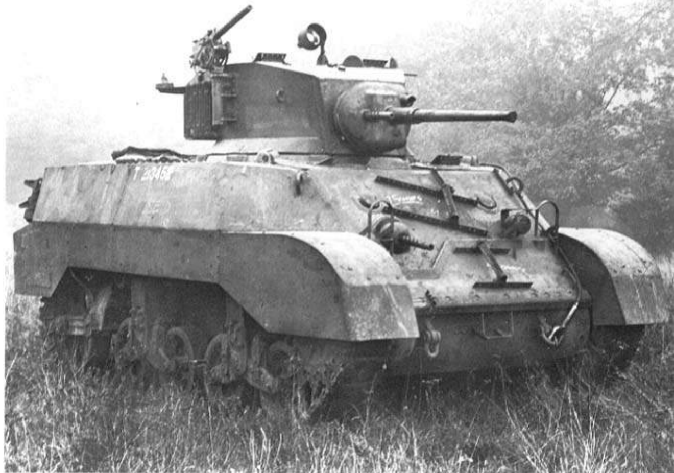
Above: The M3A3 had a larger, welded hull, allowing more room for larger fuel tanks and extra ammunition stowage. In British service it was known as Stuart V. (TM)
