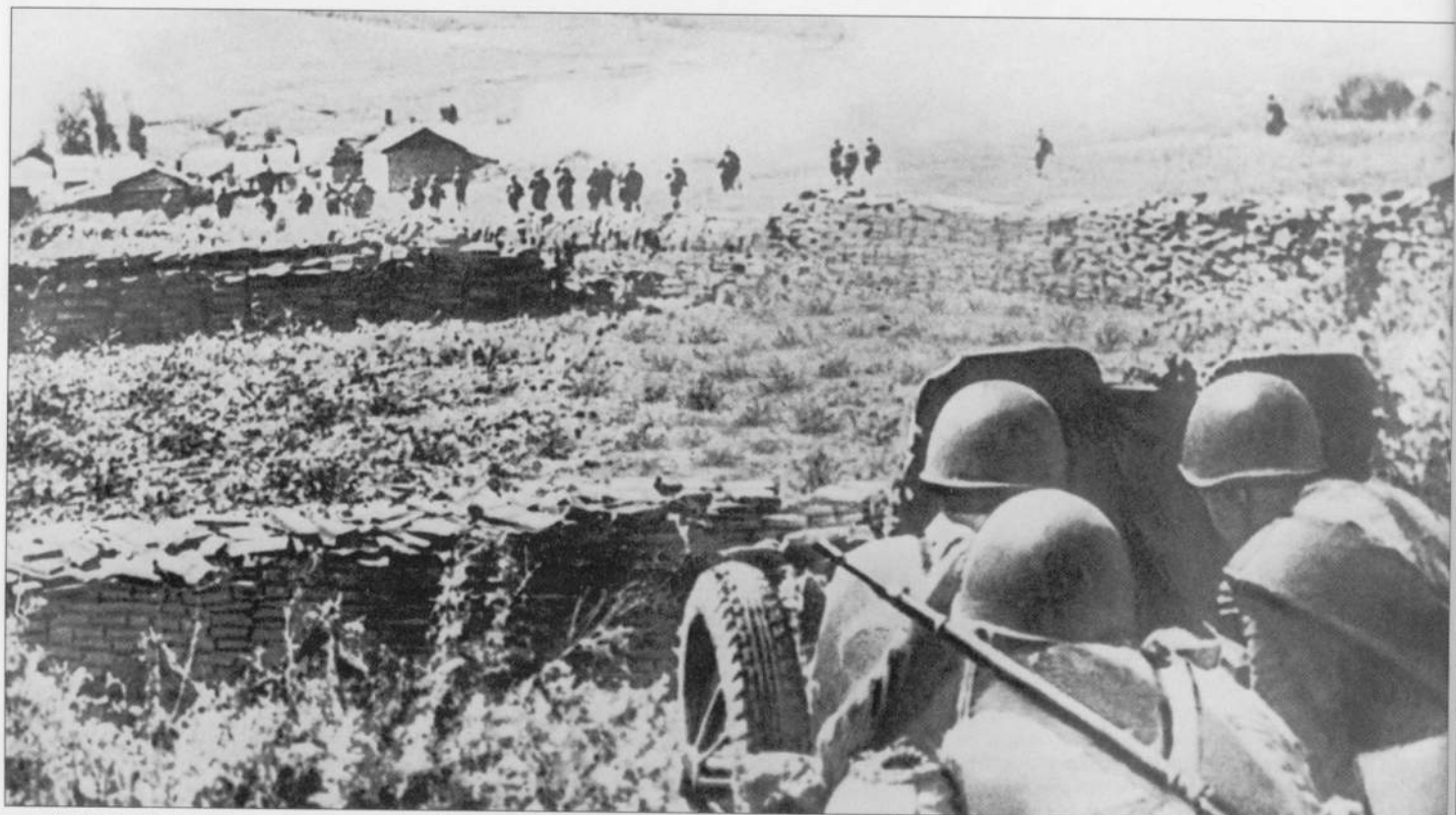
A group of anti-tank gunners covers the advance of attacking Soviet infantry in the vicinity of Kalach. The weapon they are using is a 45mm Model 1932 L/46 gun. This particular model, which was based on the German 3.7cm Rheinmetall PaK 35/36, weighed 510kg (1124lbs) in action and fired a 1.43kg (3.15lb) shell that was capable of easily penetrating 38mm (1.50in) of armor at an angle of 30 degrees at a range of 1000m (1094yd). A very effective anti-tank gun, it remained in service until the end of the war.
