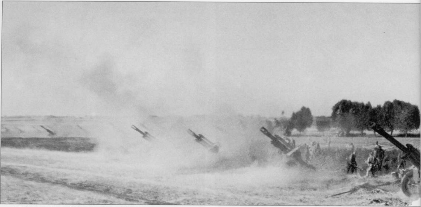
A battery of 152mm (5.98in) howitzers delivers a heavy, concentrated barrage on German positions north of Stalingrad. These big guns were more than capable of firing 40kg (88lb) high explosive shells or a 51kg (112lb) semi-armor-piercing shells with a muzzle velocity of 432m/s (472yds/sec). Each gun had a crew of seven. Working hard together, they could easily fire three or four rounds every minute.
