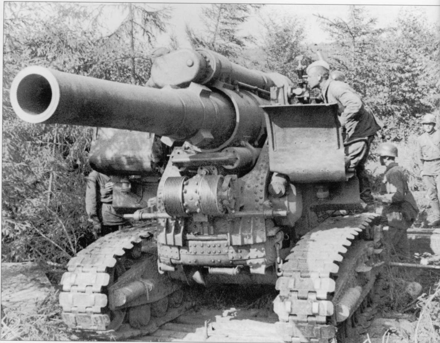
A Russian M1931 203mm howitzer is being loaded for action. A well-trained crew was able to keep up fire for many hours, despite its crude design. The Red Army used the howitzer widely on the Eastern Front. Firing a 98.5kg (217lb) shell, it was an especially effective weapon when used against immobile targets such as German strongpoints and when defending buildings.
