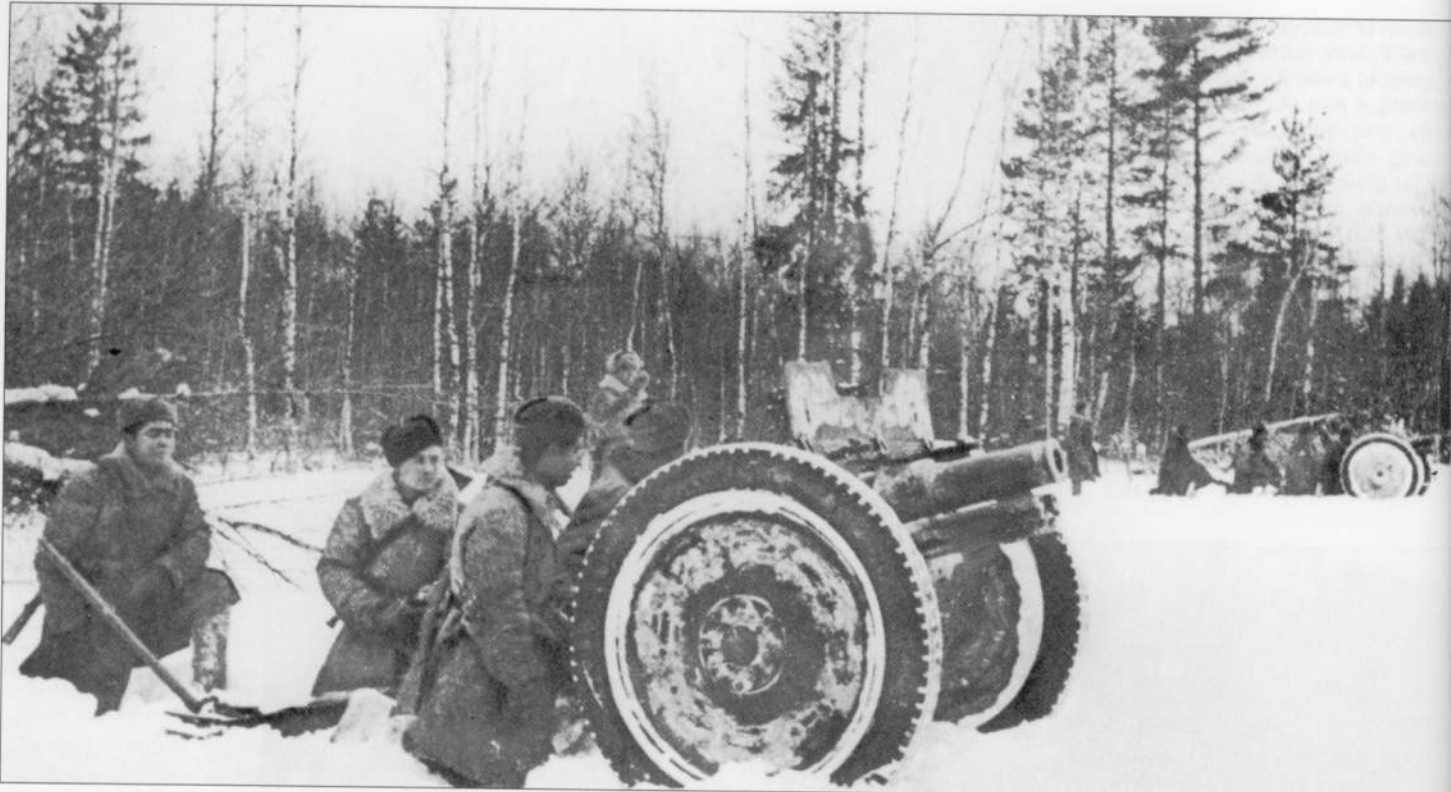
A battery of Model 1910/30 field howitzers in action. These veteran World War I howitzers were mainly used in the early years of World War II. They were upgraded during the 1930s with solid pneumatic-tired wheels. The gun could fire a 22kg (47.8lb) shell at a maximum range of 8,940m (9,771yd).
