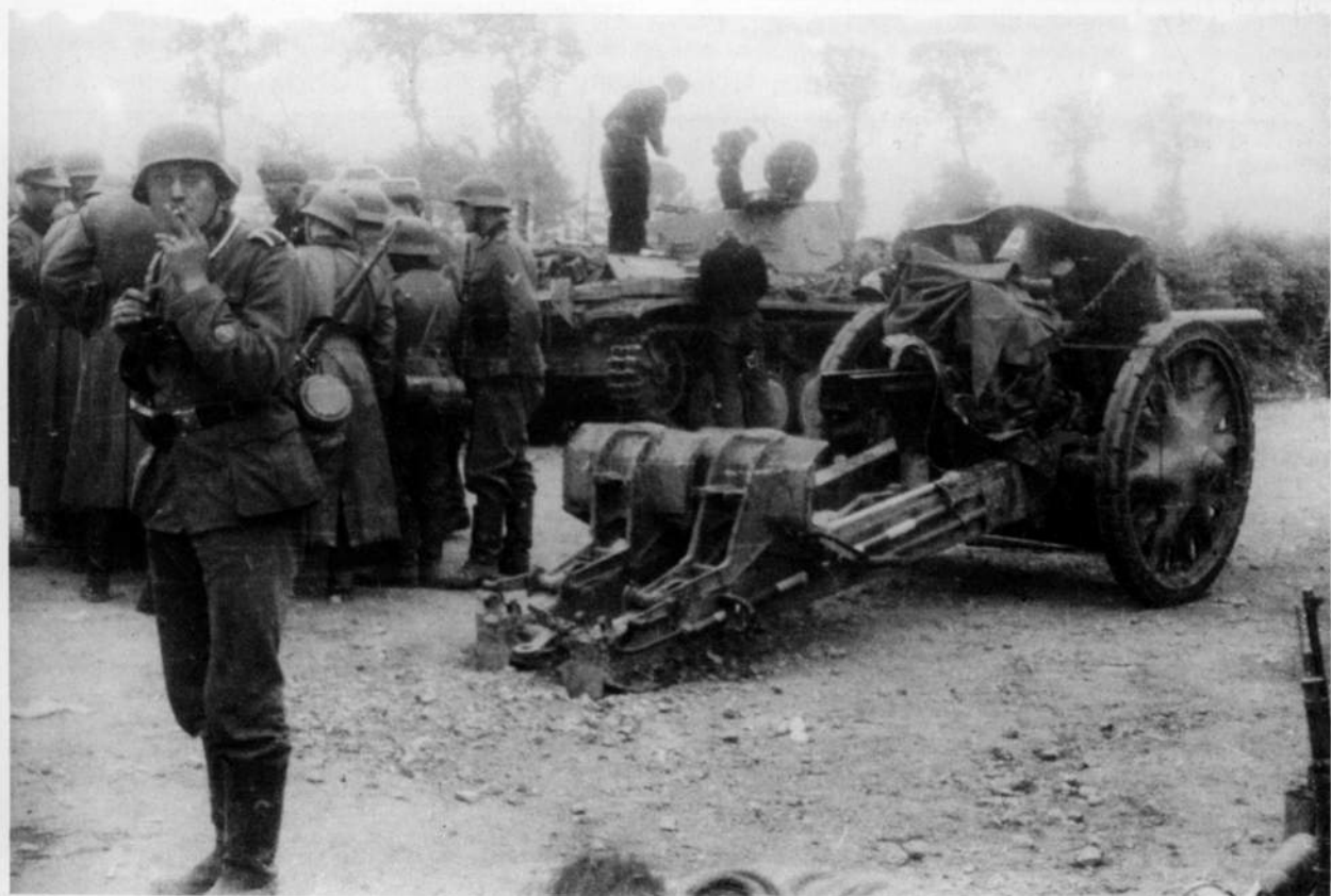
The mainstay of the divisional artillery was the 105mm light field howitzer M.18; this early model lacks a muzzle-brake.
