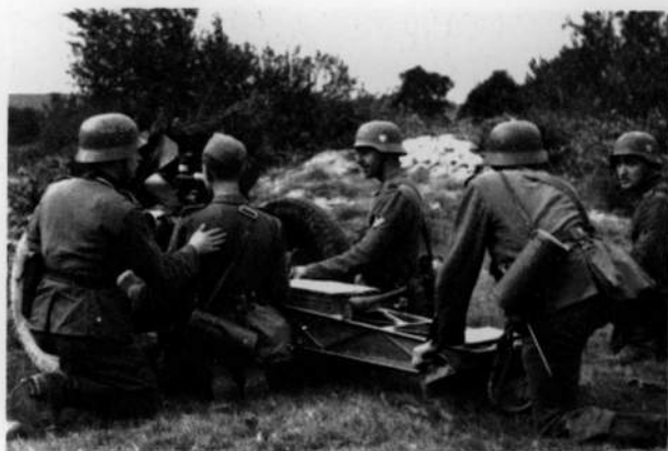
The 75mm infantry howitzer was the main integral support weapon of the Panzer-Grenadier regiments; it was later replaced by the 150mm infantry gun.
