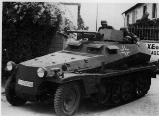
SdKfz 250/10 half-track with 37mm gun, as used by the division's reconnaissance battalion. The divisional sign and a tactical marking can just be made out painted on the top surface of the engine deck, forward of the hatches.
