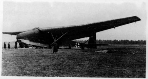
The supply of forward armoured units during speedy advances became a major problem due to the inadequate railway network and Russia's few and primitive roads. In October 1941 6th Panzer was partly supplied by means of Me 321 'Giant' gliders. These huge machines had a wingspan of 18ft.; a payload of 21½ tons was accommodated in a cargo bay the size of a railway freight wagon.
