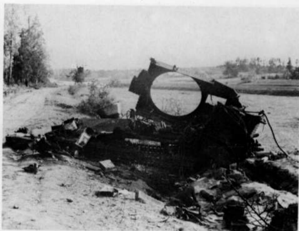
A PzKpfw 35(t) totally demolished by a Soviet bomb which fell into its open hatch.
