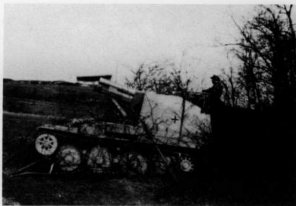
The heavy gun company of each Panzer-Grenadier regiment had six 150mm infantry howitzers on the 38(t) tank chassis (SdKfz 138/1), with a maximum range of 4,700m.
