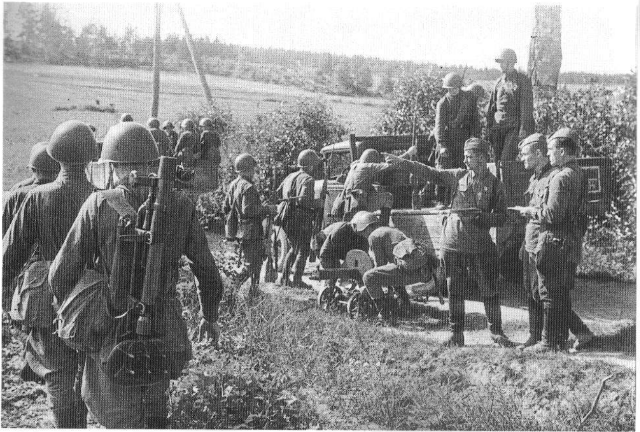
The heavy weapons company of a rifle battalion mount up on a GAZ-AA truck. The soldier to the left is carrying a 50-PM 38 mortar. Two soldiers near the truck are loading a 7.62mm Maxim Model 1910 machine gun aboard, on its characteristic wheeled mounting.
