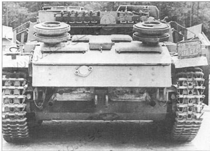
The rear of Sturmgeschütz Ausf. G, Fgst.Nr. 92112, which was used as a test vehicle for the steel-tired rubber-saving wheels. The new centre tow coupling for tow bars was introduced into production from December 1944. (TM)
