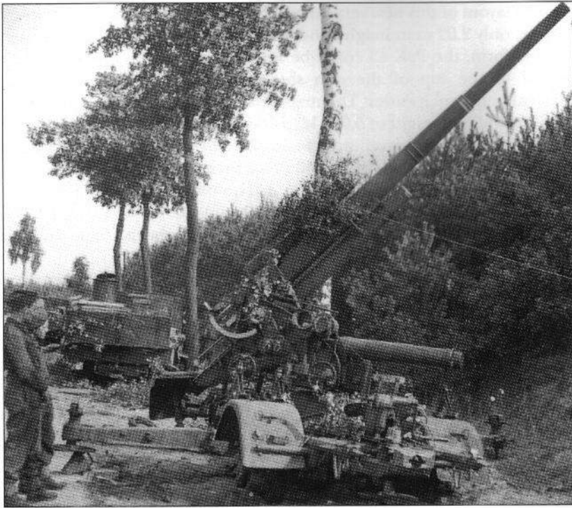
Abandoned 88 mm FlaK 37 gun being examined by British troops as they advance towards the L'Escaut Canal near the Dutch border. It appears that the crew used the trees as natural camouflage to screen the gun from Allied aerial reconnaissance.
