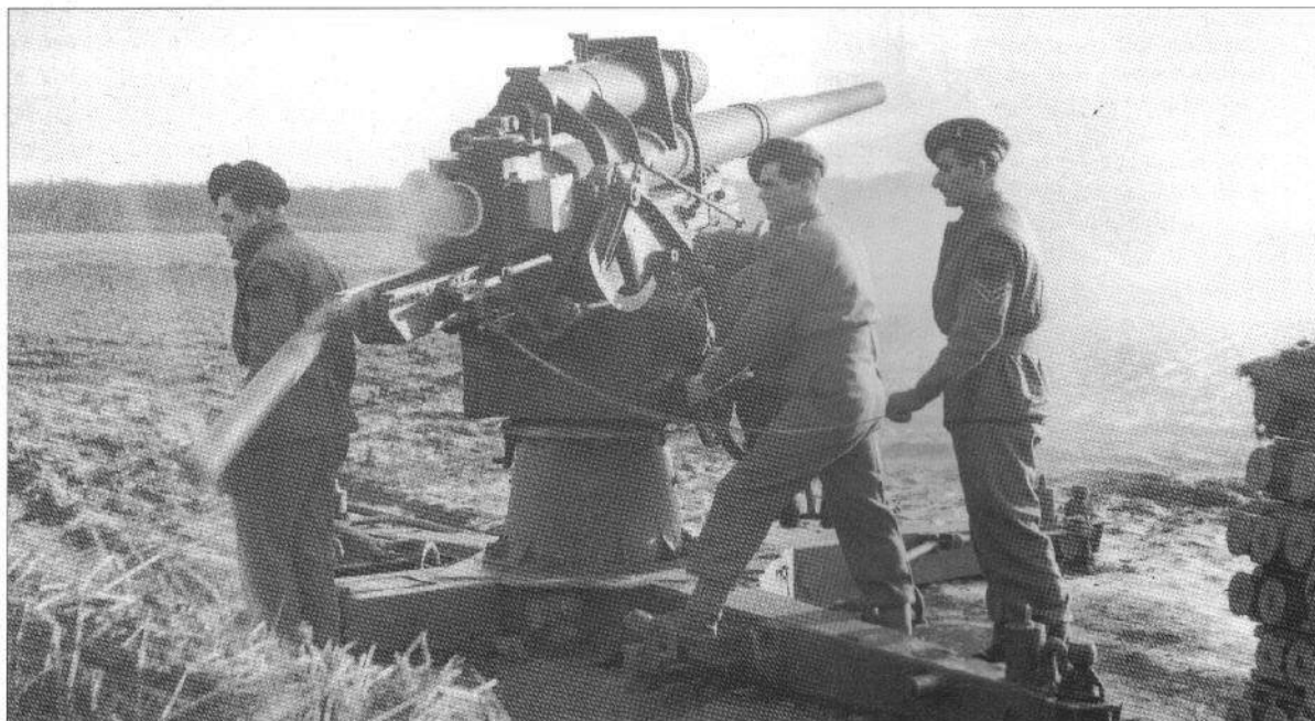
BELOW AND RIGHT Men of 172 Battery, 58 Light Anti-Aircraft regiment, Royal Artillery using 88 mm guns against their former owners, December 1944. Note the spent shell cases being ejected and the man at right holding a firing lanyard. Each of the wicker-type ammunition cases contain three shells.
