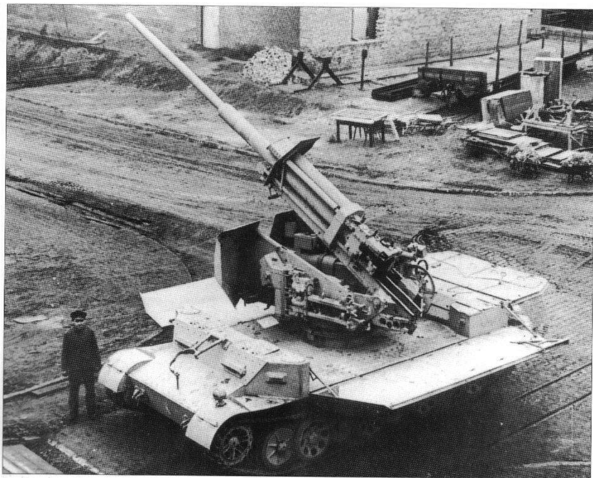
The VFW 1 fitted with the barrel of a FlaK 41, seen here at the Krupp works in Essen. Note the side panels which are lowered to permit all-round traverse of the gun. It never entered service.
