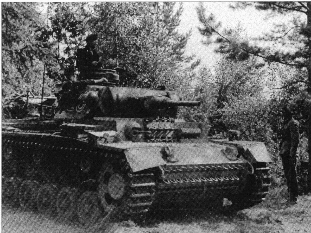
Panzer III on the Eastern Front 1941. It still has the 5-cm gun, which was to prove so inadequate against the Soviet T34s. (Robert Noss)
