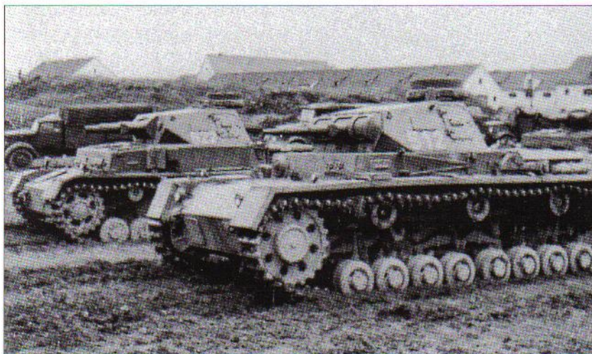
Panzers on the training grounds. Although at first glance these rare vehicles look like Panzer IVs with eight roadwheels, they are in fact Panzer IIIbs, of which only 15 were built, in 1937. Later versions of the Panzer III had only six roadwheels. (Robert Noss)
