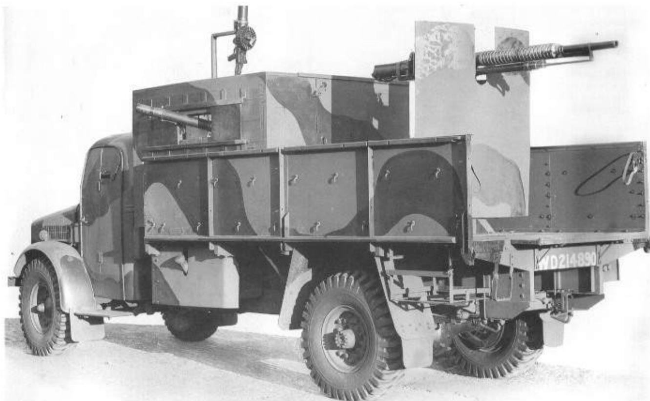
Above: Armadillo MkIII mounted a 1.5 pounder COW gun in a blockhouse, with up to three Lewis guns (one on an AA mount), plus a rear-mounted heavy machine gun. One of a number of slightly different models converted from Bedford 3-ton chassis. (TM)
