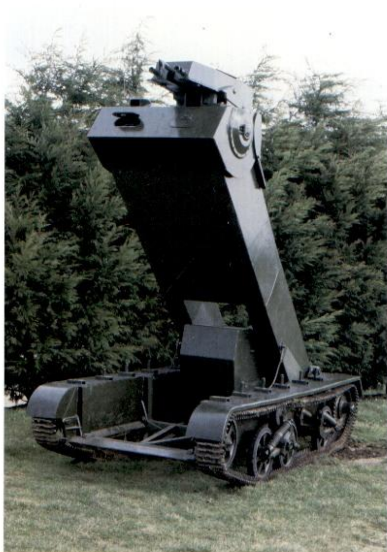
Above: Praying Mantis , a conversion on the Universal Carrier chassis, which mounted twin Bren LMGs in the 'head'. (TM/Roland Groom)
