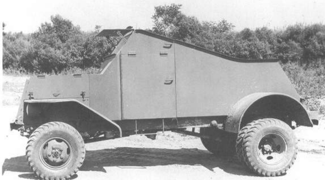
Left: The Chrysler scout car 1941, with a simple armor plate body bolted to a 1.5 ton 4x4 Dodge truck chassis. (TM)
