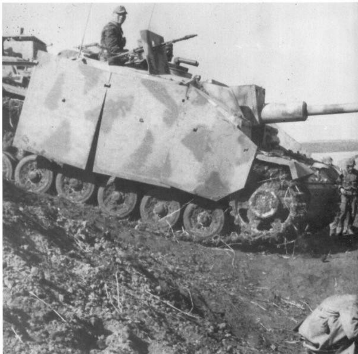
Right: Sturmgeschütz 40 Ausf G (also called the Stug III Ausf G ) assault gun/tank destroyer negotiates a Soviet anti-tank ditch. The main armament was the 7.5cm StuK 40 L/48 gun. Note also the armoured shield on the machine gun by the loader's hatch and the peri-binoculars on the commander's cupola.
