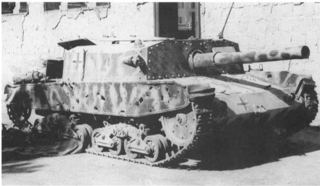
Left: The Semovente M43 105/25 mounted a 105mm gun, carried a crew of three and weighed some 15.7 tons. This one has German markings. (TM)
