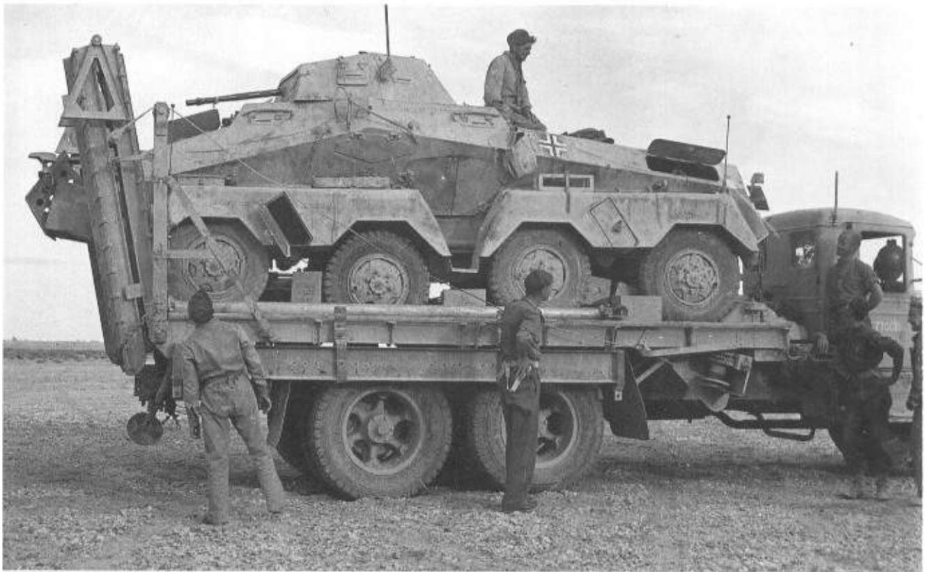
Above: An SdKfz 231 8rad, captured by the British. Main armament was one 2cm KwK30 and a co-ax MG34. (TM)
