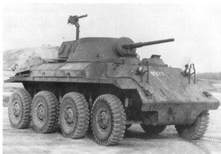
Top: The T18E2 Boarhound armored car of 1942 followed on from the T18 pilot model. Built for the British but only thirty were ever completed. (TM)
