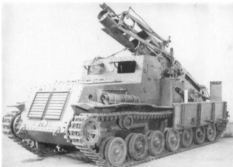
Above: Built in 1943, the HA-TO mounted an enormous 300 mm trench mortar on the open rear deck. (TM)
