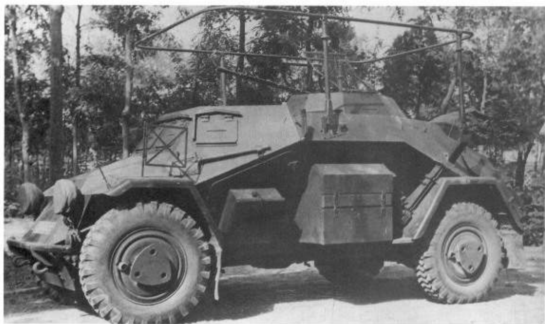
Above: The SdKfz 232 6rad (Fu) was the radio version of the six-wheeled SdKfz 231. Note the distinctive frame-type aerial. (TM)
