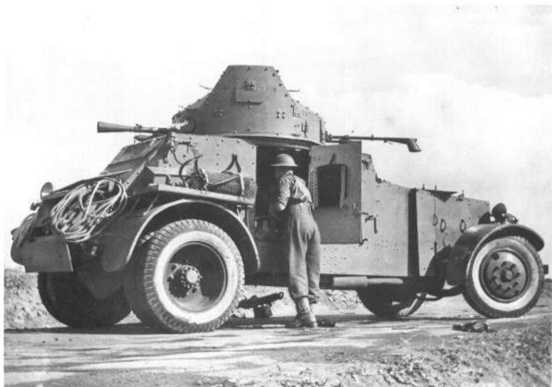
Right: This White-Laffly Automitrailleuse was rebuilt from First World War stock in 1925 with a raised hull and pneumatic tyres. This one was captured in North Africa, November 1942. (TM)
