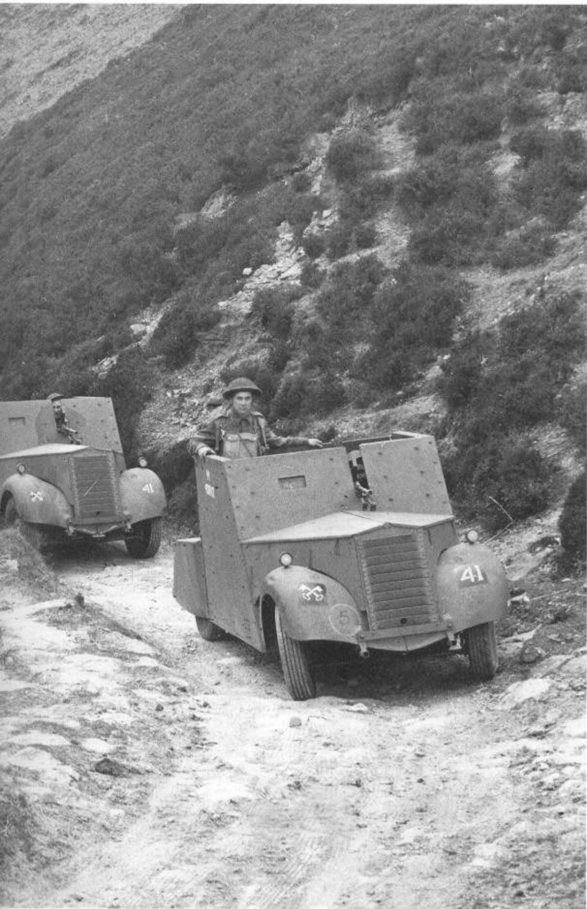
Left: A column of Beaverette MkIIs on training 'somewhere in England'. The MkII had better all-round armour. They are from armoured car regiment (41) of 2nd Infantry Division (Crossed Keys). (TM)
