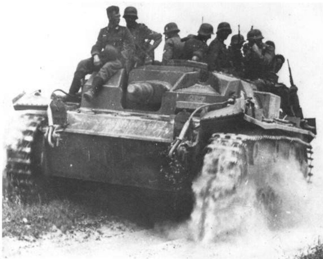
Left: Stug III Ausf A/B assault gun mounting a 7.5cm StuK 37 L/24 gun. This one is carrying Panzergranadiers into action. (TM)
