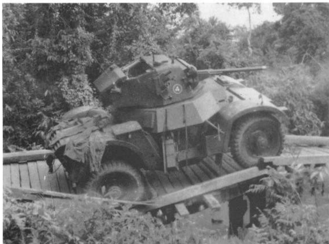
Below: An AEC Mkl heavy armoured car, which mounted a 2 pounder gun and co-ax BESA, in a two-man turret very similar to that of the early Valentine tank. (TM)
