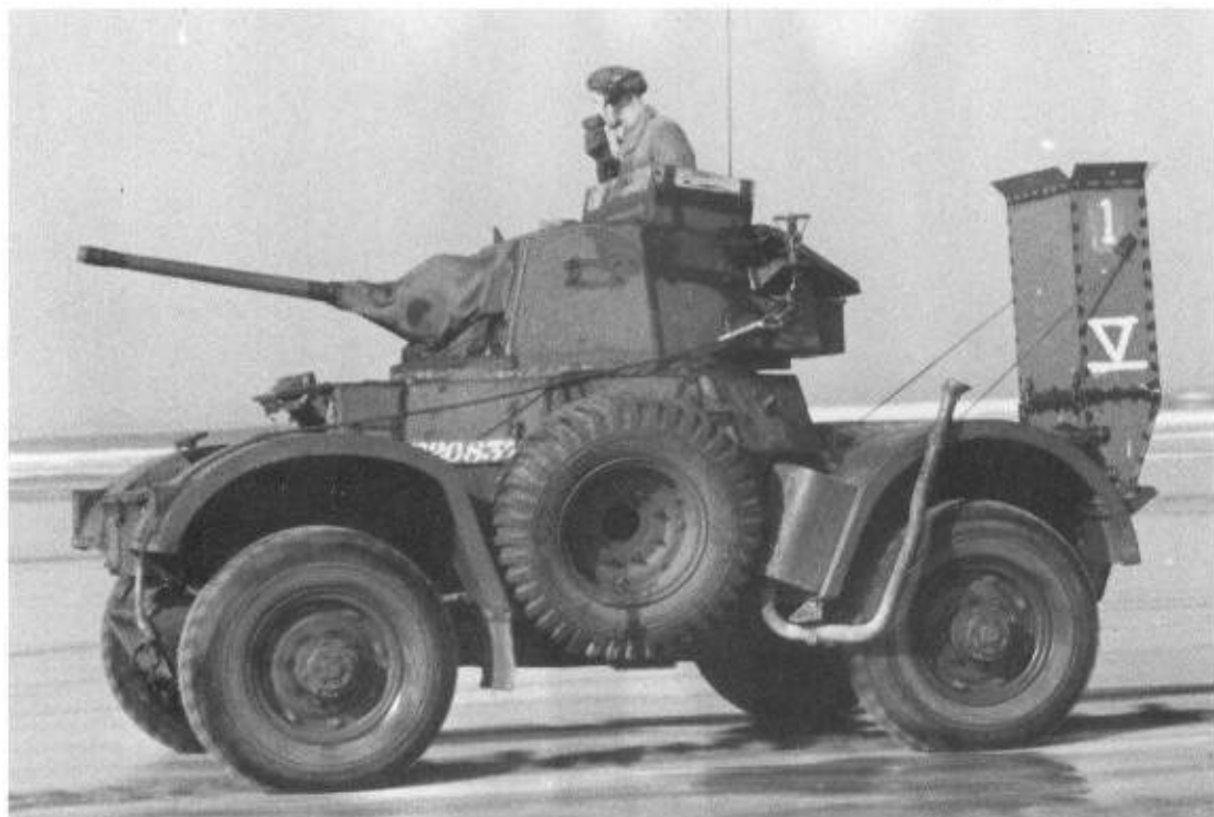
Right: A Daimler armoured car fitted with amphibious equipment during deep wading trials held in 1944. Note the gun apron, radiator duct and flap-valve over the exhaust (submerged whilst wading). (TM)
