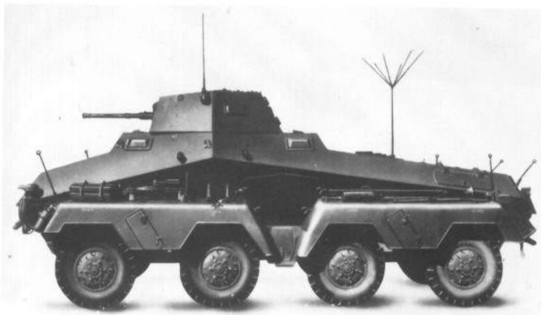
Left: This SdKfz 232 8rad (Fu) is fitted with a single rod-type aerial on the turret and a star-shaped aerial on the rear deck. This replaced the cumbersome frame-type aerial. (TM)
