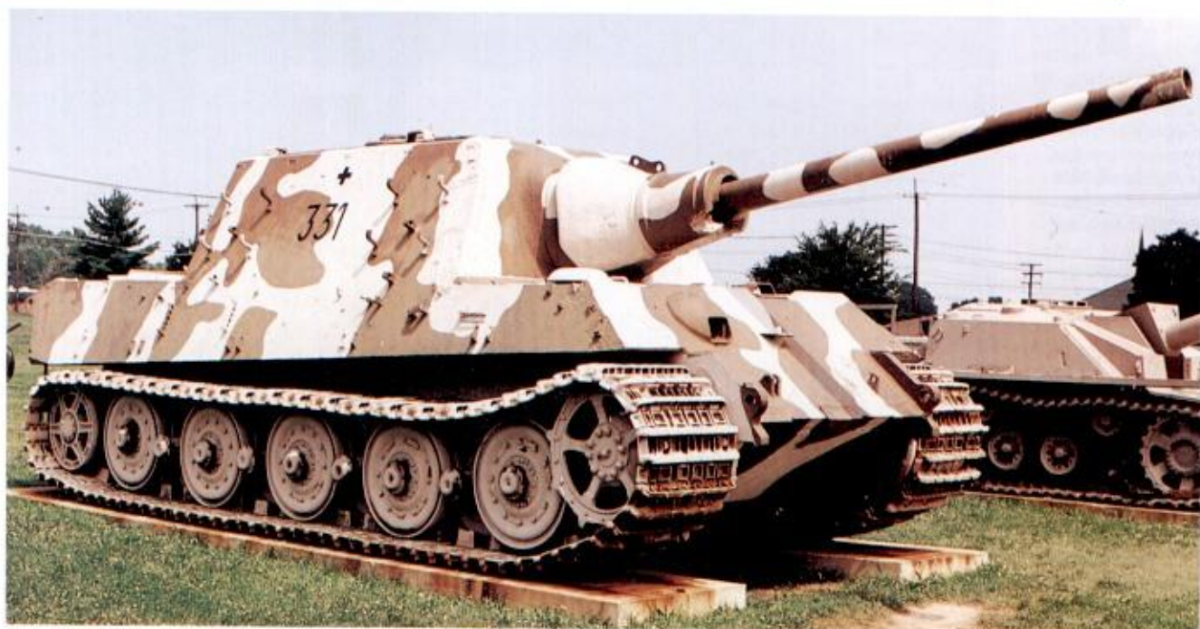
Below: Heaviest AFV to see action in World War Two was the Jagdtiger SkKfz 186, only seventy-seven of which were built. It was almost invulnerable to enemy fire due to armour up to 250mm thick. The author saw one which had wiped out almost an entire regiment of Shermans in the Ardennes. (RJ Fleming)
