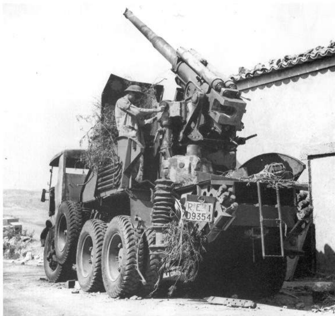
Left: Ansaldo 90/55 gun model 41 on a Breda Tipo 51 heavy 6x4 truck chassis, fitted with six large side jacks for stability whilst firing. This one was abandoned in Sicily, August 1943. (TM)
