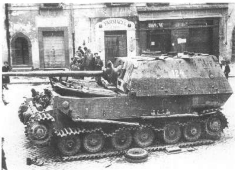
Below: Badly damaged, this 65-ton Elefant (Elephant) heavy assault gun, stands in a shattered Italian town's main street, it's 8.8cm gun silent forever. (GF)
