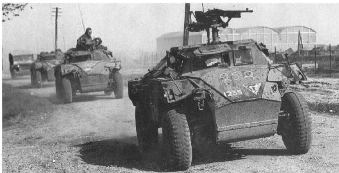
Above: Humber Mk1 scout car. So great was the demand for scout cars that other firms were asked to produce them, including the Rootes Group who built the heavier (3.19 tons), slightly larger Humber. (TM)
