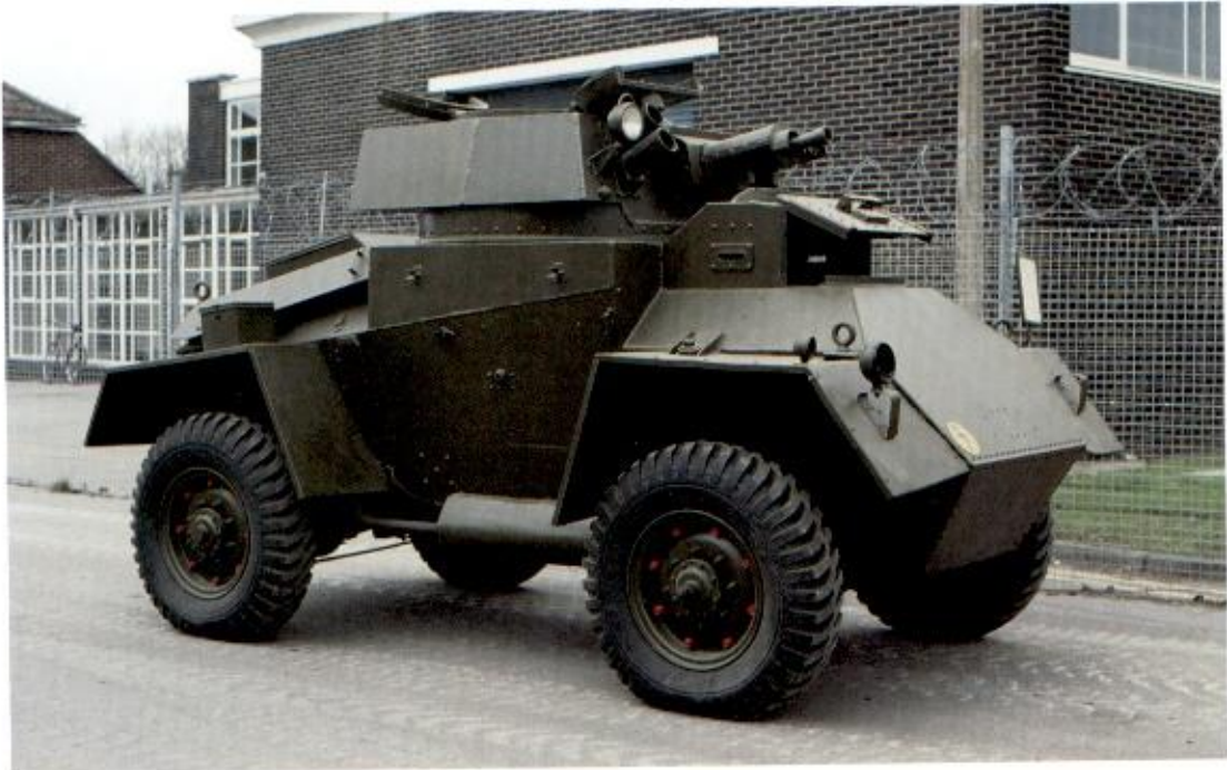
Right: A Guy Mk I armoured car, built in 1939, was also known as the Guy Wheeled Light Tank. It was the first all-welded armoured car produced for the British Army. (TMI/Roland Groom)
