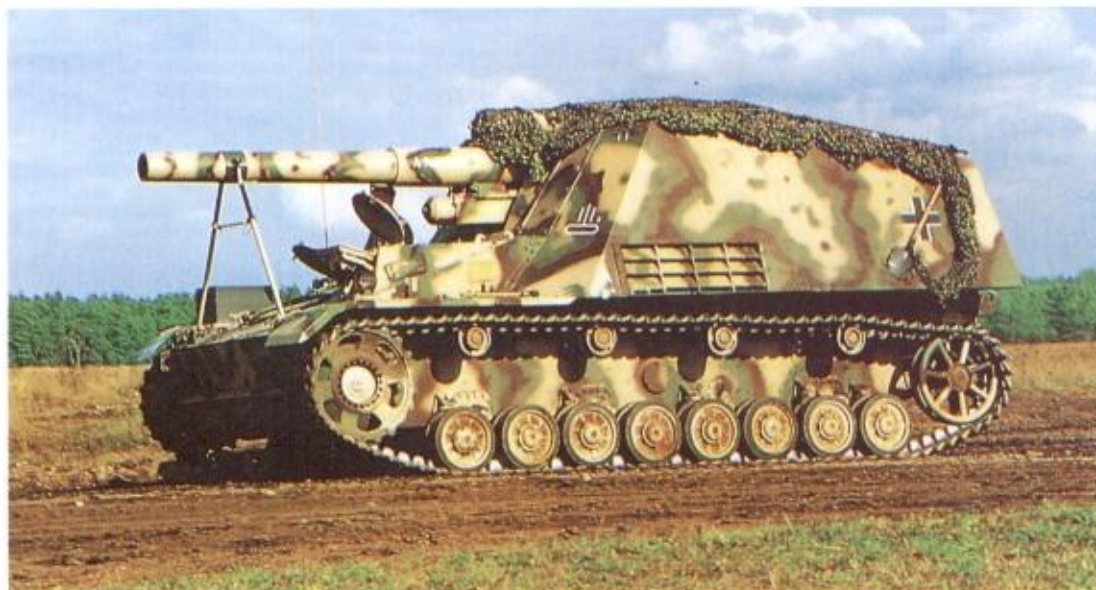
Right: Also on display in the Panzermuseum is Hummel , the 15cm schwere Panzerhaubitze auf Geschützwagen IV, SdKfz 165, a most effective SP heavy howitzer, built to provide Panzer units with artillery support. (Panzermuseum)
