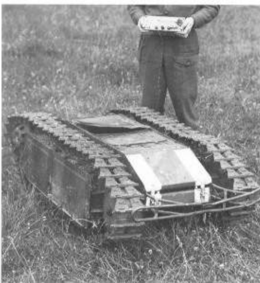
Left: Goliath SdKfz 303 leichter Ladungsträger was a remotely controlled, expendable tracked demolition charge vehicle, of which there were two types, this is the heavier version. For long-distance transportation it could be carried on a purpose built two-wheeled trailer. (TM)
