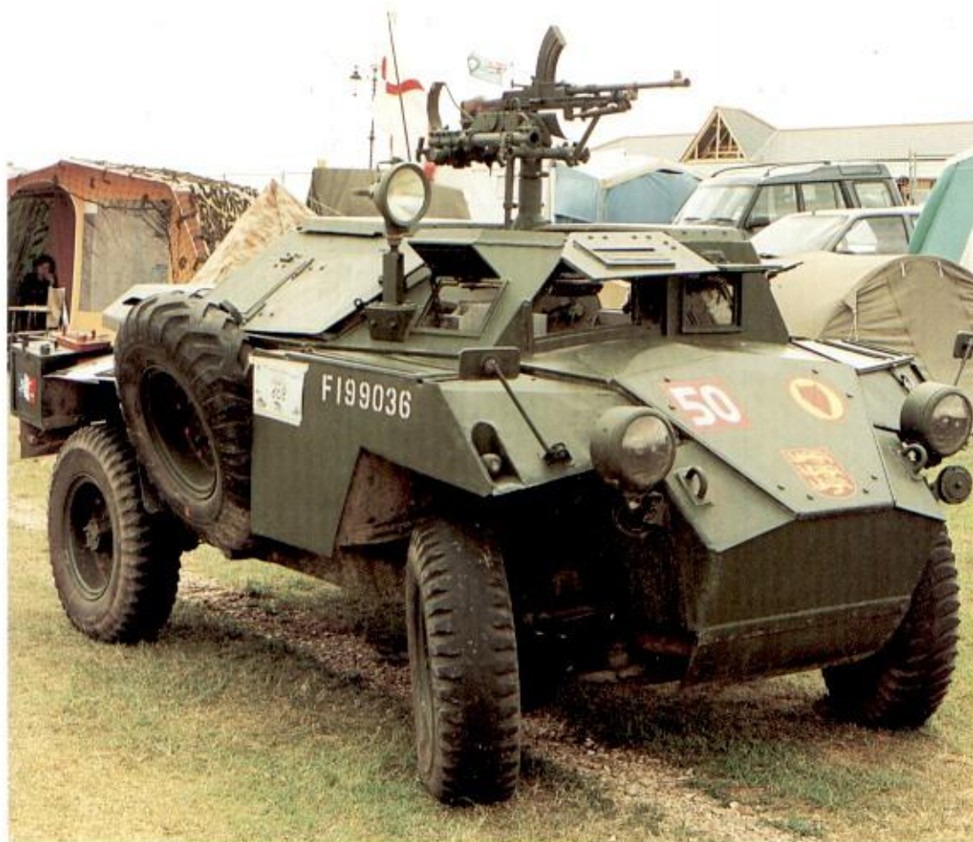
Left: Humber scout car, with a pintle-mounted Bren LMG. The formation sign - a red fox mask on a yellow disc, denotes 10th Armoured Division, whilst '50' shows it belonged to the armoured brigade headquarters. (TM/Roland Groom)
