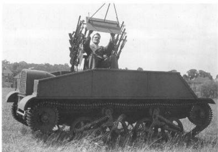
Above: A Loyd carrier fitted with six Bren guns in an AA mount. (TM)
