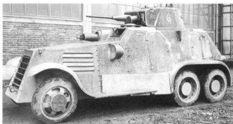
Top: The Swedish-built Landsverk 181 armoured car used a Scania Vabis 6x4 truck chassis and mounted a 20mm gun in conventional looking turret. (TM)
