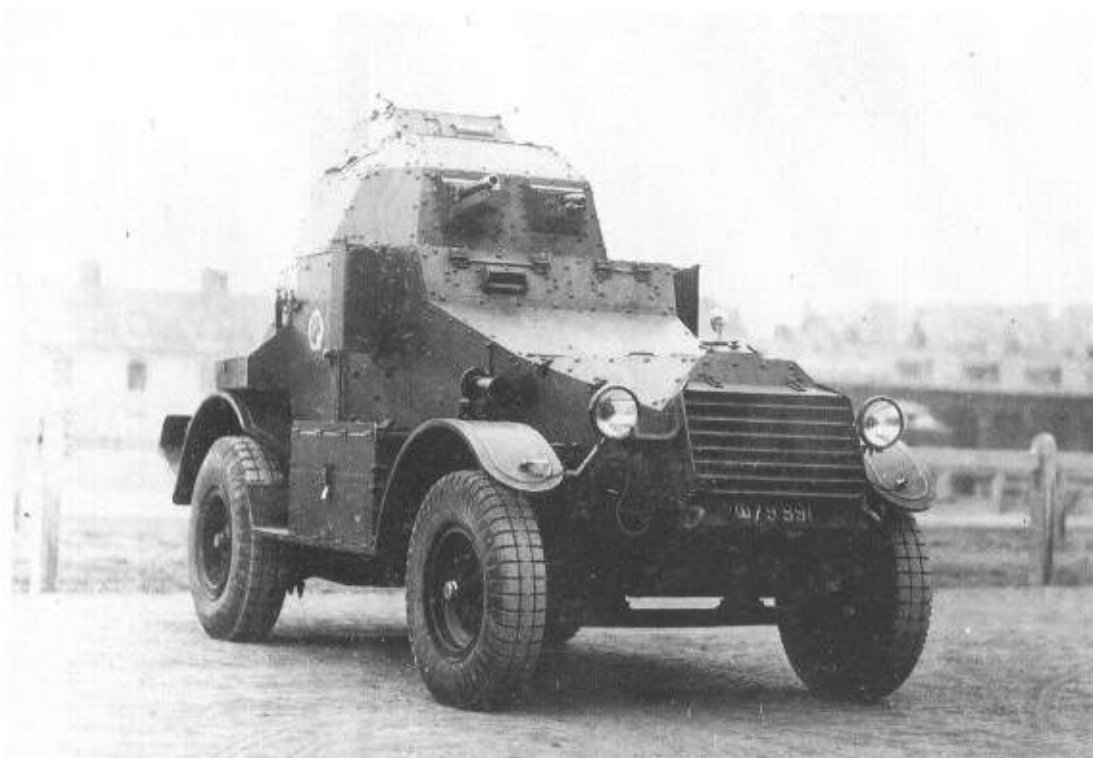
Left: An AMD Panhard 165/175 TOE, built in 1933, was a later model of the Panhard AM 20 CV, with armour 9 mm thick and weighing 6.7 tons. (TM)
