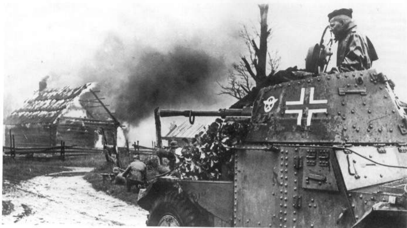
Above: An AMD Panhard 178 here in German service in Russia when it was known as the Panzerspähwagen Panhard 178-P204(f). It was a good armoured car, weighing some 8.2 tons and mounting a 25 mm cannon. (TM)
