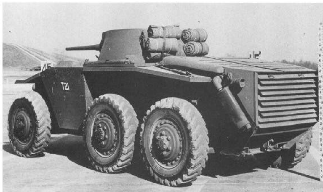
Above and left: Front and rear views of the Studebaker-built T21 6x4 armored car of 1942. It was also designated as the T43 GMC. (TM)
