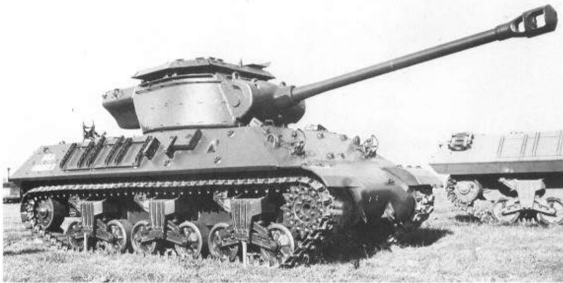
Left: The M36B2 used the M10 hull and was fitted with an armored canopy over the open-topped turret. It mounted a 90mm AA gun adapted for anti-tank fighting. This was the US Army's best anti-tank gun of World War Two. (TMI)
