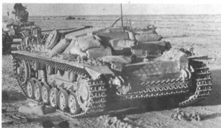
Above: The Stug III Ausf C/D did not have the gunner's direct vision port and improved armour. (TM)
