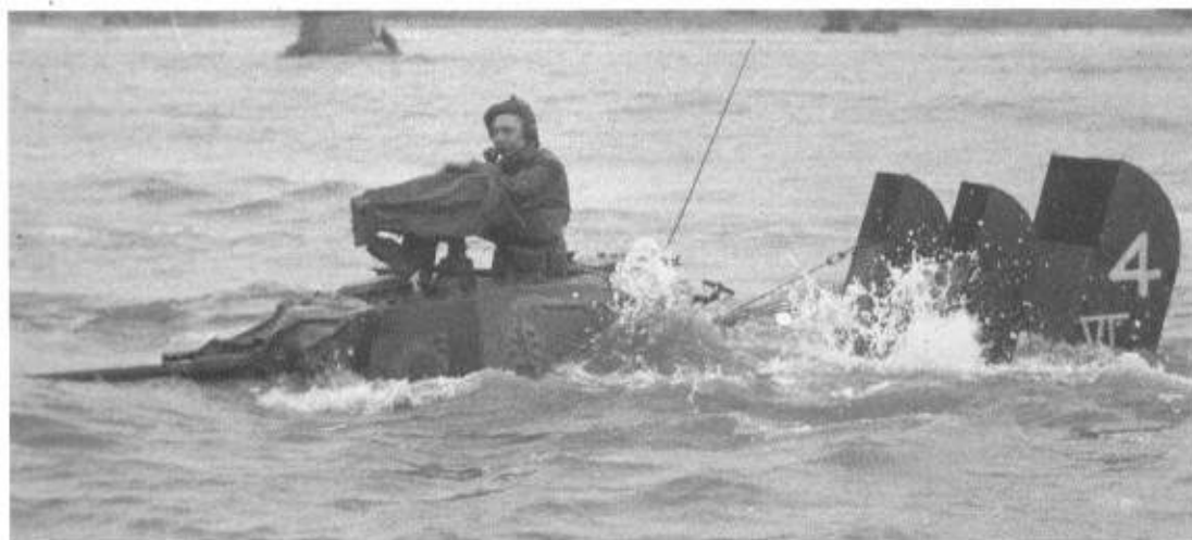
Left: This Daimler armoured car is almost submerged during amphibious trials. The driver would have worn the same underwater escape apparatus as the crews of DD tanks. (TM)
