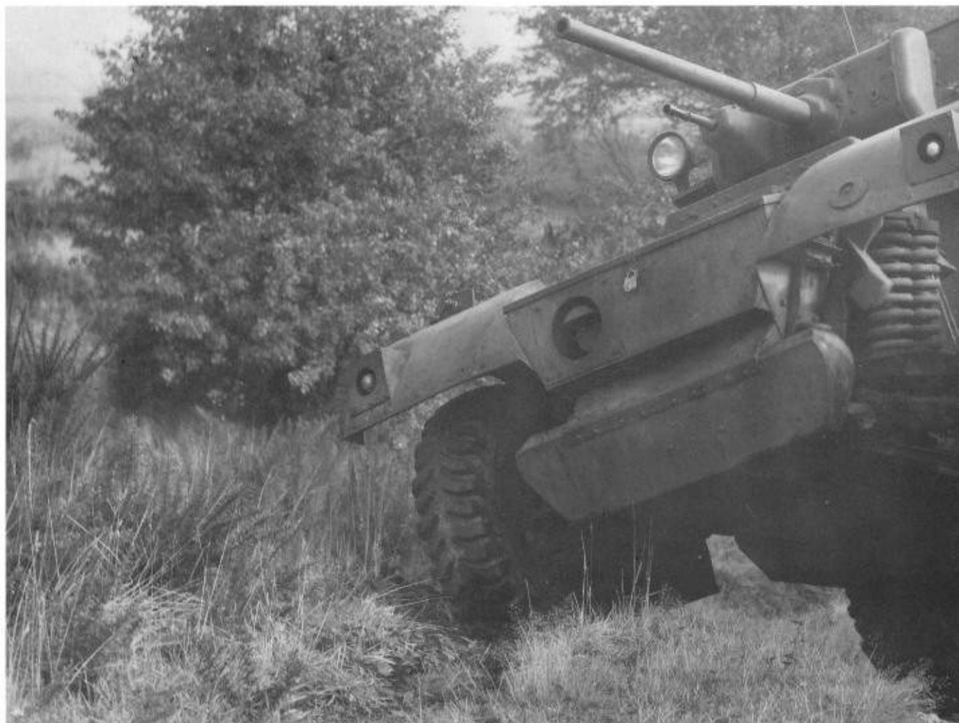
Right: A Daimler armoured car fitted with amphibious equipment during deep wading trials held in 1944. Note the gun apron, radiator duct and flap-valve over the exhaust (submerged whilst wading). (TM)
