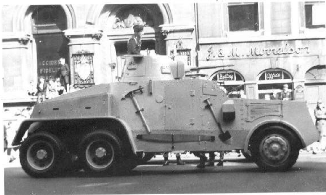
Above: Two Ford Mk VI armoured cars move through a village in Eire, March 1942. Armed with a single Vickers .303in MG, the 14ft 10ins long car had a top speed of 40 mph. (TM)
