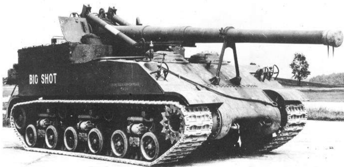
Above: The T83 chassis was used for both the M40 GMC 155mm gun (shown here) and the M43 8-inch howitzer. (TM)
