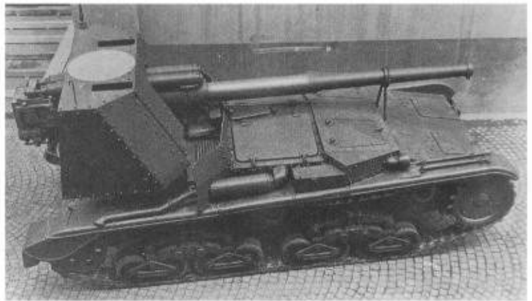
Left: Largest of the Semovente was the 149/40, which was due to go into mass-production by the end of 1943, but was cancelled after the Italian surrender. (TM)
