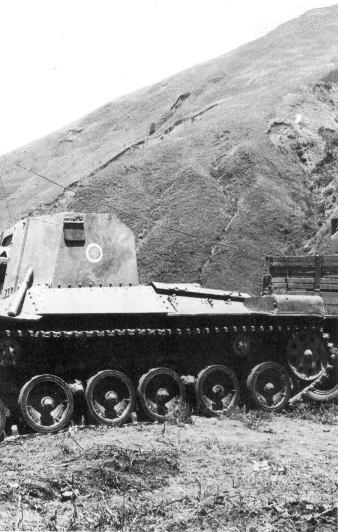
Left: The HO-N II mounted the long-barrelled 75mm Type 90 gun in an open-topped turret. (TM)
