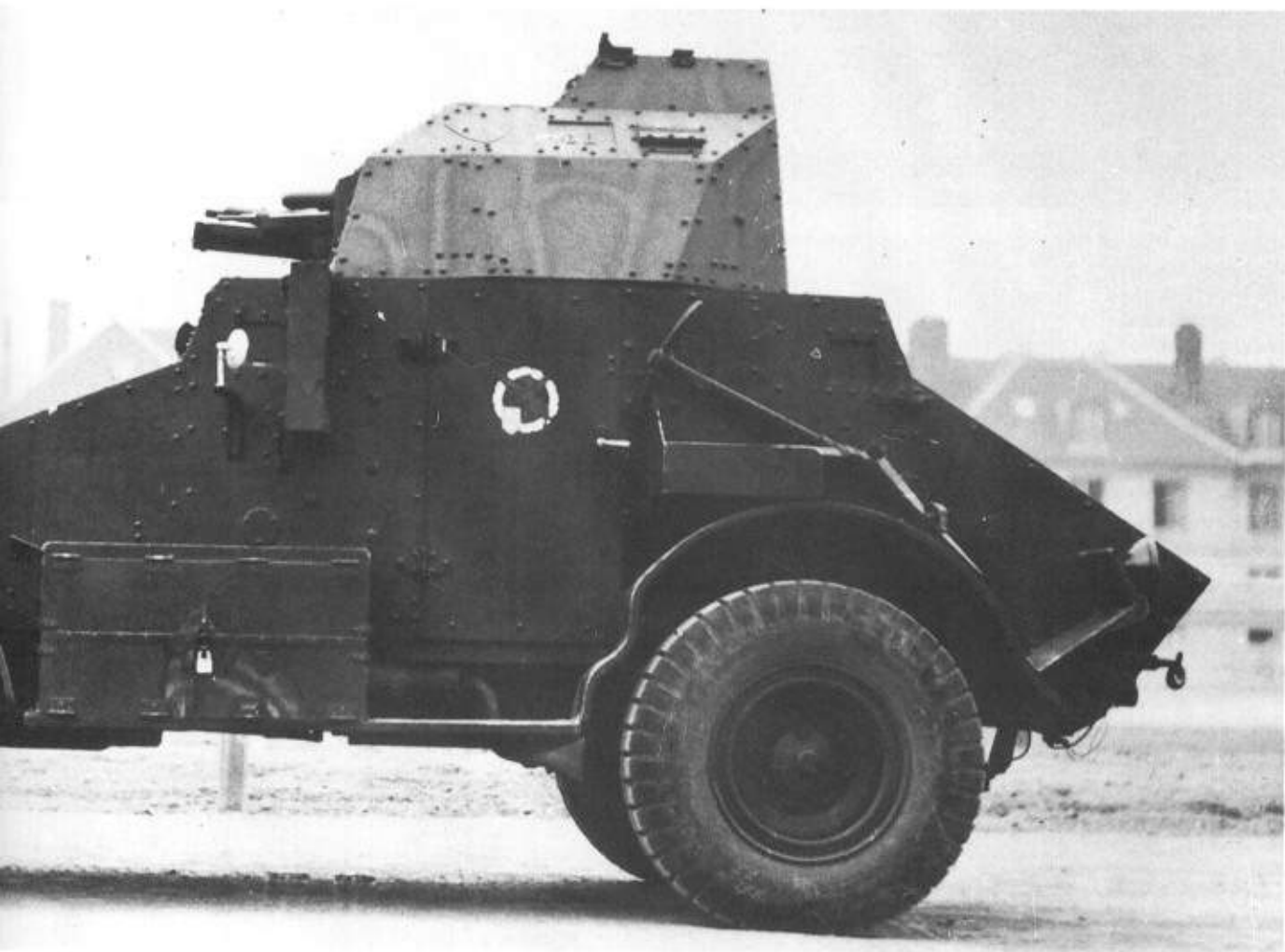
Below: Side view of the AMD Panhard 165/175 TOE. Its chassis was 17ft 6ins long had a faceted turret and disc wheels. (TM)
