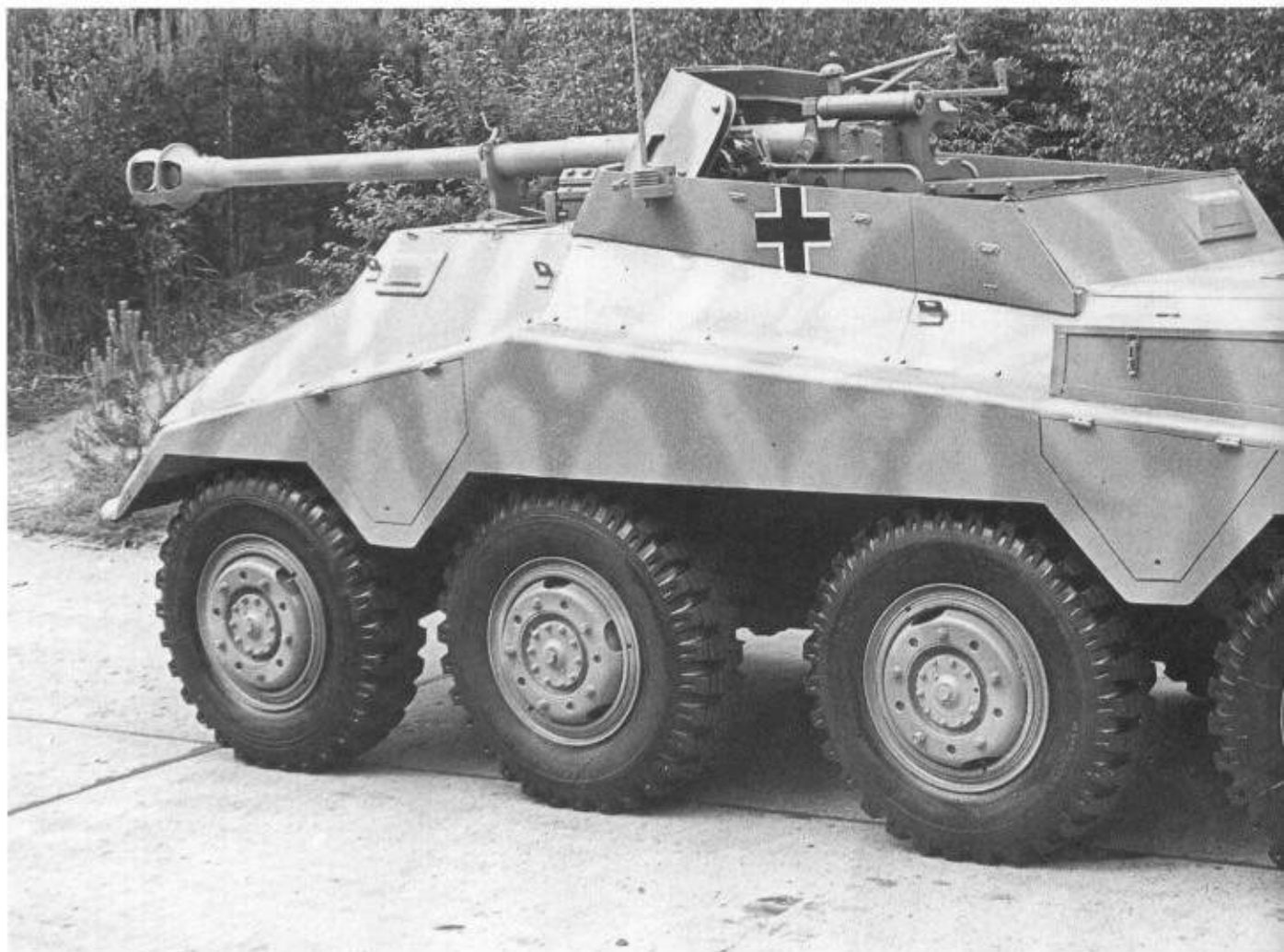
Above: SdKfz 234/4 Brad, mounted a 7.5cm PaK40 gun to provide close anti-tank support to other armoured cars. This one is displayed in the Panzer Museum, Munster, Germany.
