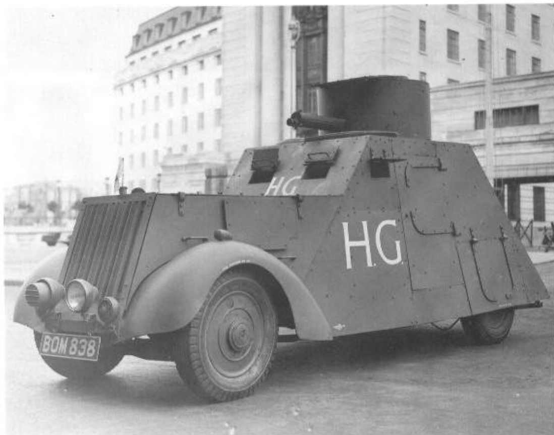
Right: The London County Council Home Guard Battalion took over this good-looking armoured car, built in the Council's workshops during August 1940. It mounted a Vickers machine gun and carried a crew of three. (TM)
