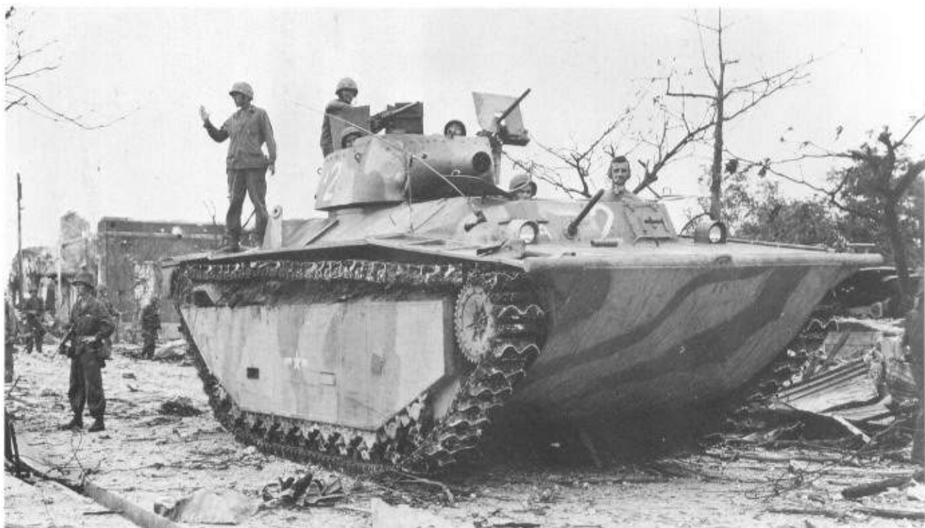
Above: The LVT(A)4 carried 100 ammunition rounds for the 75mm howitzer, exactly the same load as the M8 HMC. A total of 1,900 were built. (TM)
