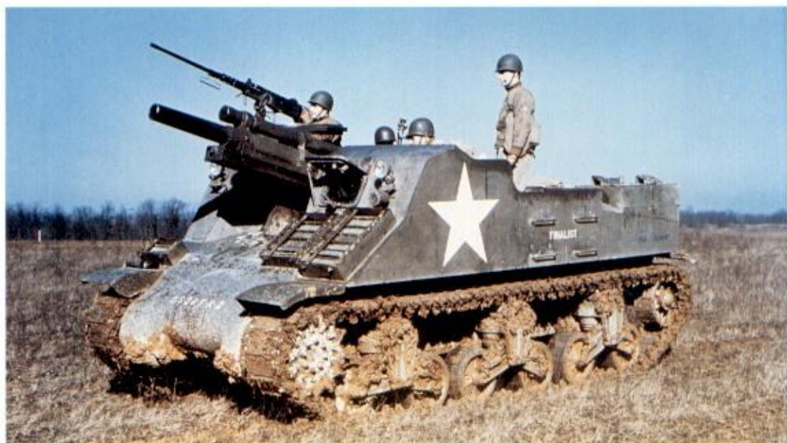
Right: Another view of the Priest, showing four of the seven-man crew and the pulpit-mounted .50in Browning heavy machine gun. (Patton Museum)
