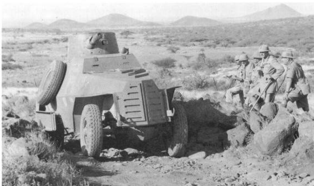
Right: The later version of the Marmon-Herrington MkII had a welded hull with the side doors fitted further back on the body. This one was photographed in Eritrea, 1940. (TM)
