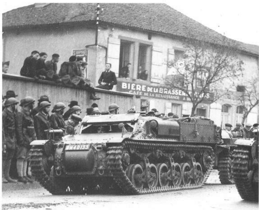
Above: The diminutive 2-ton Renault Chenillette was used for a wide variety of tasks. Much of its design was derived from the British Carden-Loyd. (TM)
