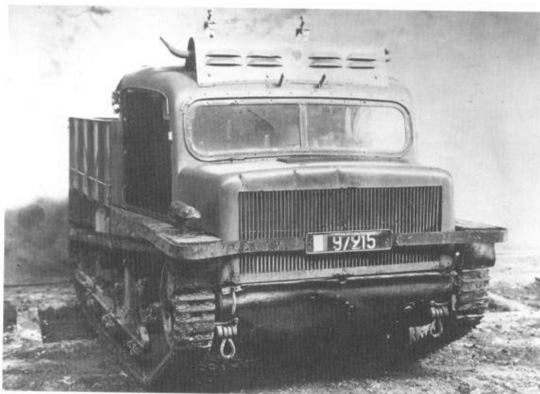
Left: An interesting version of the Renault Chenillette , fitted with a truck cab and body. (TM)
