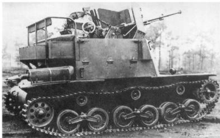
Below: The SO-KI twin 20mm anti-aircraft guns on a lengthened KYU-GO chassis. (TM)
