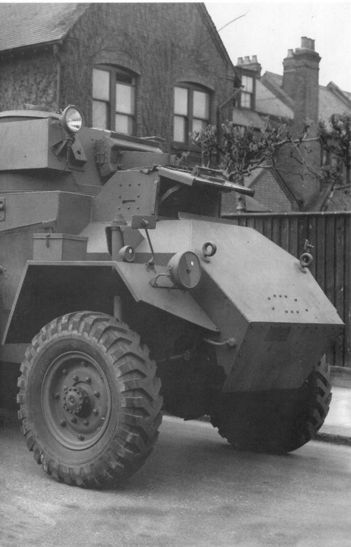
Left: The Humber Mk1 armoured car was designed using the pre-war Karrier KT4 artillery tractor chassis. (TM)
