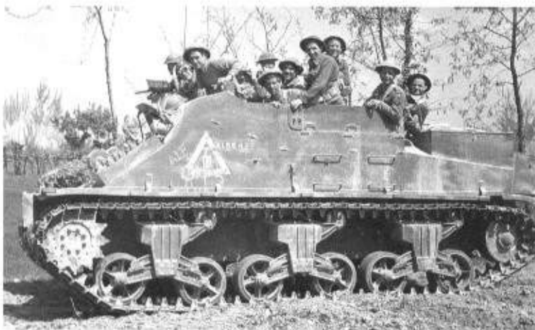
Below: British adaptation of the M7 was the Priest Kangaroo armored personnel carrier (APC), which could carry up to twenty fully-equipped soldiers and two crew. (TM)
