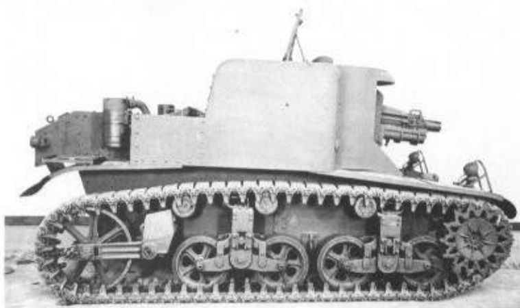
Above: The T18 HMC, (Howitzer Motor Carriage) mounted a 75mm howitzer in a massive cast hull on a M3 light tank chassis. (TM)
