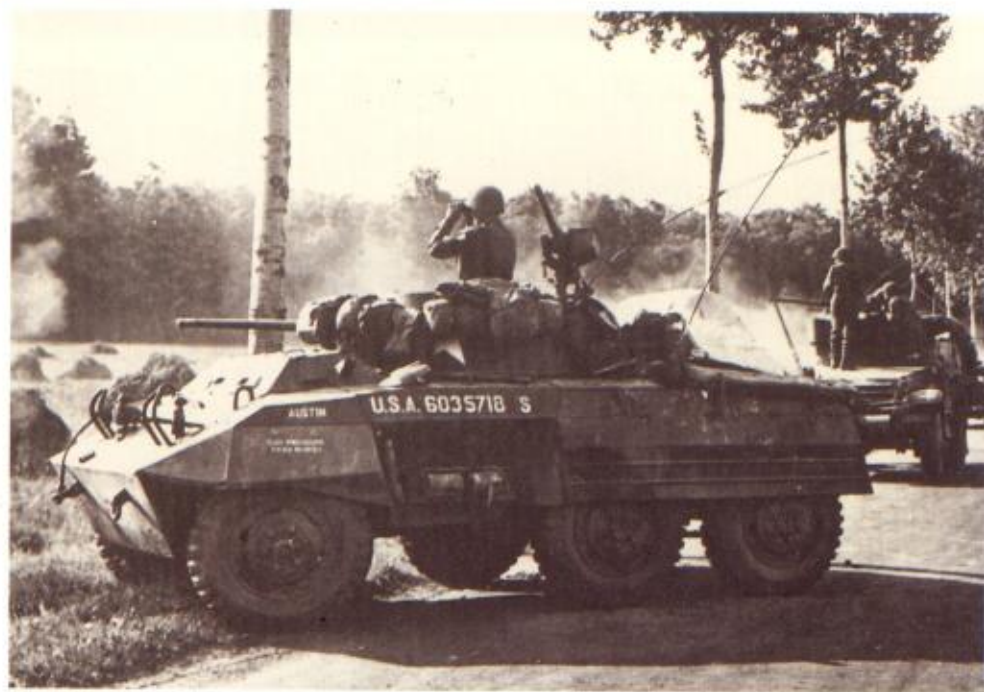
Below: The M8 Greyhound was the only armoured car to be used by the US Army in large numbers. Over 8,500 were built by the Ford Motor Company. (TM/Roland Groom)
