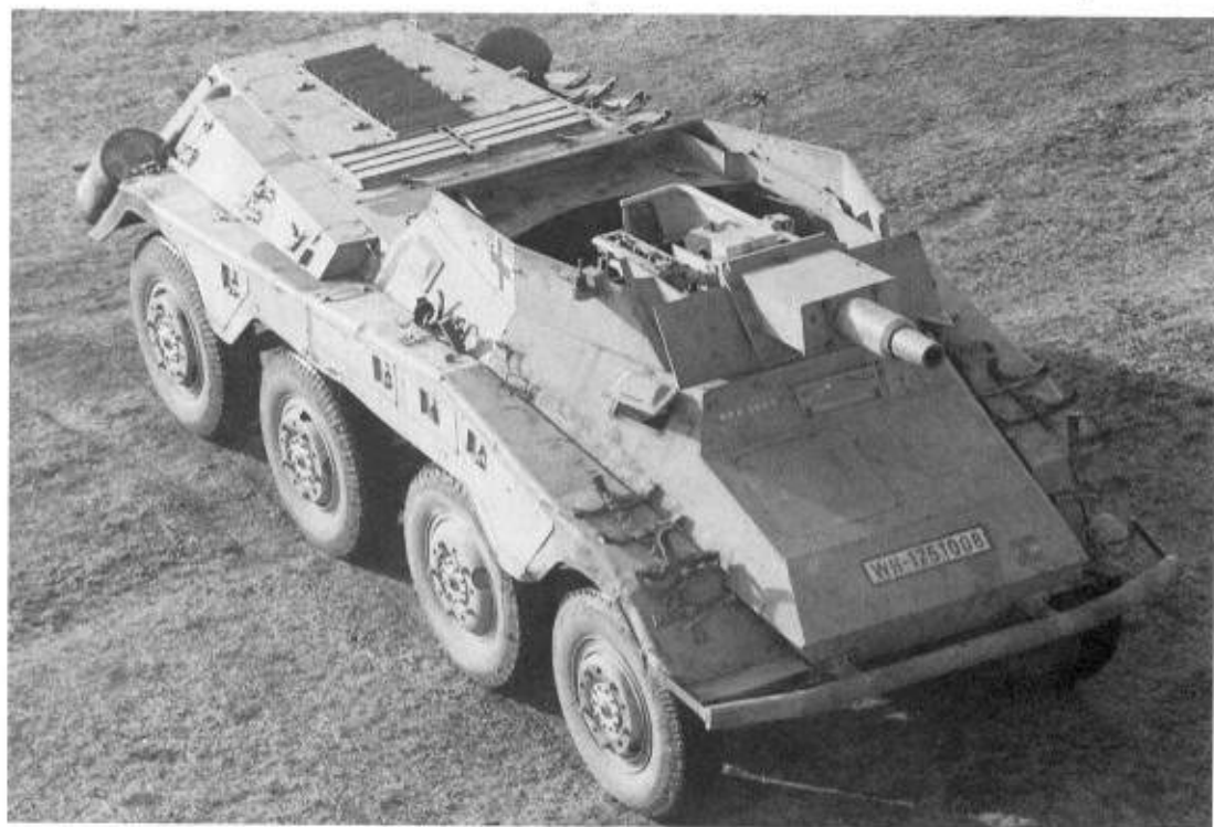
Left: The SdKfz 234/3 8rad mounted the short-barrellled 7.5cm KwK 51 L/24 gun – under ninety were built. (TM)
