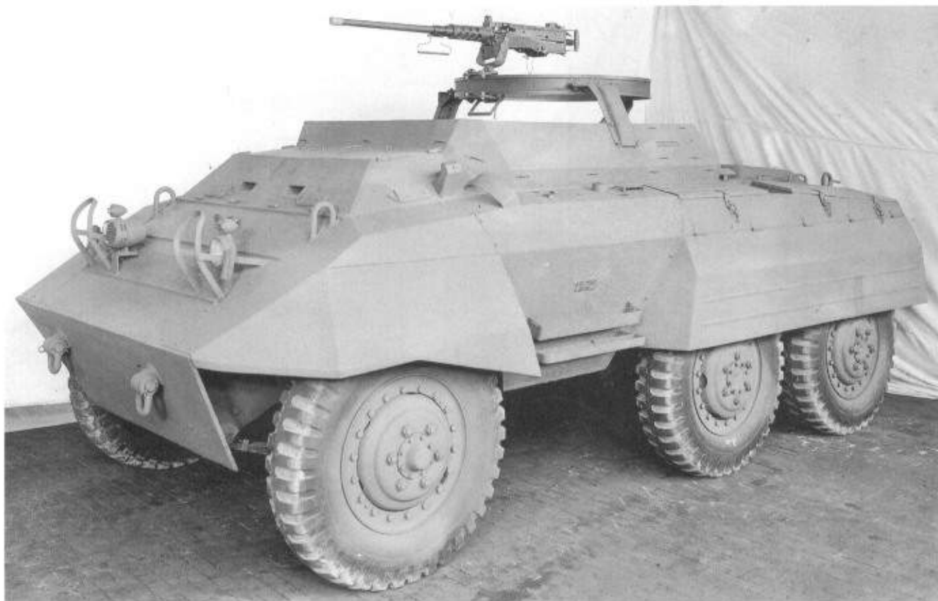
Above: The M20 armored utility car, of which nearly 4,000 were built by Ford. A versatile machine with a .50in heavy machine gun on a skate-ring mount. (TM)
