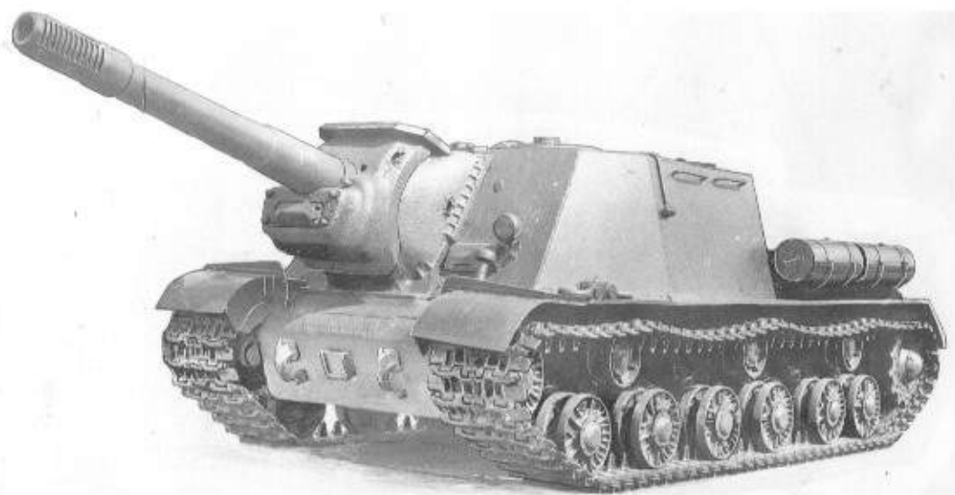
Left: The ISU-152 heavy self-propelled gun entered service in 1944, and provided long-range covering fire to support attacking formations. It was normally used in the direct fire role. (TM)
