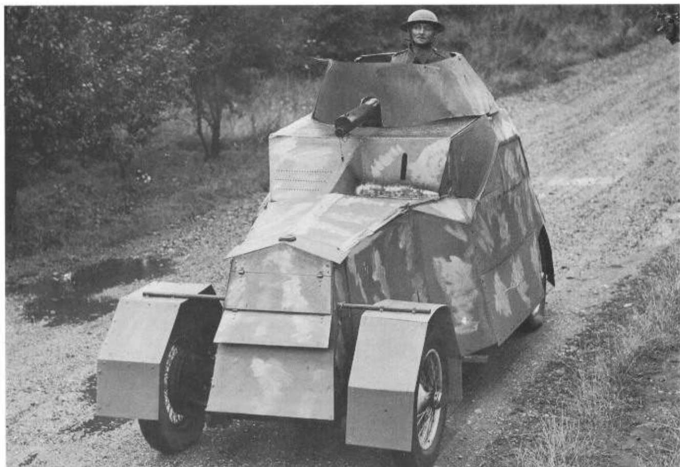
Above: The 'Tickler Tank', built using a Sunbeam car chassis by the Tickler Factory of Maidenhead, England and manned by the Home Guard. July 1940. (TM)
