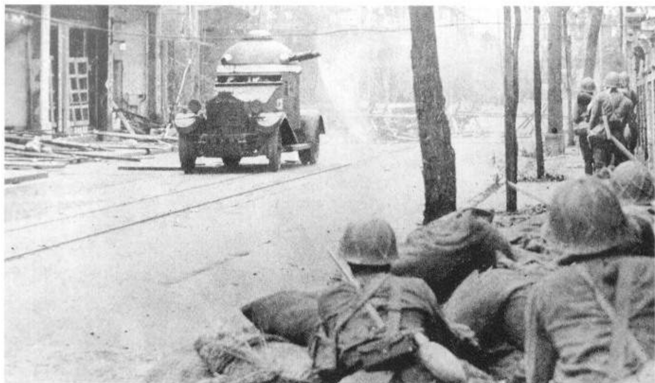
Above: An ex-British Indian pattern Vickers-Crossley, known as the Type 2587 (or Type 87), drives down a street in war-torn China watched by Japanese infantrymen. (TM)
