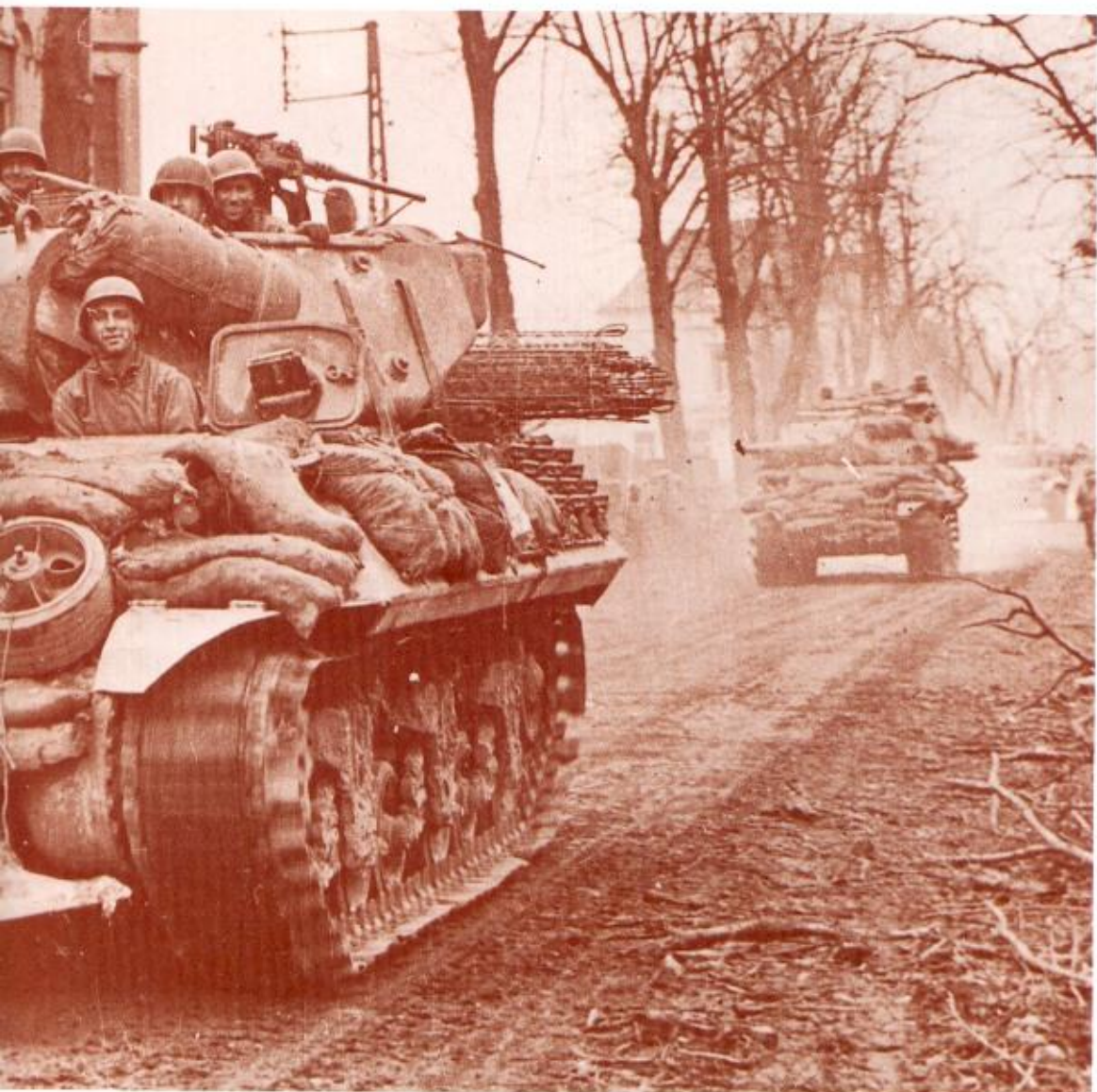
Below: M10s were sometimes used to provide artillery support, especially when there were shortages of conventional artillery. The 3-inch gun had a maximum range in excess of 14,500metres and fifty-four rounds were carried on the vehicle. (TM)
