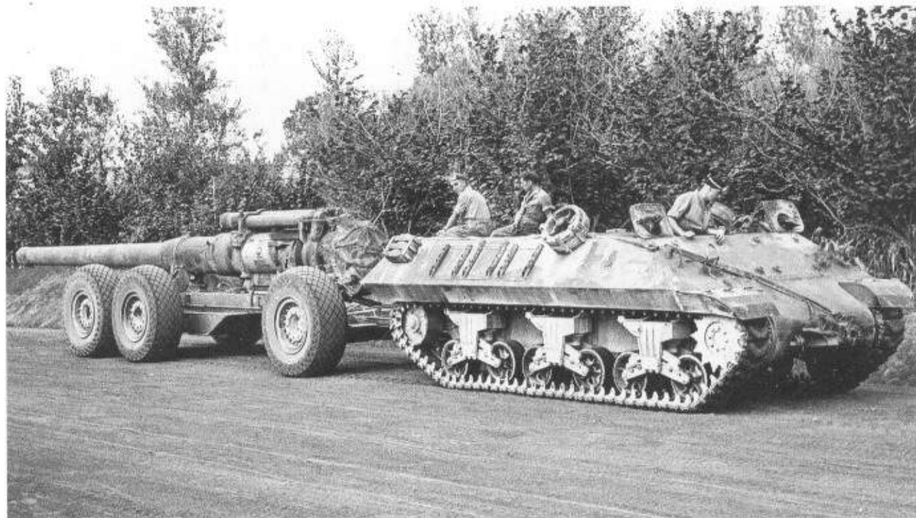
Below: M 35 Gun Tractor, towing a 155mm gun, was based on the M4A2 Sherman chassis. (TM)
