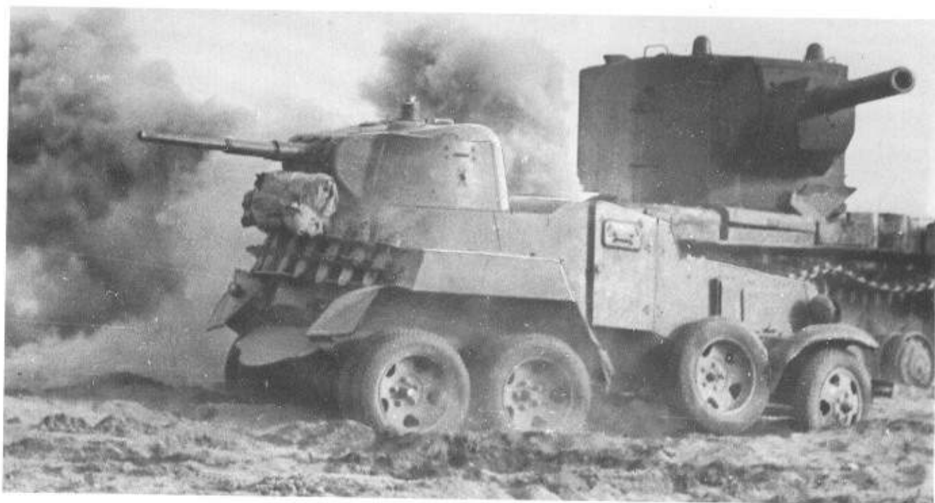
Above Amid the smoke of battle, a six-wheeled BA-10 heavy armoured car, with its turret traversed to the rear, drives in front of a massive KV 2 heavy tank. The spare wheel on the side of the BA-10 is almost grounded. (TM)
