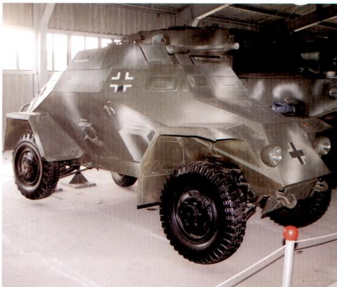
Left & Below: Two views of the SdKfz 222 leichter Panzerspähwagen. Without the anti-grenade cover fitted, the main armament 2cm KwK 30 or 38 L/550 which was mounted along with a co-ax MG34, is seen clearly. (RJ Fleming)
