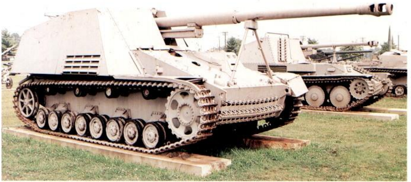
Above: Mounting a lethal 8.8cm PaK43/1 (L/71) anti-tank gun on the same chassis as the Hummel , the Nashorn/Hornisse (Rhino/Hornet) first saw active service in Russia from 1943. It was later used in both Italy and Northeast Europe. (RJ Fleming)
