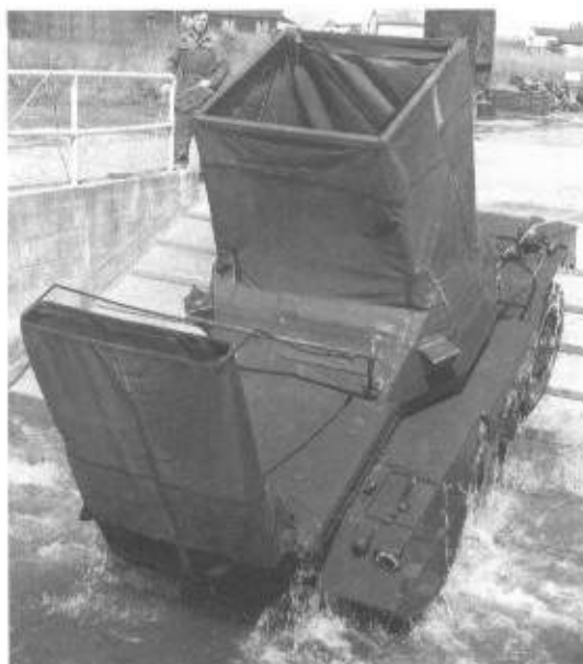
Left Daimler scout car fitted with full amphibious equipment to both engine and crew compartment. (TM)
