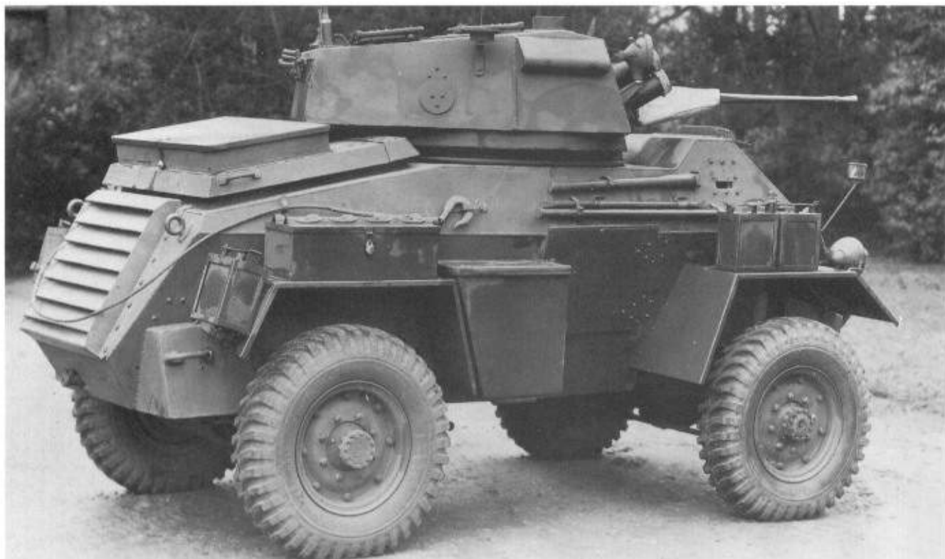
Above: The Humber Mk III still weighed about 7.2 tons, but had a larger turret, so could carry another crew member (four instead of three) (TM)
