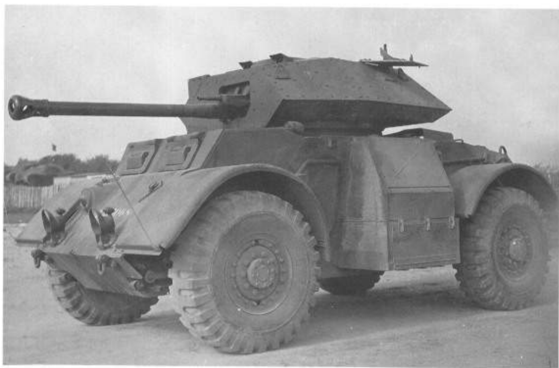
Left: Staghound fitted with a British Crusader tank turret, mounting a 75mm gun and co-ax BESA machine gun. (TM)
