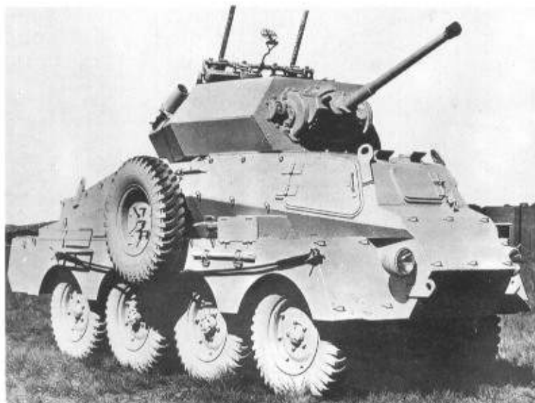
Above: The South African Armoured Reconnaissance Car MkVI (Marmon-Herrington armored car MkVI) mounted a 6 pounder instead of a 2 pounder gun. It was first ordered in mid-1942, but then cancelled. (TM)
