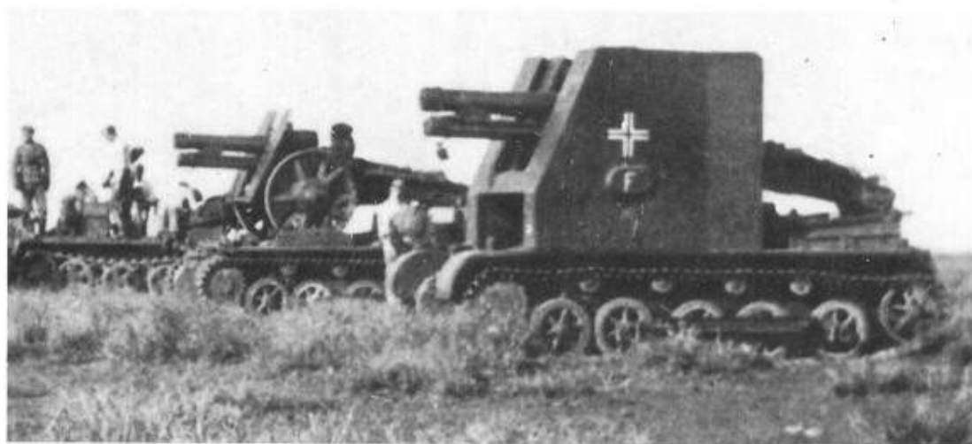
Above: The 10.5cm leFH18/1 L/28 auf Waffenträger GW IVb, was better known as the Heuschrecke (Grasshopper) 10. Only three prototypes of this tracked light field howitzer were built in 1943. (TM)
