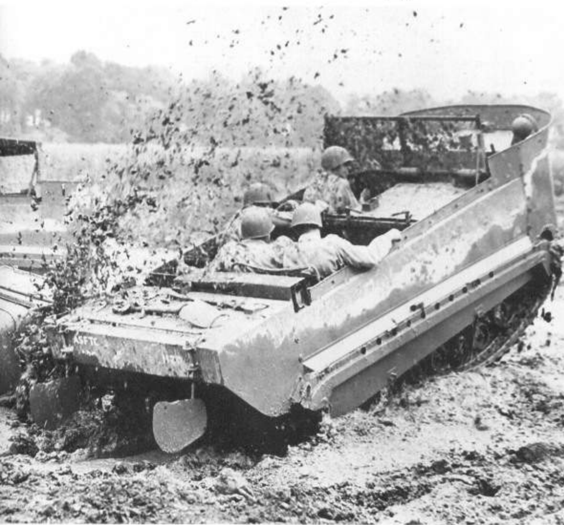
Left: A fully amphibious M29C Weasel, fitted with twin rudders and spray guard. (TM)
