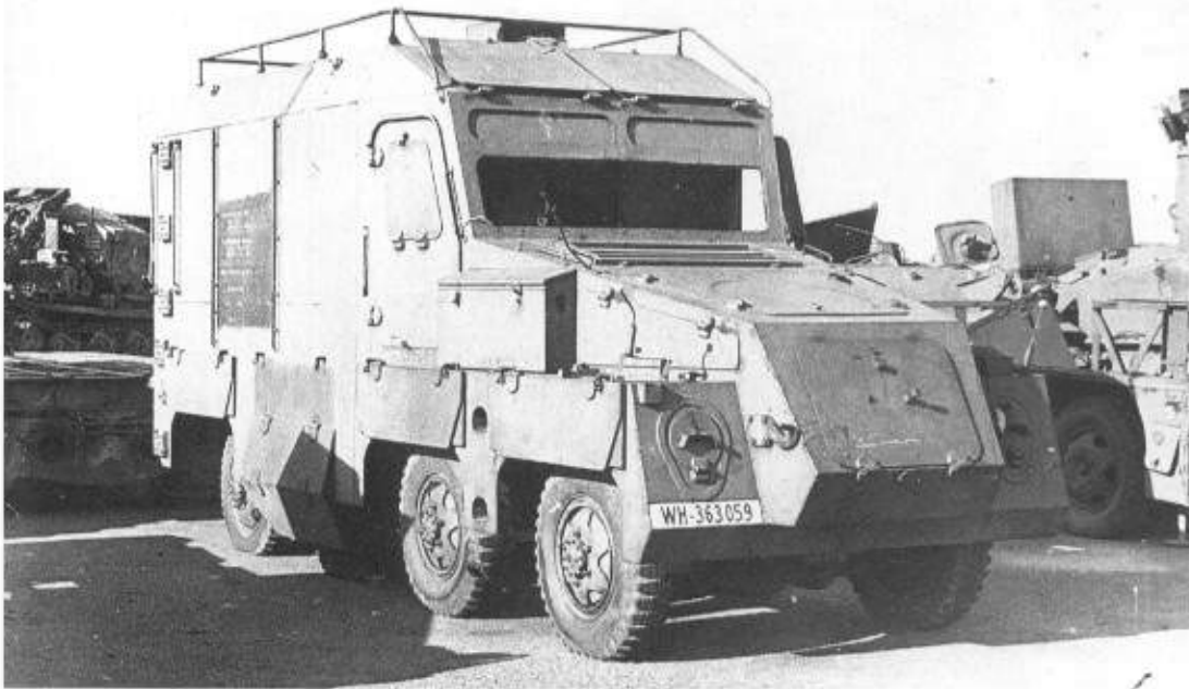
Above: An SdKfz 231 8rad, captured by the British. Main armament was one 2cm KwK30 and a co-ax MG34. (TM)
