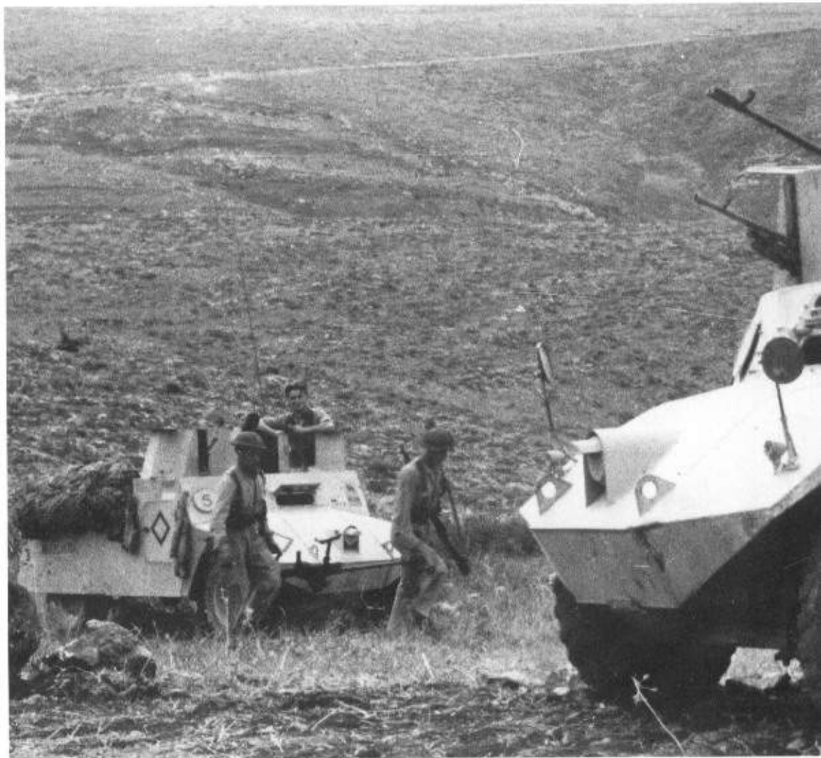
Below: Morris MkII light reconnaissance car, a 4x2 vehicle weighing 3.7 tons with a crew of three and a top speed of 50mph. Armament was a Bren LMG and a Boys anti-tank rifle. (TM)
