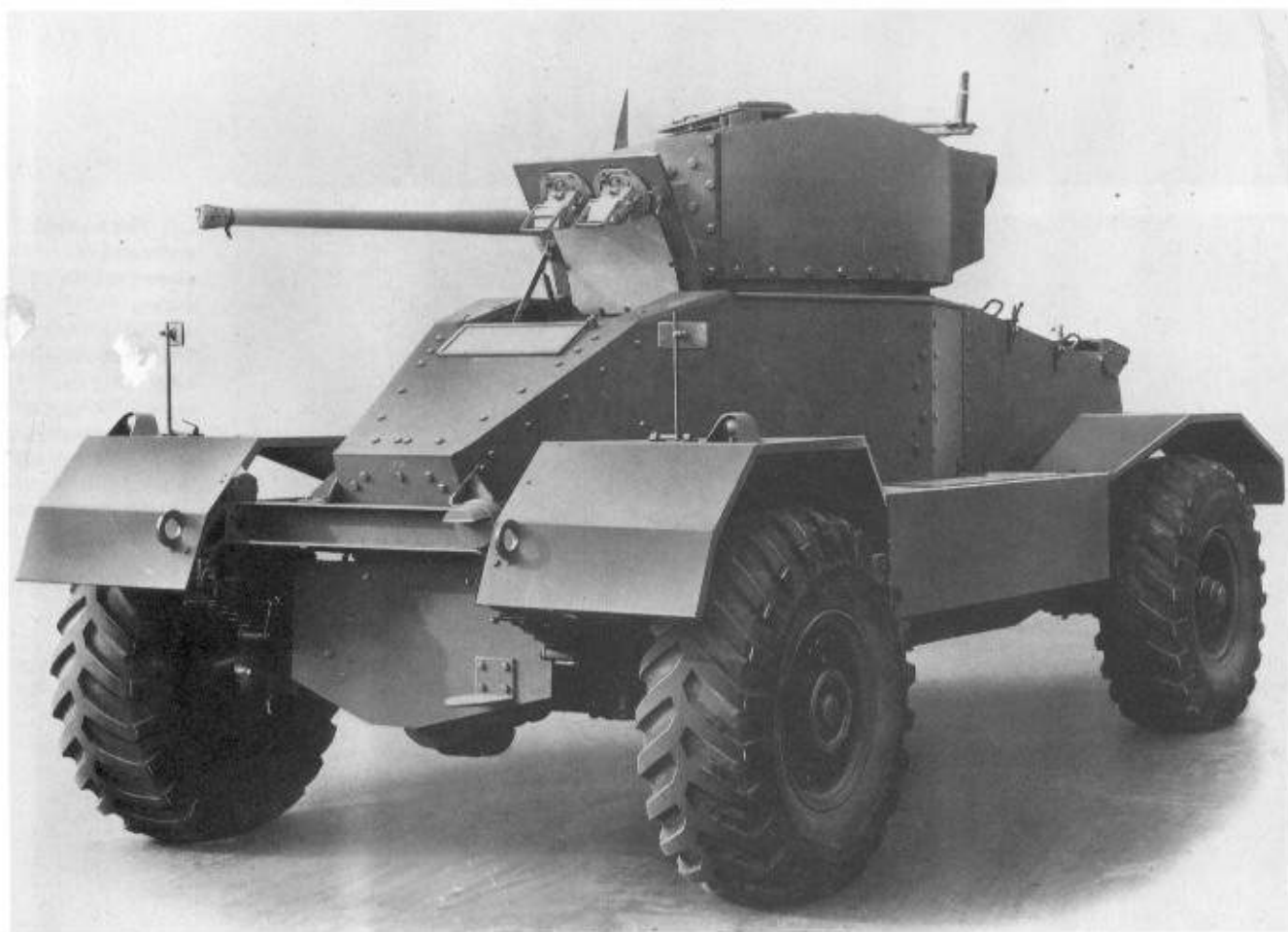
Below: An AEC Mkl heavy armoured car, which mounted a 2 pounder gun and co-ax BESA, in a two-man turret very similar to that of the early Valentine tank. (TM)
