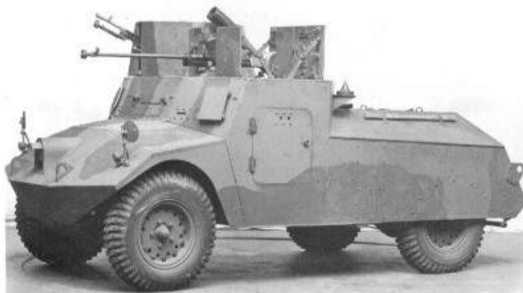
Below: Morris MkII light reconnaissance car, a 4x2 vehicle weighing 3.7 tons with a crew of three and a top speed of 50mph. Armament was a Bren LMG and a Boys anti-tank rifle. (TM)
