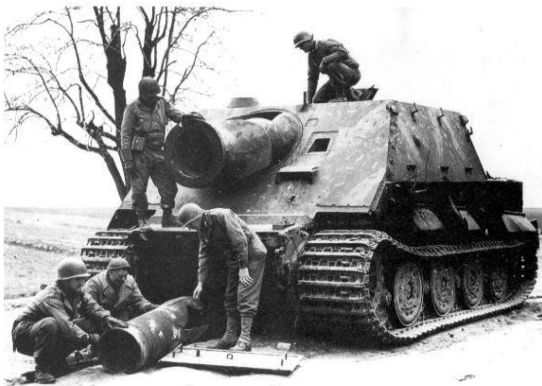
Left: The Tiger-Mörser mounted a massive 38cm mortar and weighed 65 tons. Only eighteen were ever converted from Tiger 1's during 1944. It fired rocket-assisted, mortar ammunition originally developed by Rheinmetall-Borsig for the German Navy to be used in anti-submarine warfare. (TM)
