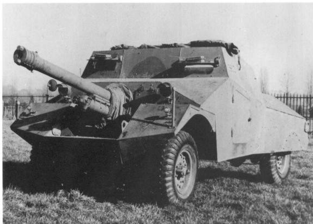
Left: This Morris light reconnaissance car has been turned into a formidable vehicle, by mounting a 6 pounder gun, but there is no evidence that it was ever used in battle. (TM)
