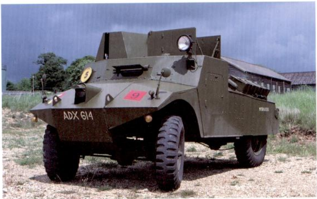
Right & far right: Front and rear views of the Morris Light Reconnaissance Car Mk II, which was armed with a Bren gun and a Boys anti-tank rifle. Over 3,600 of all Marks were built. (TM/Roland Groom)
