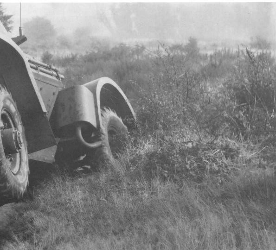
Left: A newly-built Daimler Mk1 armoured car, on trials at the Daimler Car Company, negotiating difficult terrain. (TM)
