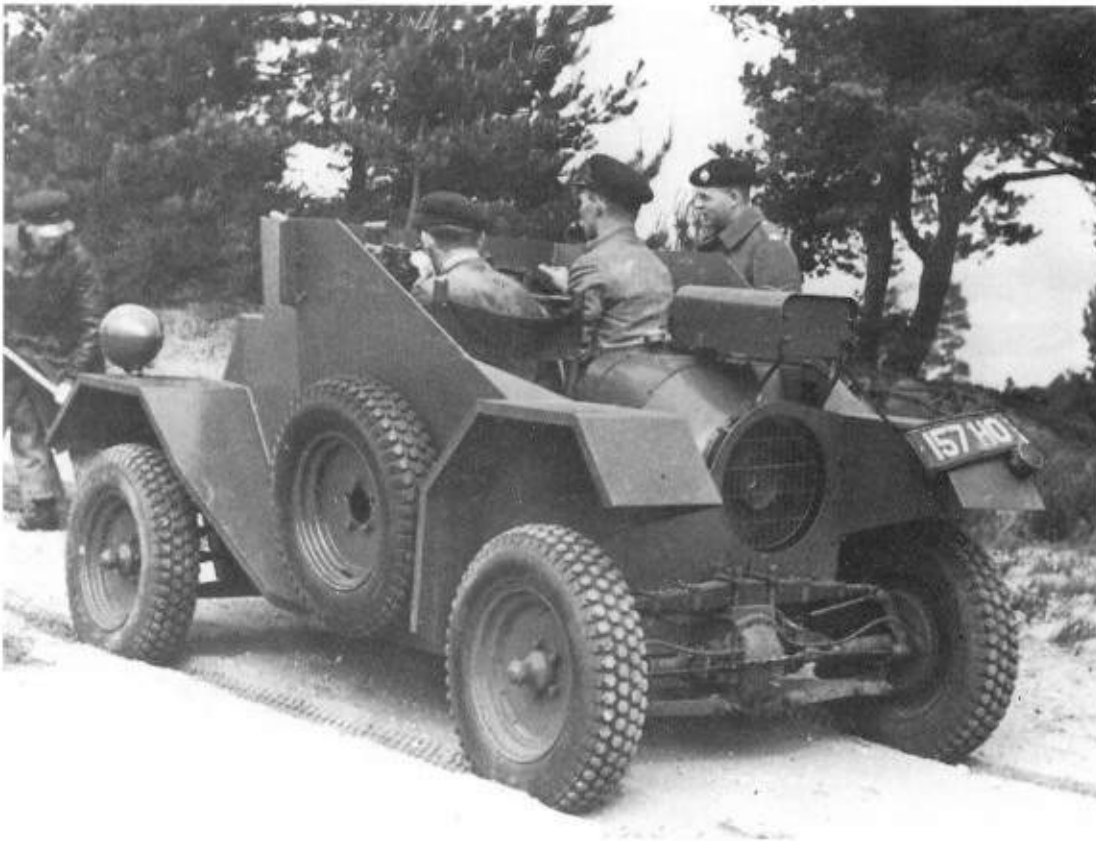
Left: The BSA, which was the other contender for the scout car project. It weighed 1120lbs more than the Alvis model and had marginally inferior performance, however, it was cheaper and had a lower centre of gravity. It was chosen for production, with a re-designed hull and roof. (TM)
