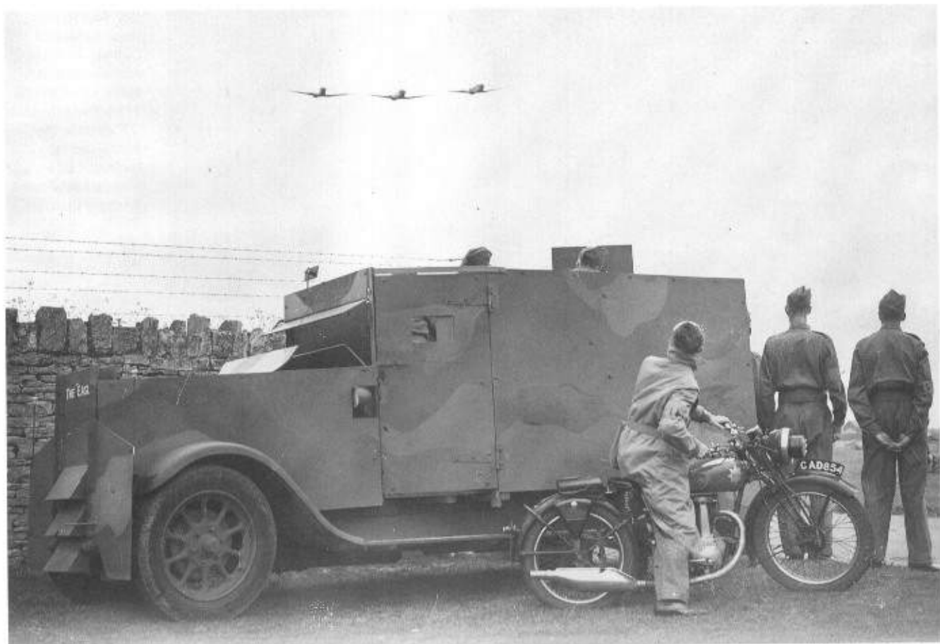
Above: One of many improvised armoured cars constructed in Britain during the dark days of 1940. 'EAGLE' was built by the Stroud Home Guard, Gloucestershire - they adapted three civilian cars into two well-armoured cars and an ambulance. (TM)
