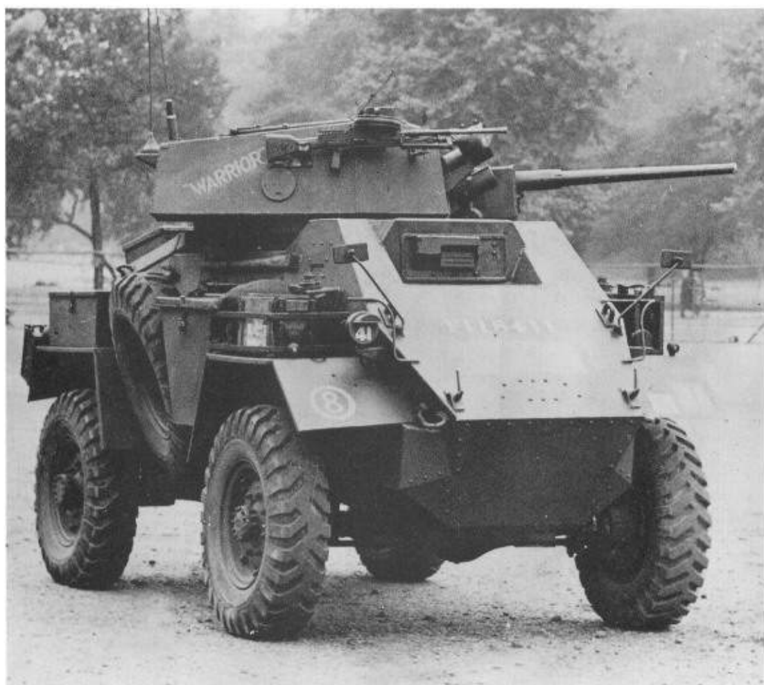
Above: The Humber Mk III still weighed about 7.2 tons, but had a larger turret, so could carry another crew member (four instead of three) (TM)
