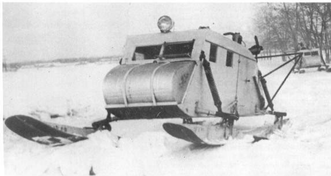
Right: The NKL-16/41 Aerosan could be fitted with a machine gun for raiding, but was mainly used for transporting men or stores. (TM)
