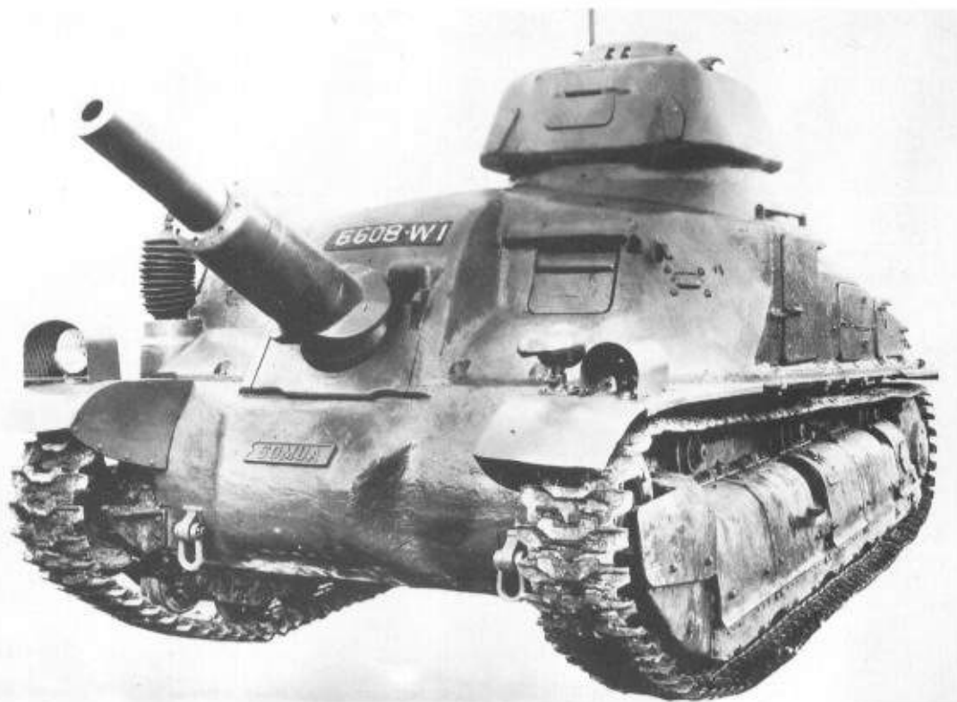
Right: The Somua SAU 40 mounted a 75mm gun in the front of a cast hull, with a Char B turret offset to the left. (TM)
