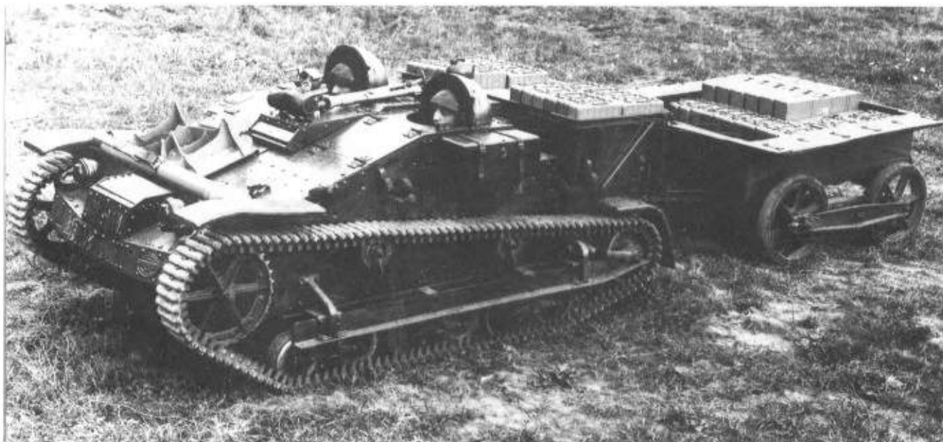
Above: The diminutive 2-ton Renault Chenillette was used for a wide variety of tasks. Much of its design was derived from the British Carden-Loyd. (TM)
