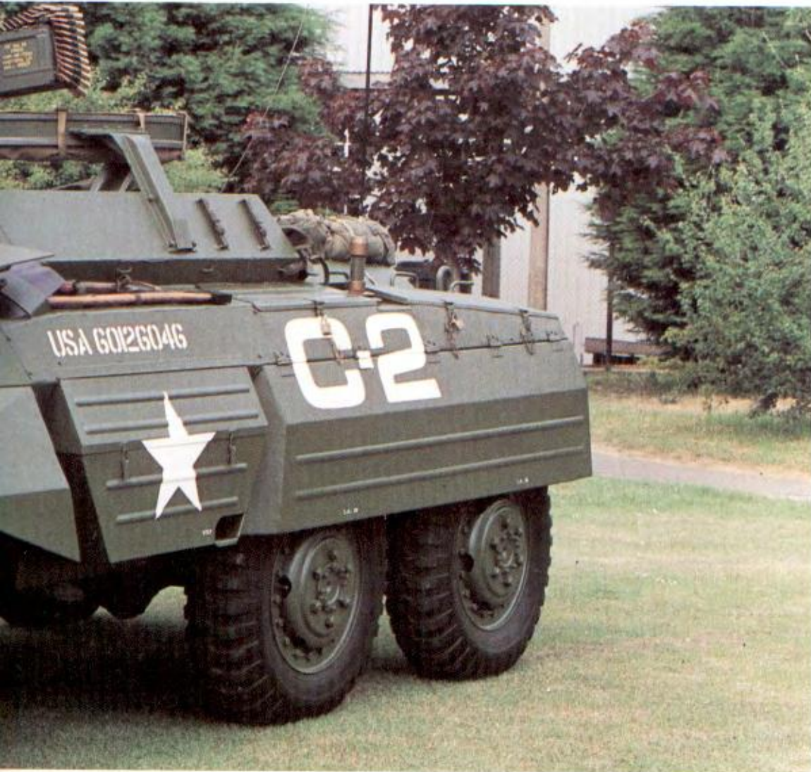
Below centre: The only remaining T16E2 Boarhound armoured car in Great Britain is at the Tank Museum. It was a massive 26.8 ton vehicle, armed with a 57mm gun.
