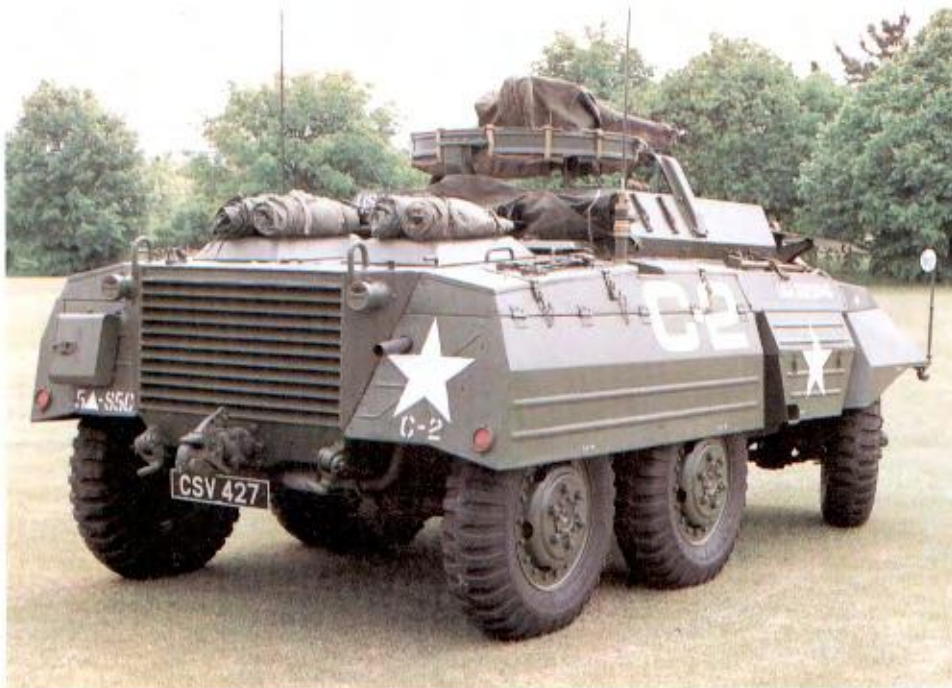
Below: The M20 was a turretless M8 Greyhound, armed with a ring-mounted .50in Browning heavy machine gun. (TM/Roland Groom)
