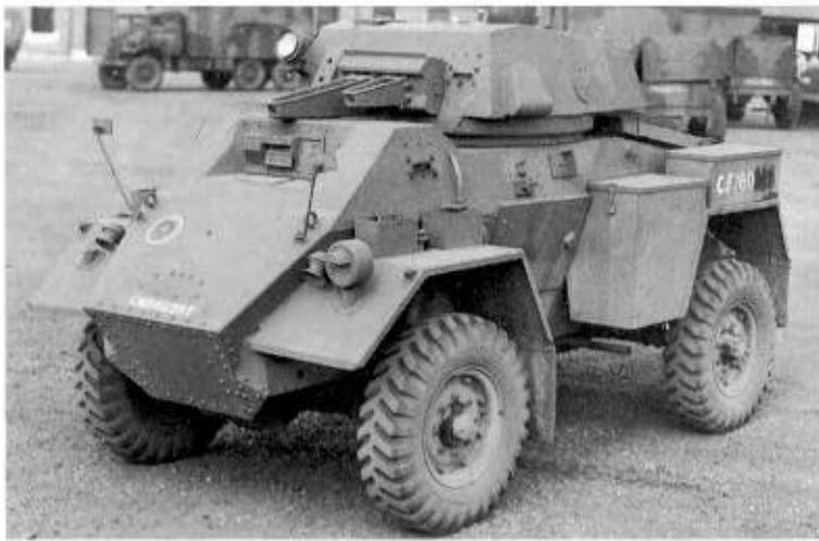
Above: A General Motors of Canada Mkl Fox armoured car, without its armament fitted (.50 and .30in Browning MGs). (TM)
