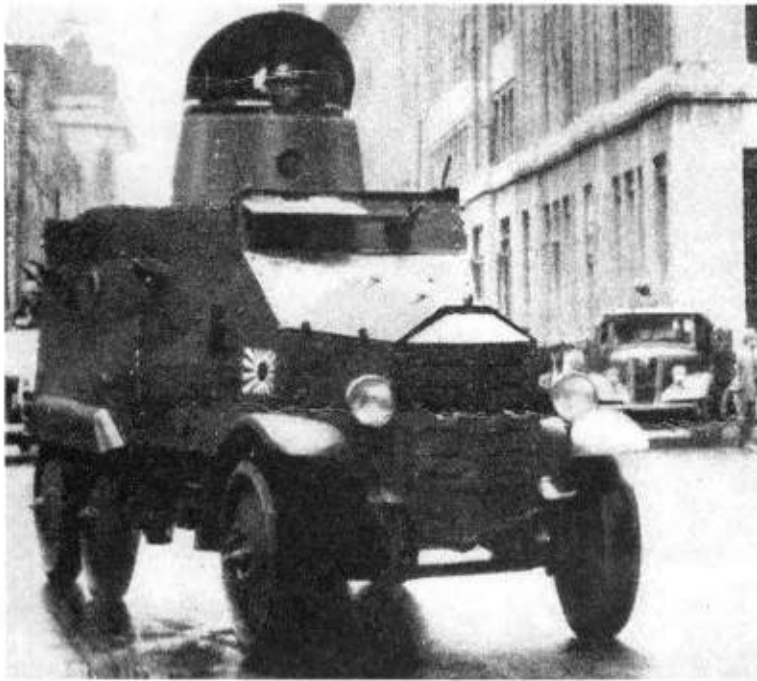
Top: A well-camouflaged naval pattern Type 2592 (or Type 92), built in 1932 it weighed 6.2 tons and had a crew of six. Note the anti-grounding wheels behind the front wheels. (TM)
