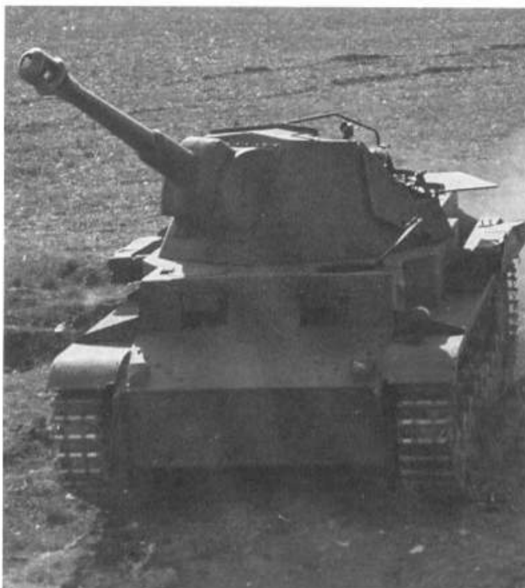
Above: The 10.5cm leFH18/1 L/28 auf Waffenträger GW IVb, was better known as the Heuschrecke (Grasshopper) 10. Only three prototypes of this tracked light howitzer were built in 1943. (TM)
