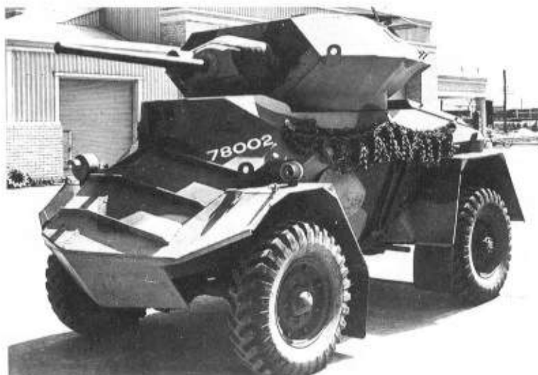
Top: The Australian-built 4x4 scout car had a crew of two. The body had vertical sides and a sharply sloping rear deck. (TM)
