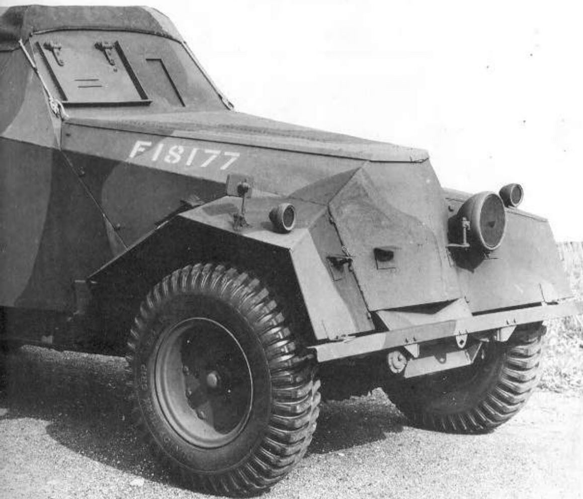
Left: Humber MkI, Ironside I light reconnaissance car, built on the Humber Super Snipe car chassis. Three were specially modified for use by the Royal family. (TM)
