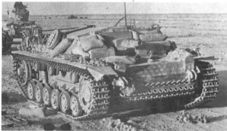
Above: The Stug III Ausf C/D did not have the gunner's direct vision port and improved armour. (TM)
