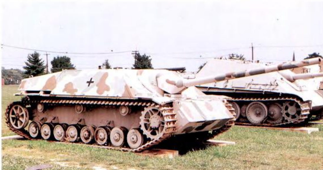
Right: Based on the PzKpfw IV chassis the SdKfz 167, Sturmgeschütz IV mounted a 7.5cm StuK40 L/48 anti-tank gun. (R.J Fleming)
