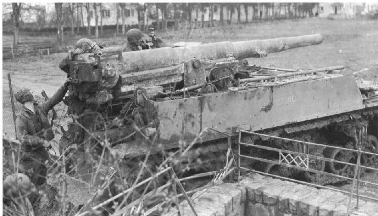
Above: A 155 mm M12 GMC being prepared for action in Belgium, 1944. The Cargo variant, to supply the M12 GMC, had the 155 mm gun removed to make space for ammunition. (TM)
