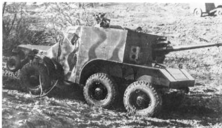
Below: This version of the Laffly S15 had a 47mm gun mounted at the rear with gun shield and an armoured body. (TM)
