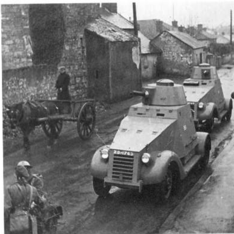
Above: Two Ford Mk VI armoured cars move through a village in Eire, March 1942. Armed with a single Vickers .303in MG, the 14ft 10ins long car had a top speed of 40 mph. (TM)
