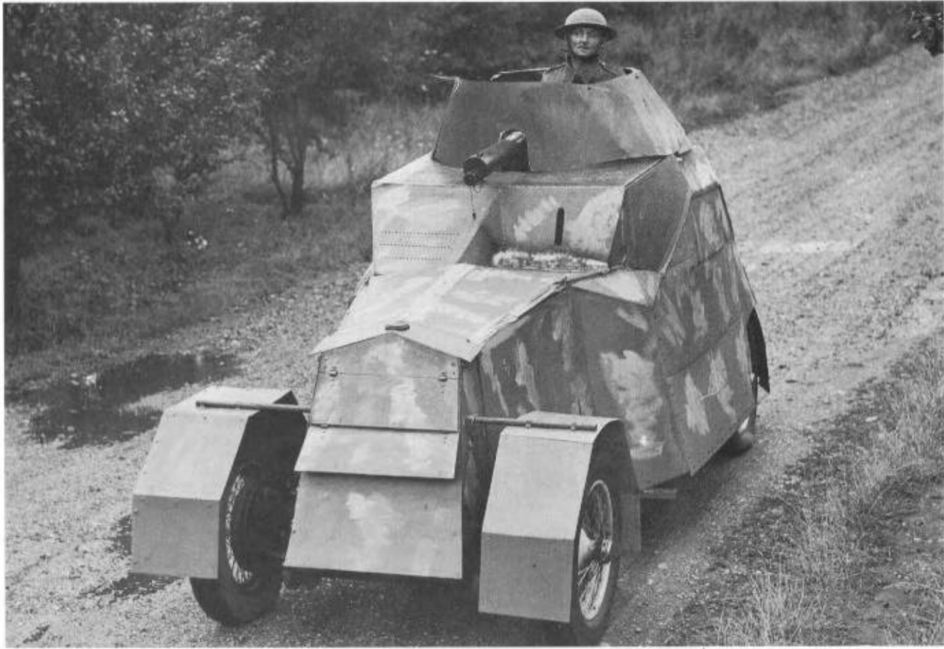
Above: The 'Tickler Tank', built using a Sunbeam car chassis by the Tickler Factory of Maidenhead, England and manned by the Home Guard. July 1940. (TM)
