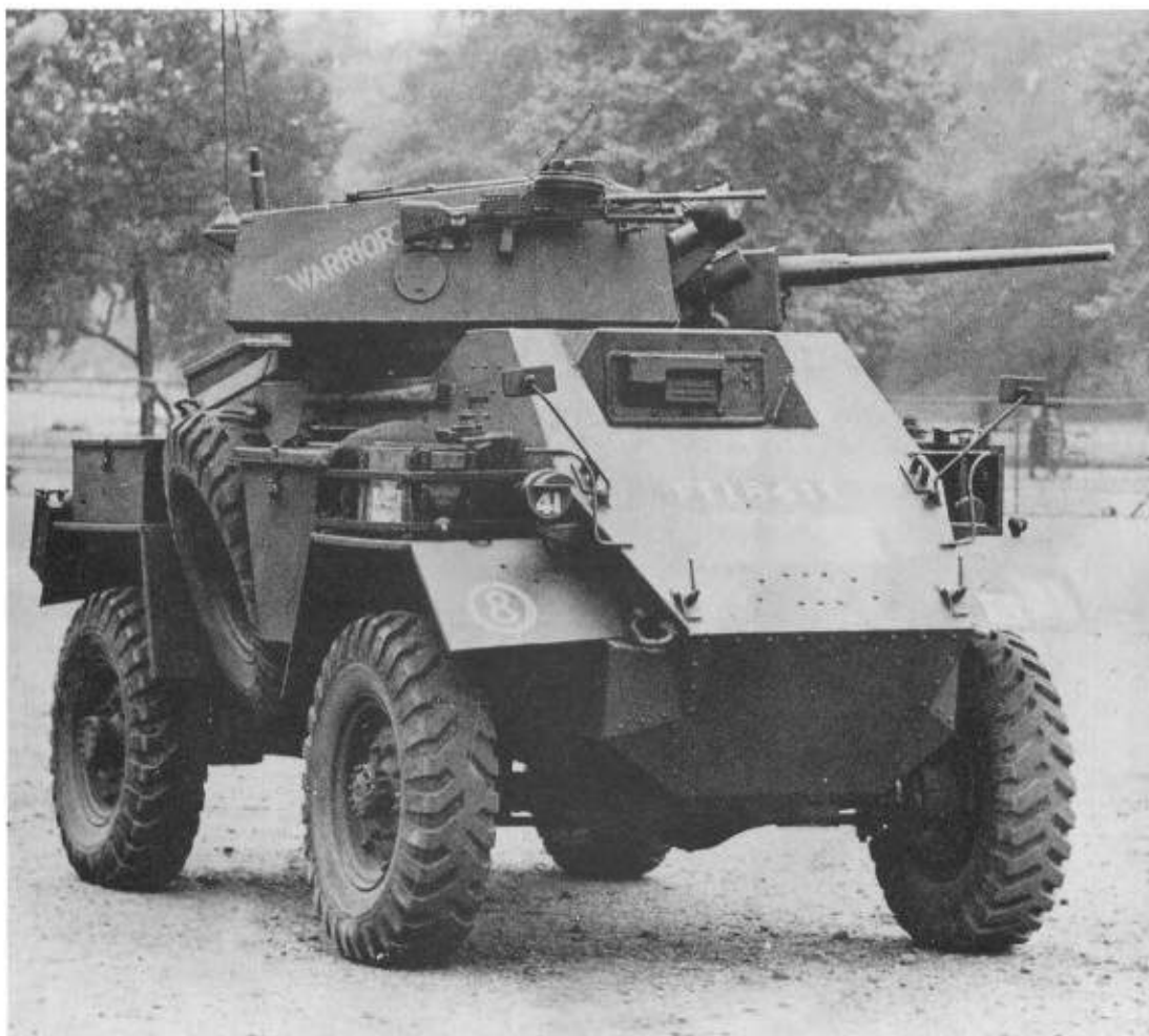
Above: The Humber MkIII still weighed about 7.2 tons, but had a larger turret, so could carry another crew member (four instead of three) (TM)
