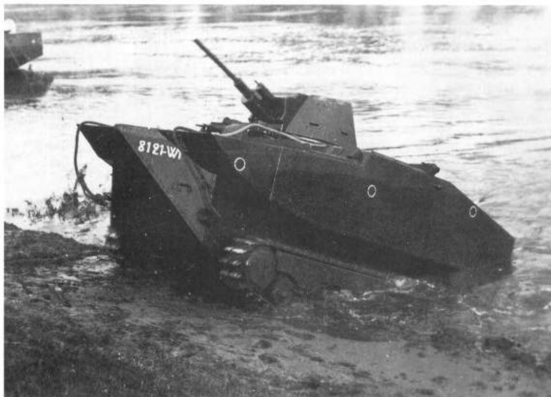
Left: An Automitrailleuse Amphibie DP2 (ARL Batignolles) pilot model amphibious tank. It never progressed further than the experimental stage after the pilot model sank in 1935. (TM)
