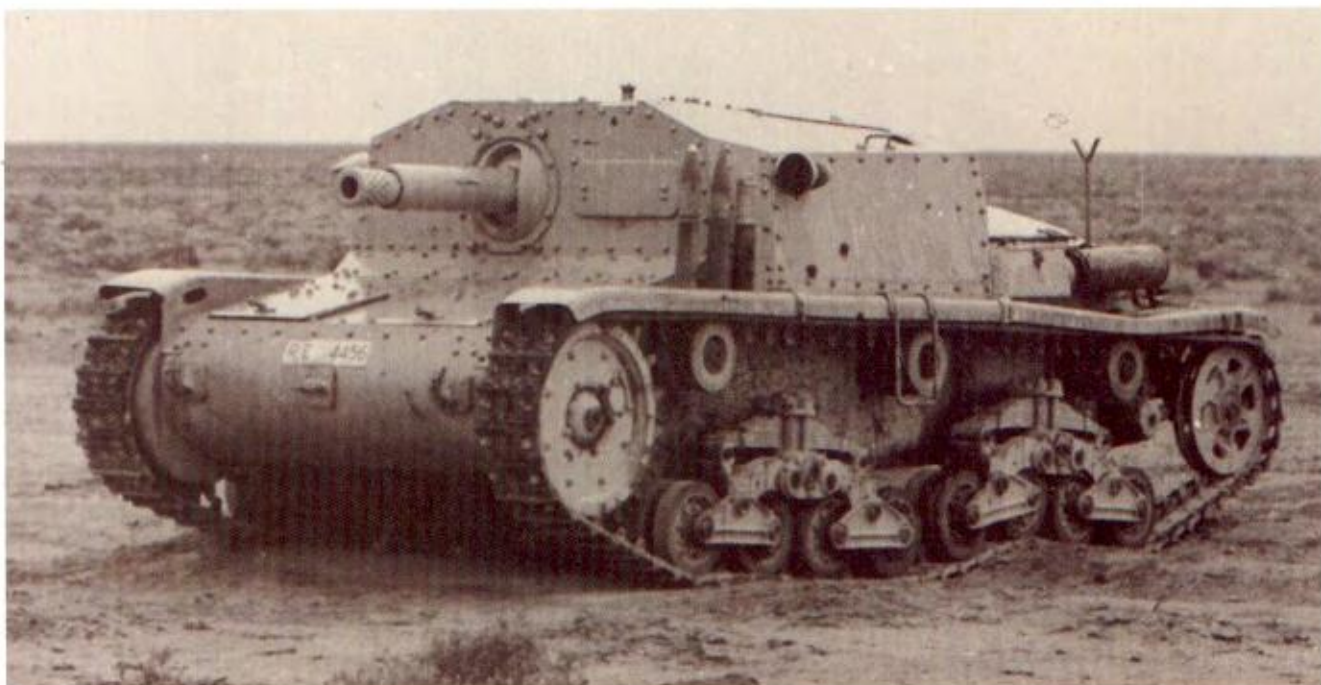
Below: Another captured Semovente 75/40 da M41, clearly shows the simple, box-like superstructure. (TM)
