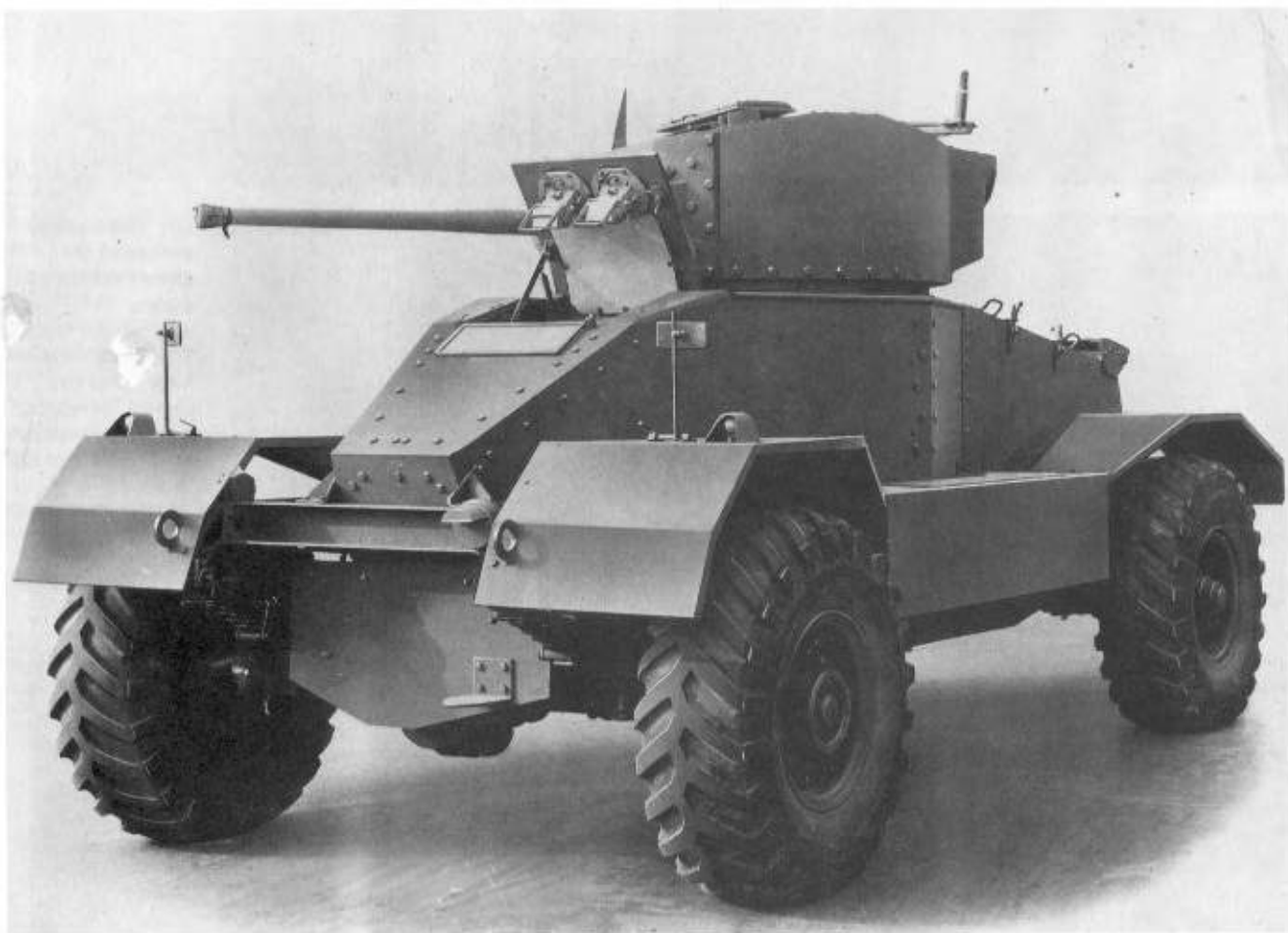
Below: An AEC Mki heavy armoured car, which mounted a 2 pounder gun and co-ax BESA, in a two-man turret very similar to that of the early Valentine tank. (TM)
