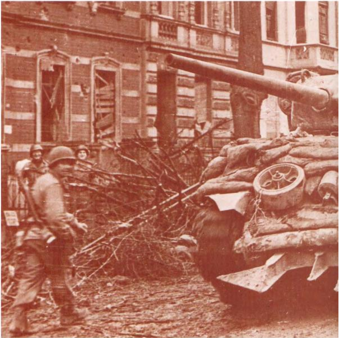
Right: The GMC M10 tank destroyer, mounted an M7 gun, was also known as the Wolverine. This one, in service with the US First Army is seen passing through the damaged town of Duren, Germany in February 1945. It is still fitted with a Culin hedgerow cutter which had proved invaluable in the bocage countryside of Normandy. (TM)
