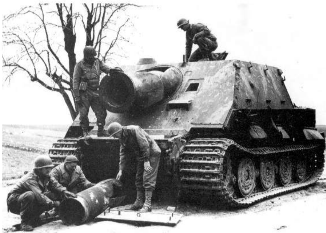
Left: The Tiger-Mörser mounted a massive 38cm mortar and weighed 65 tons. Only eighteen were ever converted from Tiger 1's during 1944. It fired rocket-assisted, mortar ammunition originally developed by Rheinmetall-Borsig for the German Navy to be used in anti-submarine warfare. (TMA)
