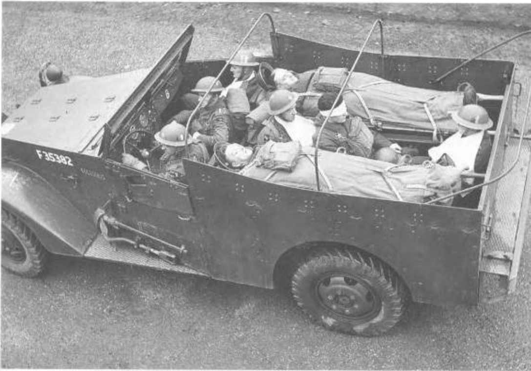
Left: The M3A1 was a versatile vehicle, seen here being used as an ambulance for carrying both stretcher cases and walking wounded. (TM)
