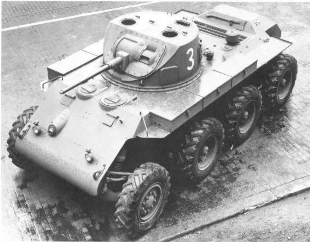
Left: Reo built three prototypes of the T13 in 1941 all mounting the same 37mm gun and a co-ax MG. (TM)
