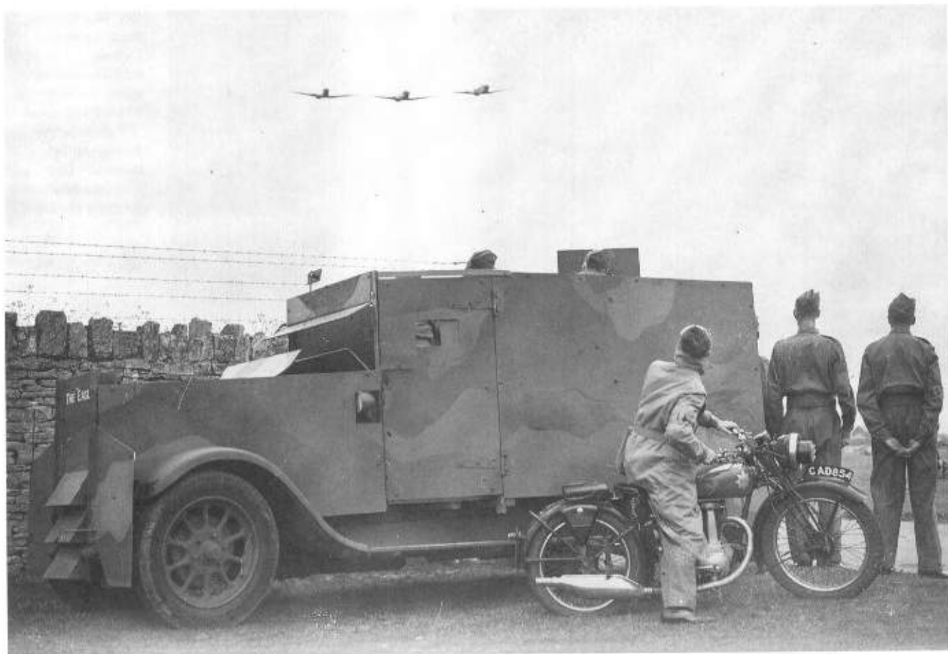
Above: One of many improvised armoured cars constructed in Britain during the dark days of 1940. 'EAGLE' was built by the Stroud Home Guard, Gloucestershire - they adapted three civilian cars into two well-armoured cars and an ambulance. (TM)
