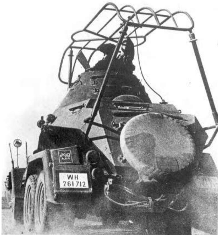
Above: The SdKfz 232 6rad (Fu) was the radio version of the six-wheeled SdKfz 231. Note the distinctive frame-type aerial. (TM)
