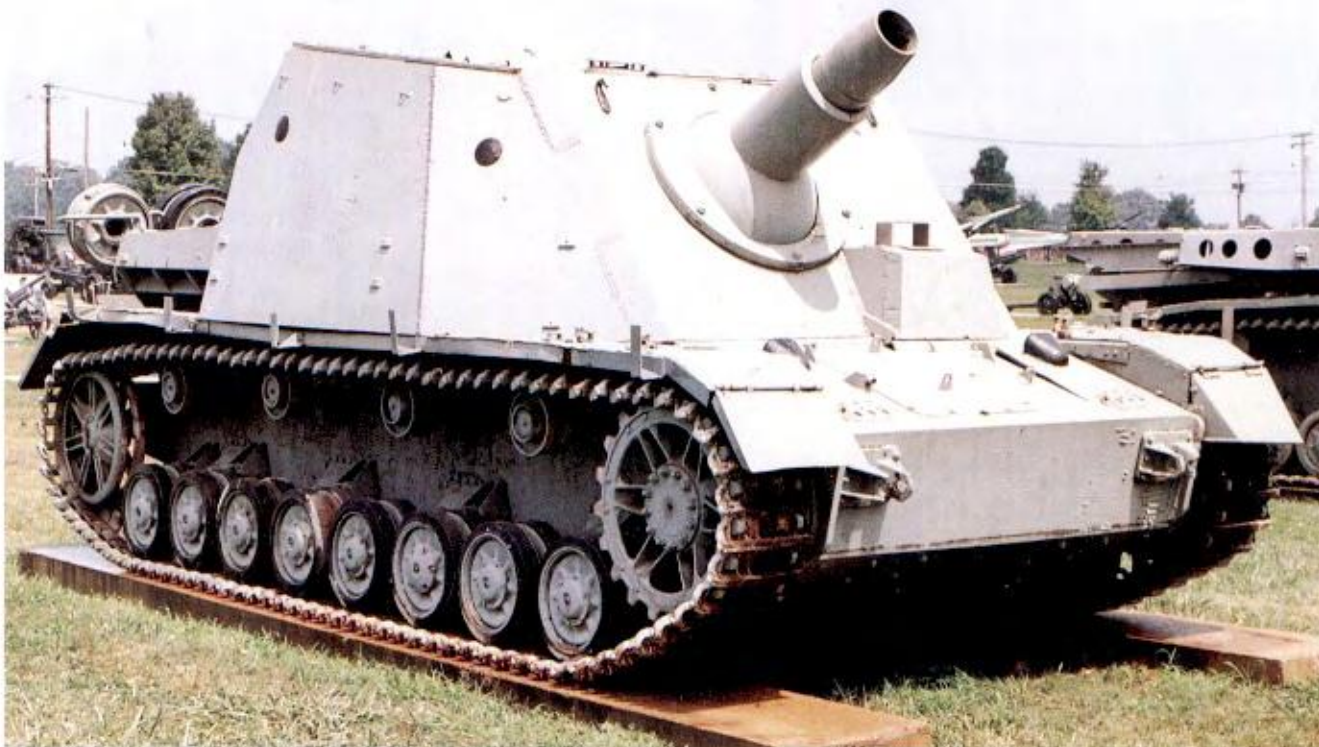
Above: SdKfz 166 Sturmpanzer IV, Brummbär (Grizzly Bear). Nearly 300 of these infantry assault guns were produced and all mounted a 15cm StuH43 L/12 on a standard PzKpfw IV chassis. (RJ Fleming)
