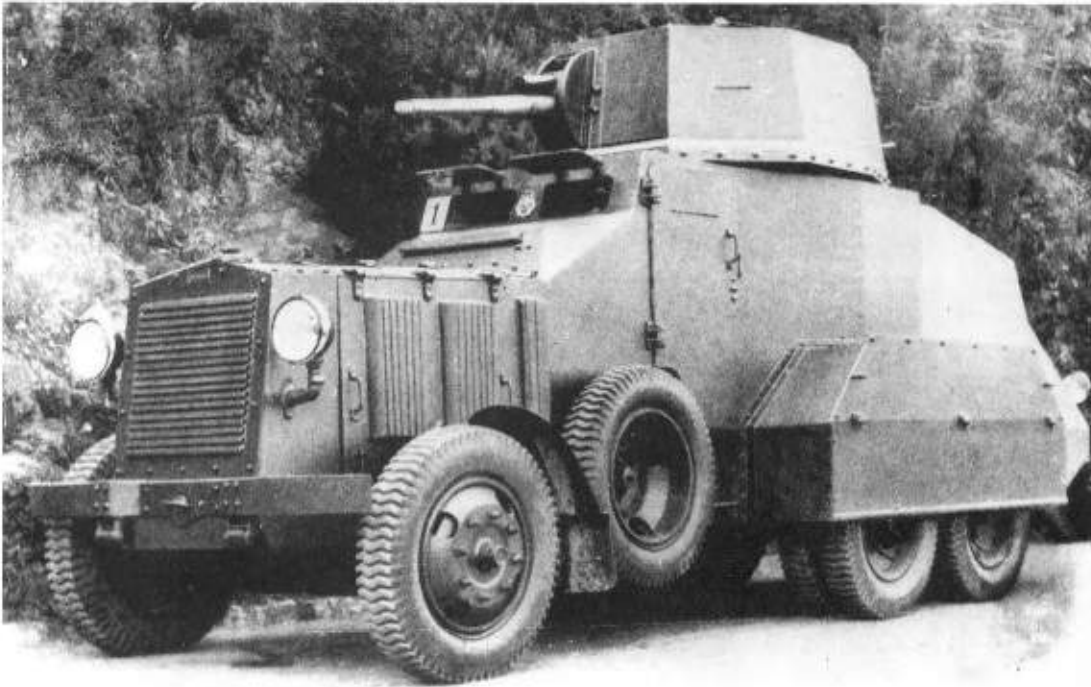
Left: The Fiat 611B, which dated from 1934, mounted a 47mm gun in a seven-sided turret and weighed some 7 tons. (TM)
