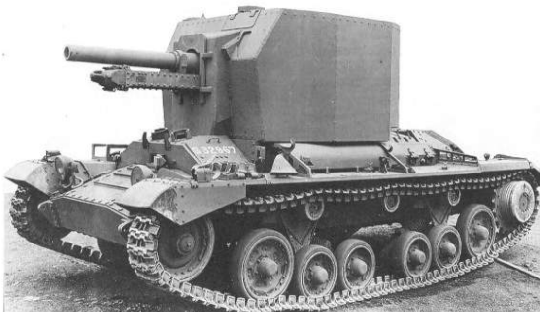
Left Bishop mounted a 25 pounder gun on a Valentine chassis, inside a box-like rigid armour structure, which did not allow full elevation of the gun. It was later replaced in service by Priest and was then only used for training purposes. (TM)
