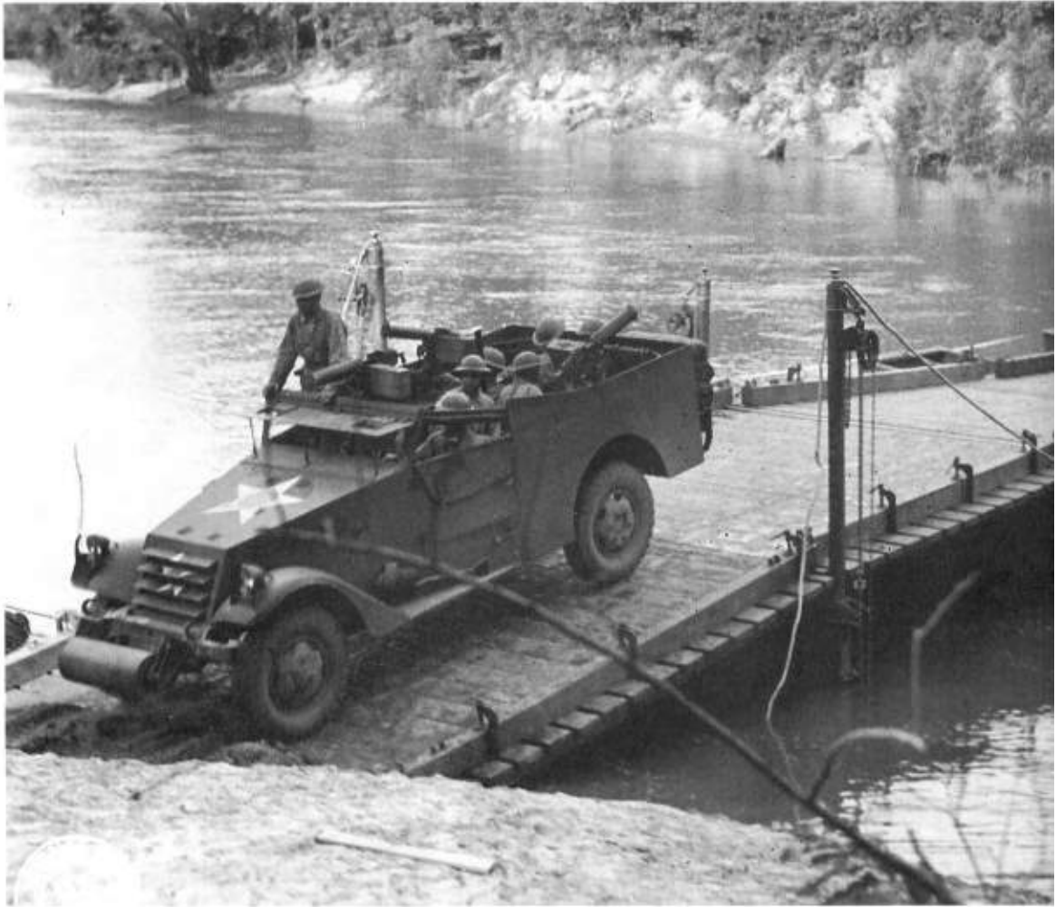
Below: M3A1 scout car fitted with the standard .50in Browning heavy MG at the front and a .30in at the rear, both on pintle mountings. (TM)
