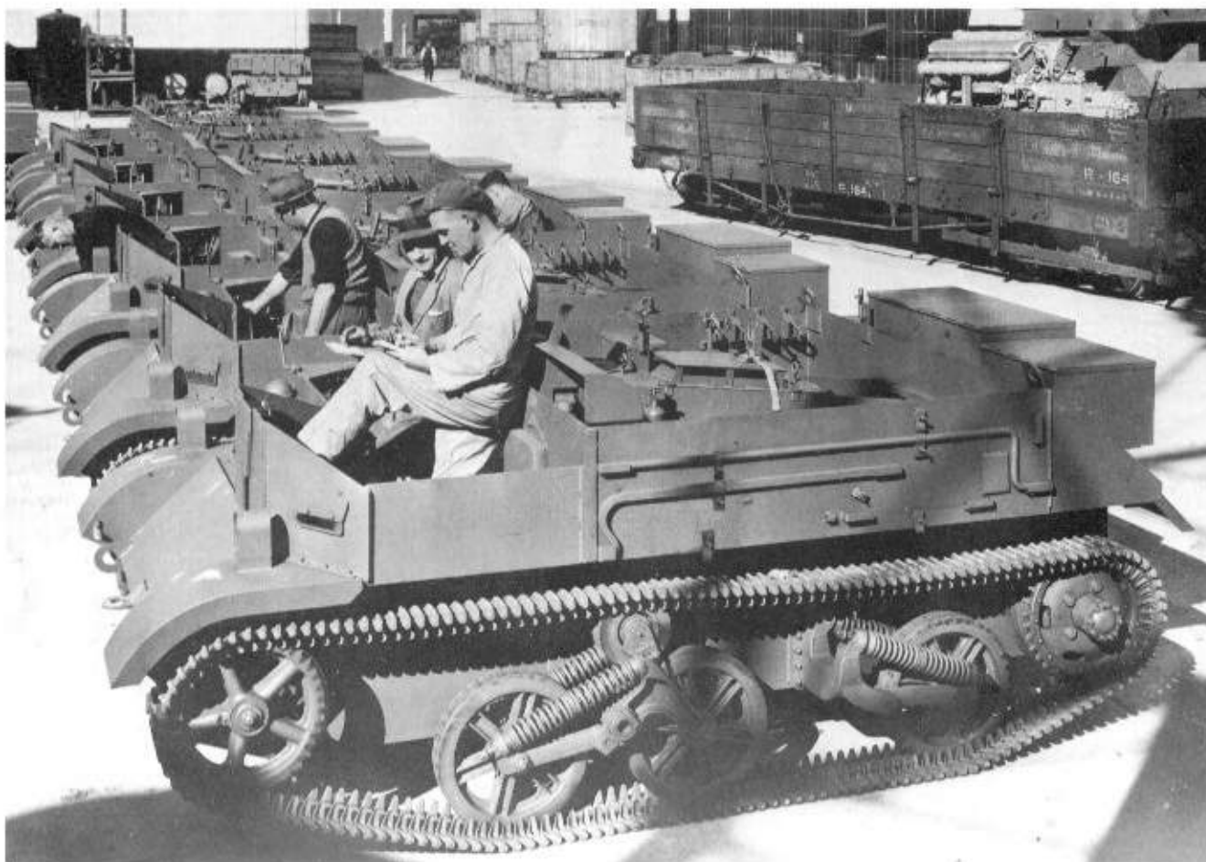
Above: A line up of New Zealand-built Universal Carriers, ready for despatch. They were initially produced using working drawings and machine tools provided from Australia. (TM)
