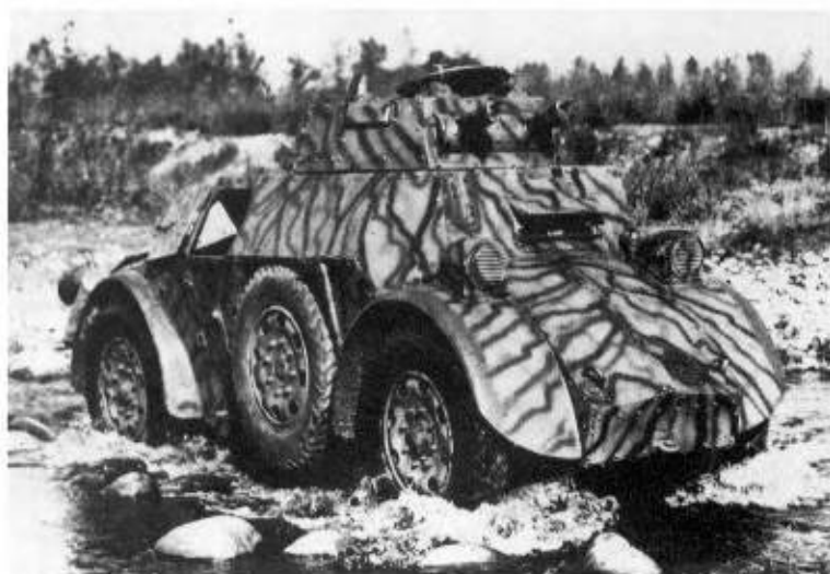
Below: Twin-machine guns in the turret was the major difference between the AB 40 and this AB 41. (TM)
