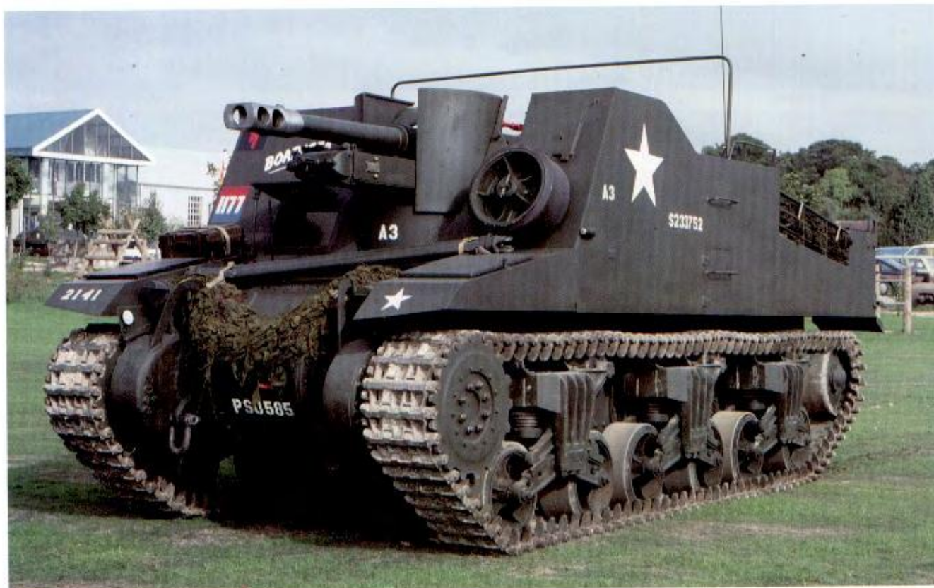
Below: A restored Sexton, the SP gun version of the Canadian-built Ram medium tank. (TM/Roland Groom)
