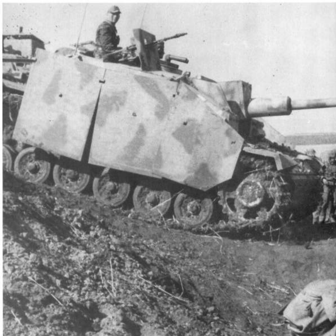
Right: Sturmgeschütz 40 Ausf G (also called the Stug III Ausf G) assault gun/tank destroyer negotiates a Soviet anti-tank ditch. The main armament was the 7.5cm StuK 40 L/48 gun. Note also the armoured shield on the machine gun by the loader's hatch and the peri-binoculars on the commander's cupola. (TM)
