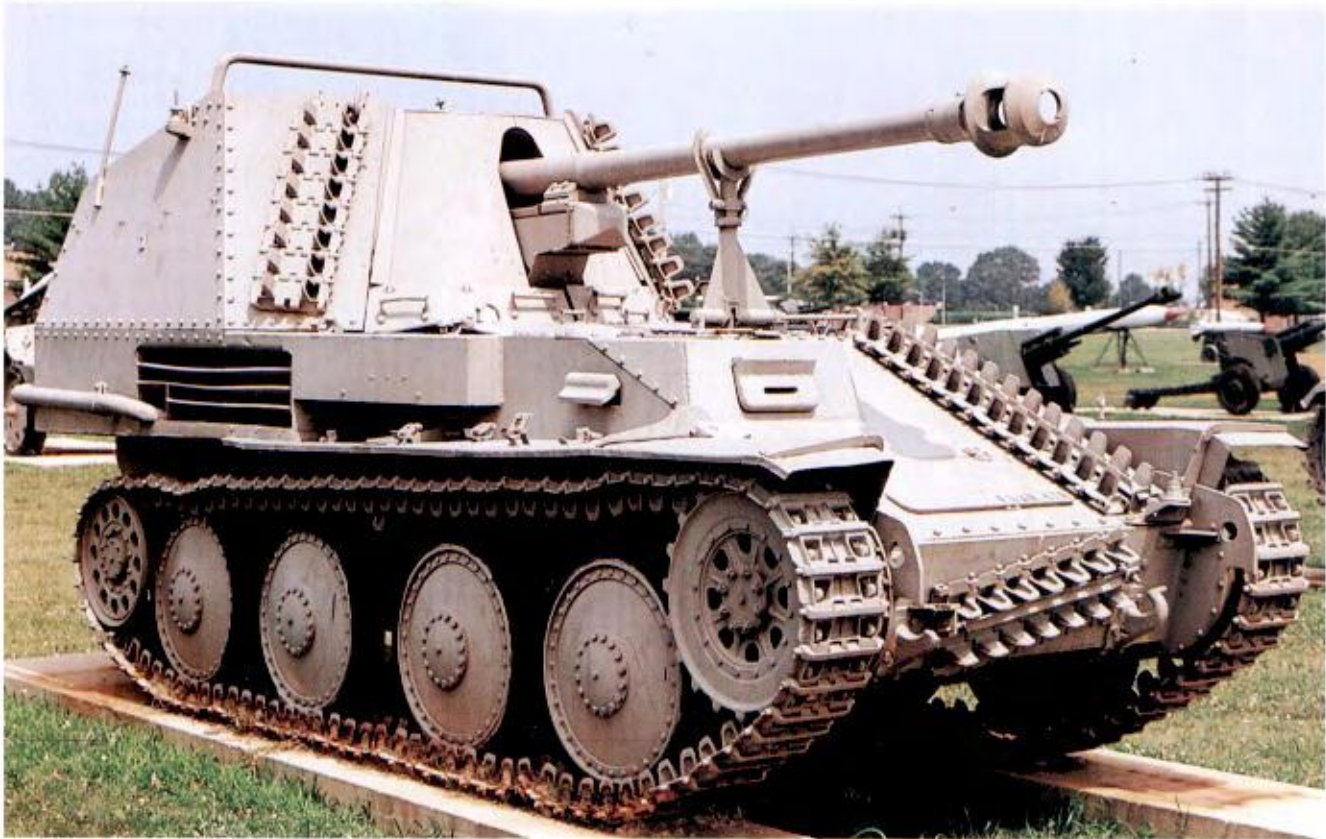
Above: SdKfz 139, Panzerjaeger 38(t) für 7.72cm PaK36(r), Marder III (Marten), mounted a Russian 7.62cm gun on an obsolete Czechoslovak tank chassis. (RJ Fleming)
