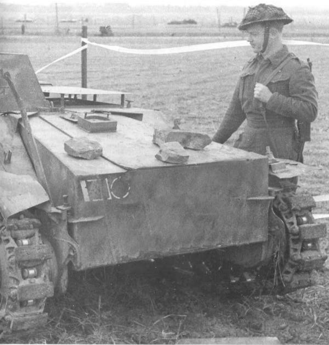
Left: SdKfz 301 schwerer Ladungsträger Ausf A/B was much larger than Goliath , weighing 3.6 tons. It was designed to be driven to a target where the demolition charge (on the front of the vehicle) could be dropped, the vehicle withdrawn and the charge remotely exploded. (TM)
