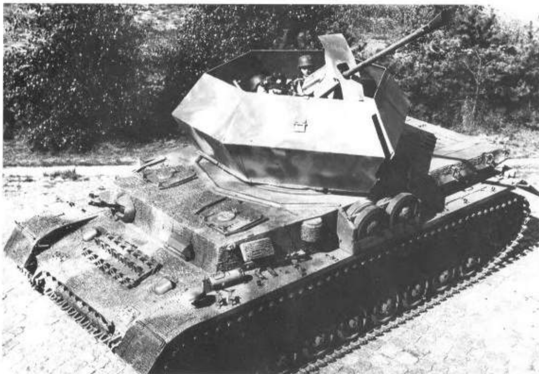
Left: Thirty-six PzKpfw IV were converted into FlaKpanzers. They mounted the 3.7cm FlaK 43/1 and was known as Ostwind (East Wind). (TM)
