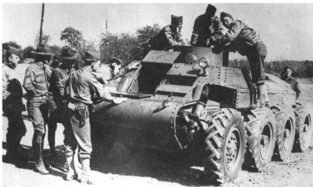
Above: The M20 armored utility car, of which nearly 4,000 were built by Ford. A versatile machine with a .50in heavy machine gun on a skate-ring mount. (TM)
