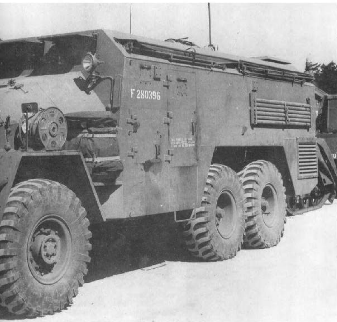
Left: An AEC 6x6 armoured command vehicle (ACV), which was larger and more powerful (150hp diesel engine) than the 4x4. As before there were HP and LP versions. (TM)
