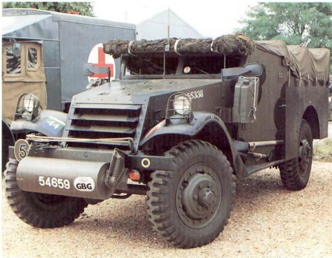
Left: A well restored White M3A1 scout car photographed at one of the Tank Museum's AFV rallies. Note the sprung roller front bumper. (TM/Roland Groom)
