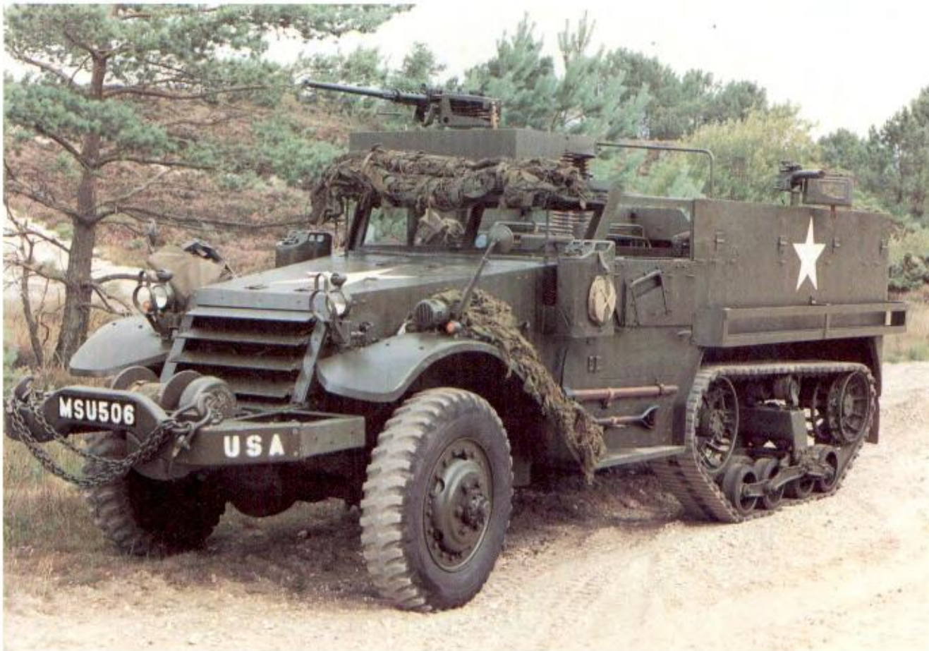
Below: On the Bovington Training Area during one of the RAC Centre's 'Battle Days' is this well equipped and restored White half-track, armed with both .50in and .30in Browning machine guns. (TM/Roland Groom)
