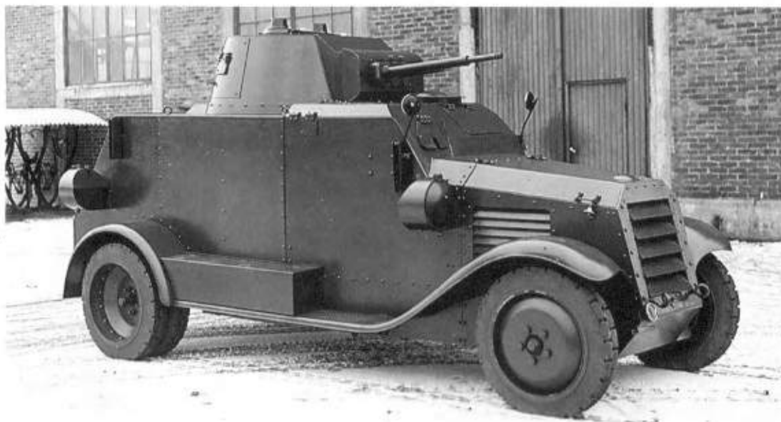
Top: The Swedish-built Landsverk 181 armoured car used a Scania Vabis 6x4 truck chassis and mounted a 20mm gun in conventional looking turret. (TM)
