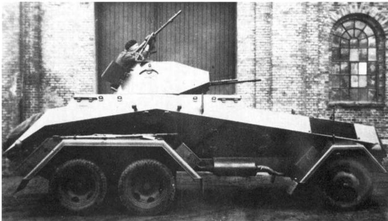
Above: The SdKfz 231 schwerer Panzerspähwagen 6 rad. This is an early prototype model, produced in 1932. The 231 was used on active service in Poland and France. (TM)
