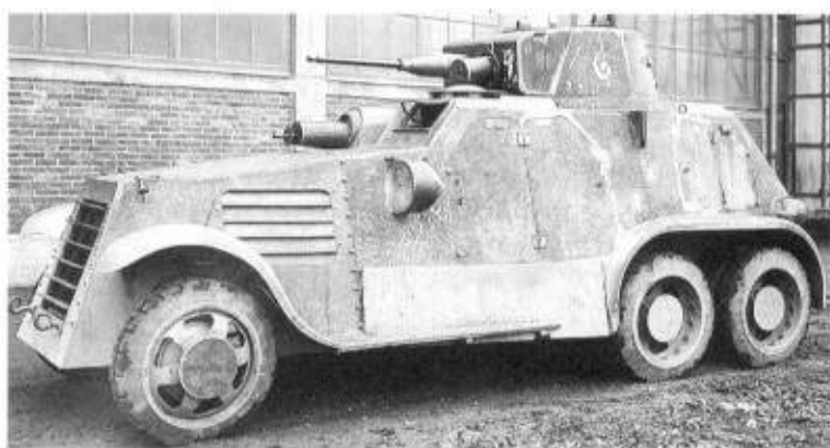
Top: The Swedish-built Landsverk 181 armoured car used a Scania Vabis 6x4 truck chassis and mounted a 20mm gun in conventional looking turret. (TM)
