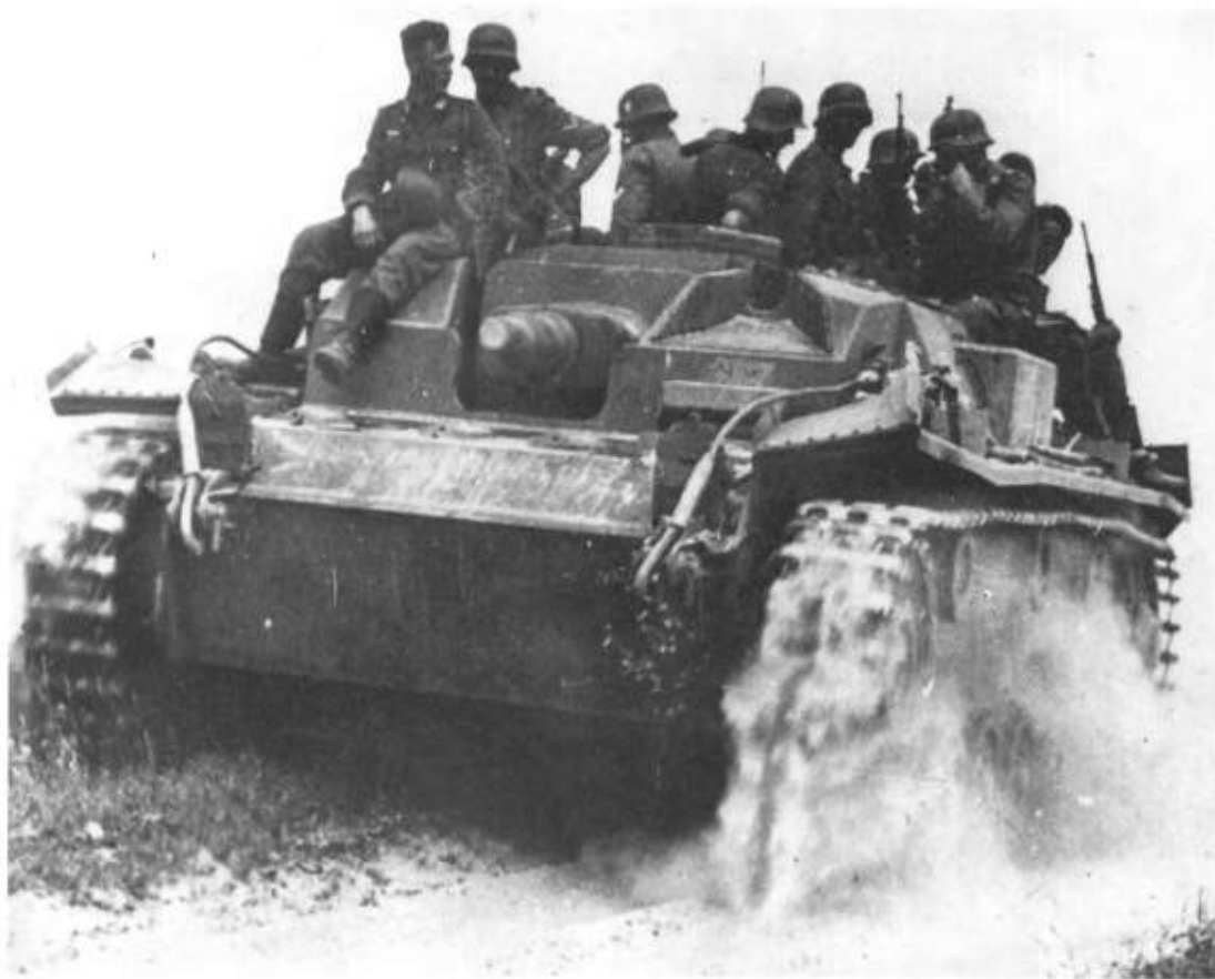
Left: Stug III Ausf A/B assault gun mounting a 7.5cm StuK 37 L/24 gun. This one is carrying Panzergrenadiers into action. (TM)
