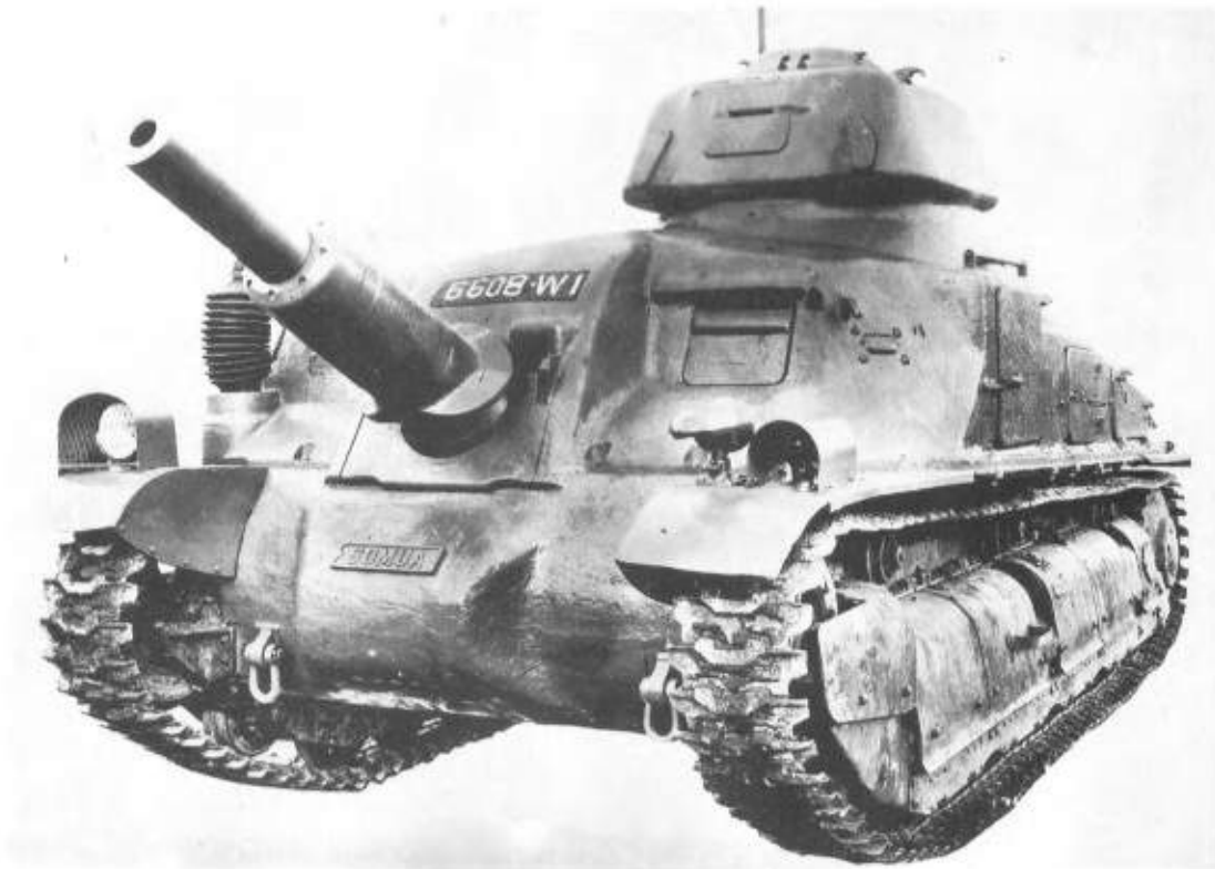
Right: The Somua SAU 40 mounted a 75mm gun in the front of a cast hull, with a Char B turret offset to the left. (TM)
