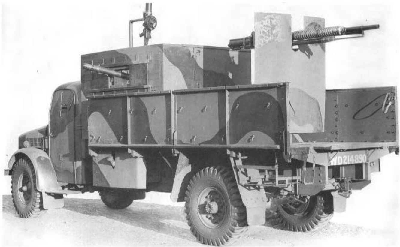
Above: Armadillo MkII mounted a 1.5 pounder COW gun in a blockhouse, with up to three Lewis guns (one on an AA mount), plus a rear-mounted heavy machine gun. One of a number of slightly different models converted from Bedford 3-ton chassis. (TM)
