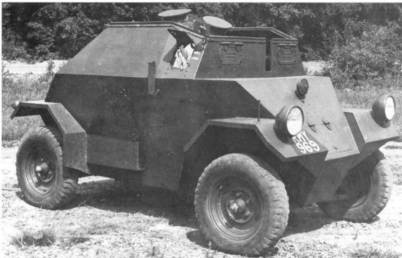
Above: Prototype Alvis Dingo scout car. This was one of the two versions produced by Alvis to meet the Mechanisation Board's specifications. It weighed around 2 tons. (TM)
