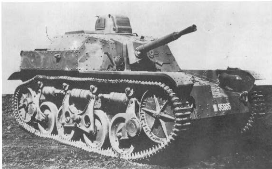
Right: Both the AMR 33 and AMR 35 were used to mount small calibre guns, this is the AMR 35 with a 25mm cannon. Note the small command cupola. (TM)
