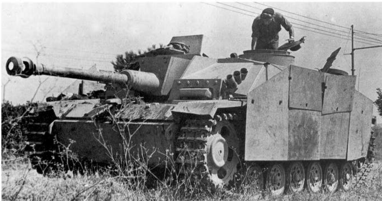
Above: Last model of the Stug III was the Ausf G which had better vision devices for the commander and a shield for the MG 34 located by the loader's hatch. Over 7,700 were built, far more than any other model. (TM)
