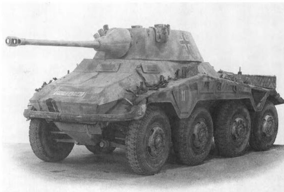
Above: SdKfz 234/4 Brad, mounted a 7.5cm PaK40 gun to provide close anti-tank support to other armoured cars. This one is displayed in the Panzer Museum, Munster, Germany.
