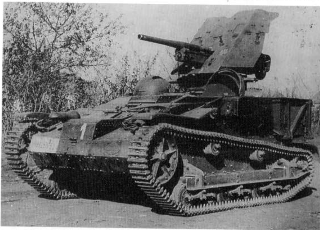
Left: This Chenillette has been modified into a mobile anti-tank gun by the Germans, who fitted a 3.7 PaK 35/36. (TM)
