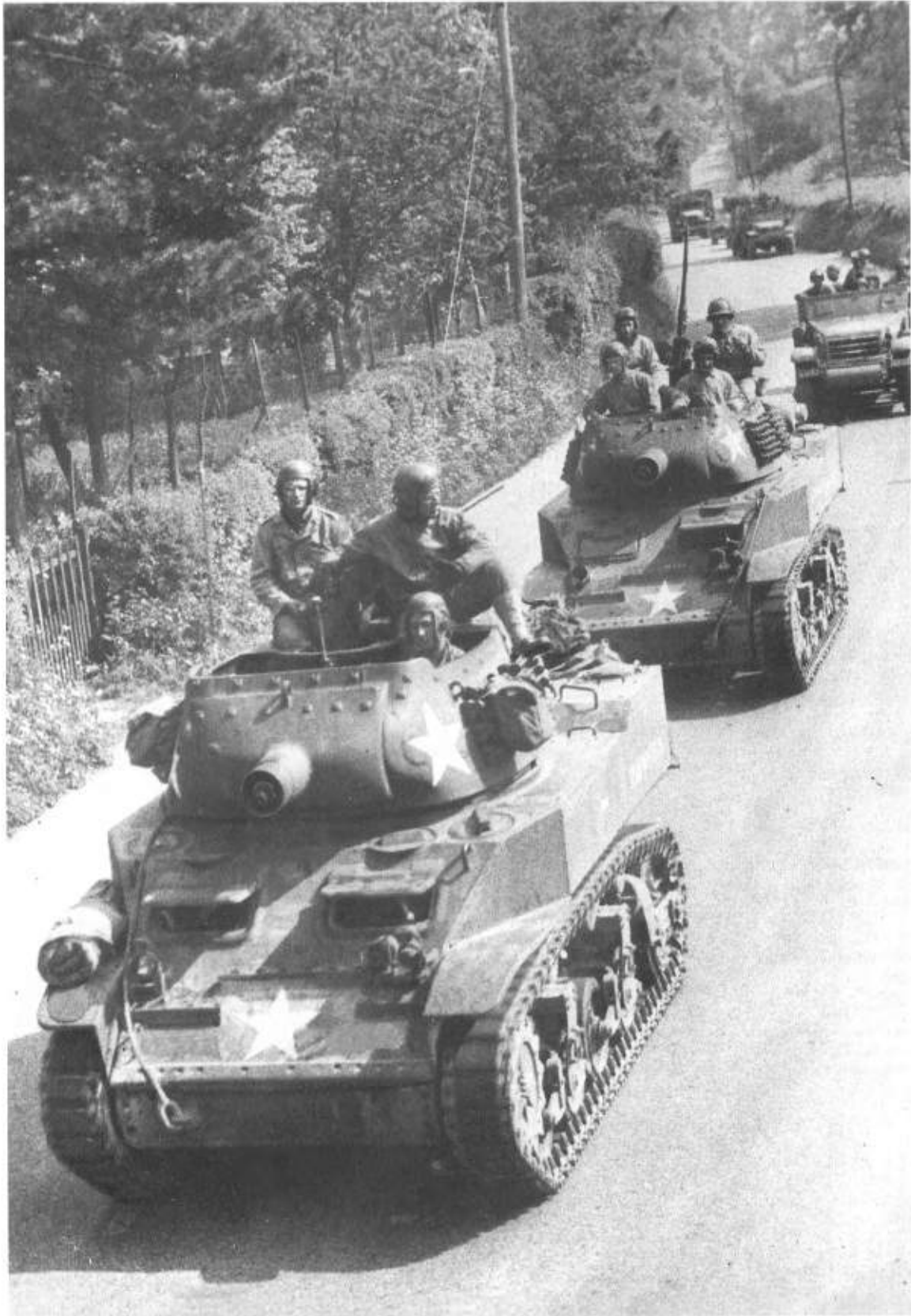
A US Army convoy, led by two M8 HMC self-propelled howitzers, passes down a country lane in England, May 1945. (TM)
