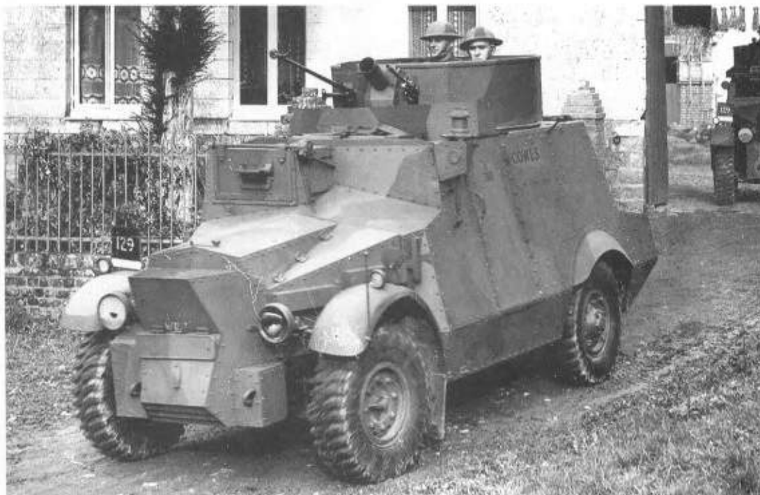
Left: A Morris CS9/LAC in France, 1940. The car, from C Squadron, 12th Royal Lancers, bears the unit code number 129 in white on a black background with a white bar, denoting Army troops. It is armed with a Bren and a Boys anti-tank rifle, both being dismountable. Note also the centrally-mounted smoke discharger. (TM)
