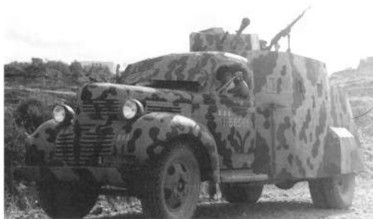
Above: Free French Forces locally modified commercial trucks into armoured vehicles. The one shown was used in Syria. (TM)
