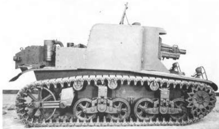
Above: The T18 HMC, (Howitzer Motor Carriage) mounted a 75mm howitzer in a massive cast hull on a M3 light tank chassis. (TM)
