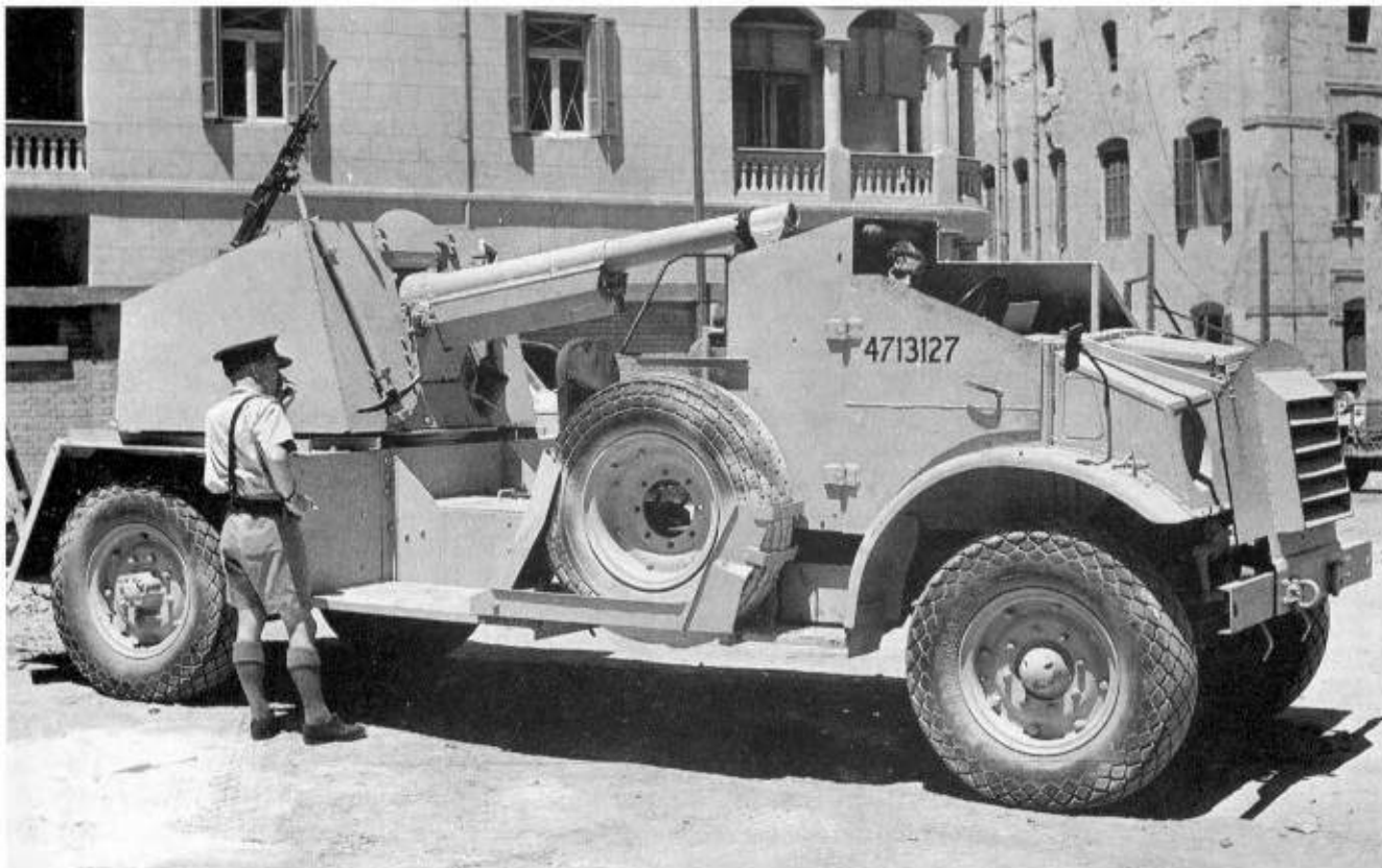
Below: A Canadian CMP 4x4 3-ton truck converted to a SP gun by fitting a French 75mm gun and extra armour. It was used by Free French Forces in North Africa, 1944. (TM)
