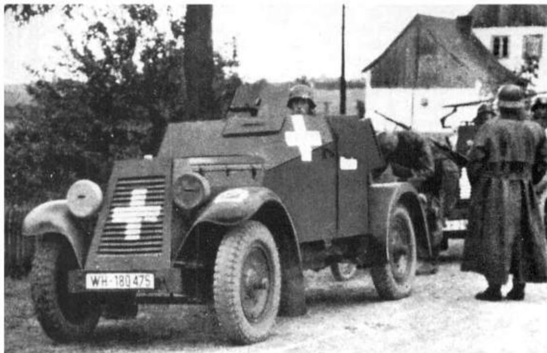
Right: The Maschinengewehr kraftwagen Adler Kfz 13 was the first of the new type of small reconnaissance vehicles, built by Adlerwerke in 1932 for the rapidly expanding German Army. (TM)
