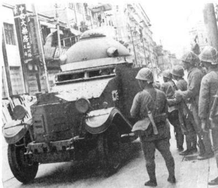
Below: The Type 87 was modernised by fitting pneumatic tyres. This vehicle is in service with the Imperial Japanese Navy (note flag). (TM)
