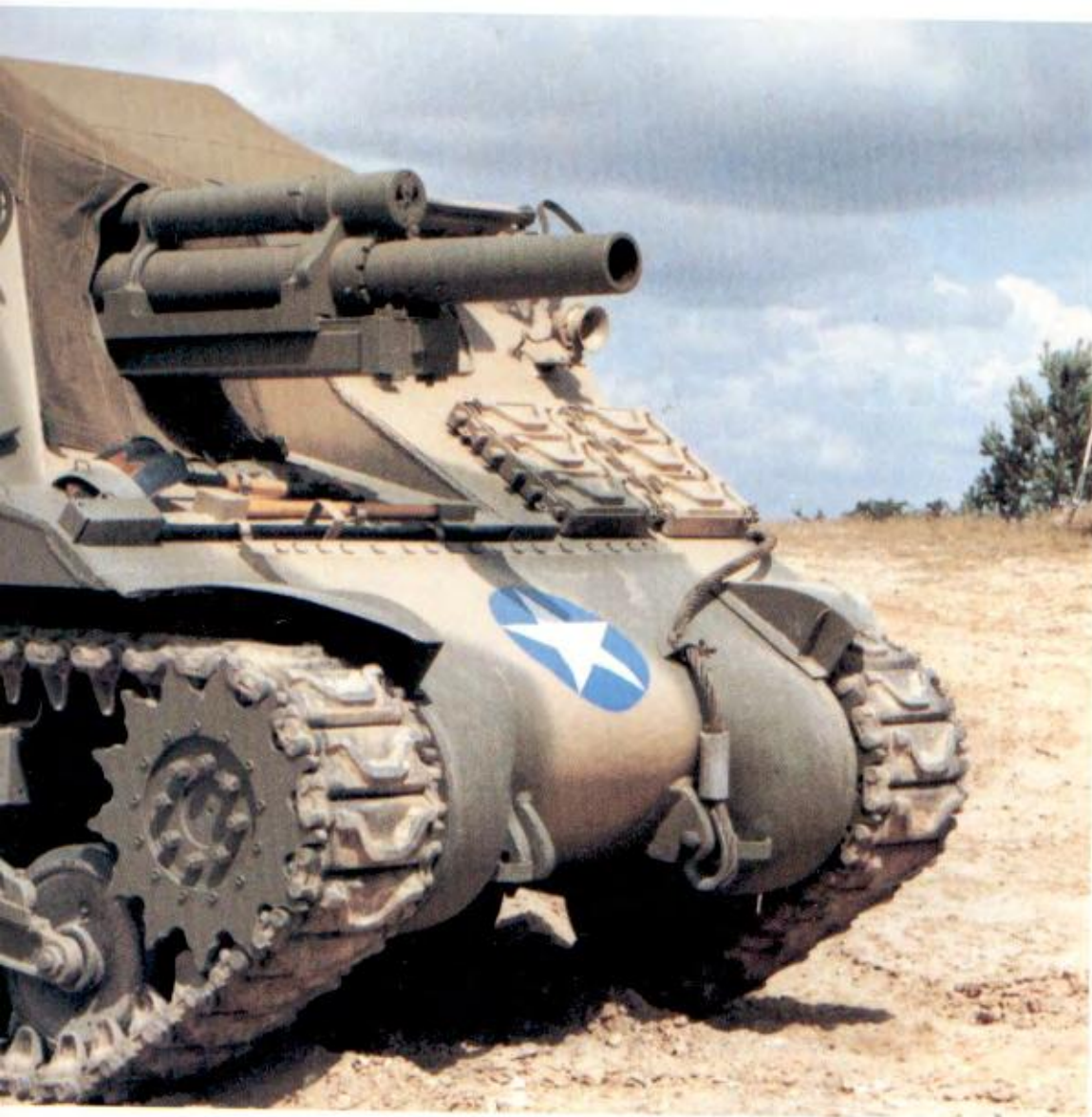
Left: A privately-owned (part of the AF Budget Collection) M7 Priest HMC, mounted a 105mm howitzer. It became the standard equipment of artillery battalions in US Armored Divisions. (TM/Roland Groom)
