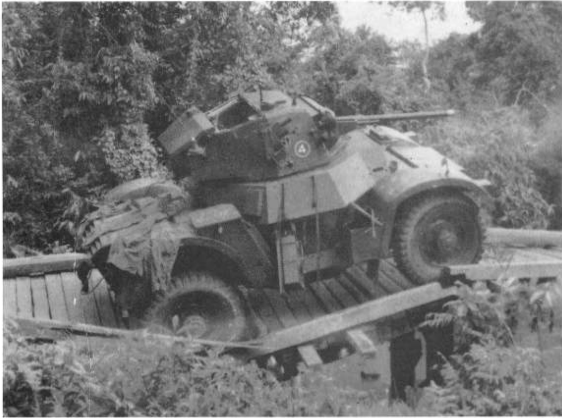
Below: An AEC Mki heavy armoured car, which mounted a 2 pounder gun and co-ax BESA, in a two-man turret very similar to that of the early Valentine tank. (TM)
