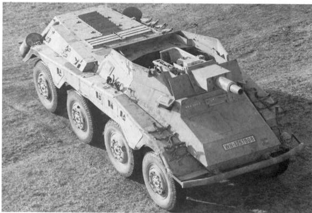
Left: The SdKfz 234/3 8rad mounted the short-barrelled 7.5cm KwK 51 L/24 gun – under ninety were built. (TM)
