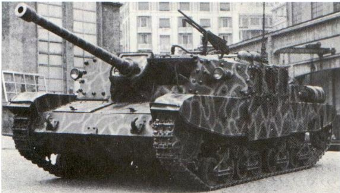
Right: The Semovente M43 DA 75/46 never saw Italian service, being built after the surrender in 1944/45 for the Germans (StuG M43 mit 75/46 852(i)). It mounted the powerful Italian 75/46 anti-aircraft gun. (TM)
