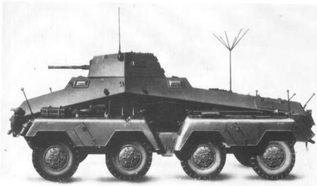
Left: This SdKfz 232 Brad (Fu) is fitted with a single rod-type aerial on the turret and a star-shaped aerial on the rear deck. This replaced the cumbersome frame-type aerial. (TM)
