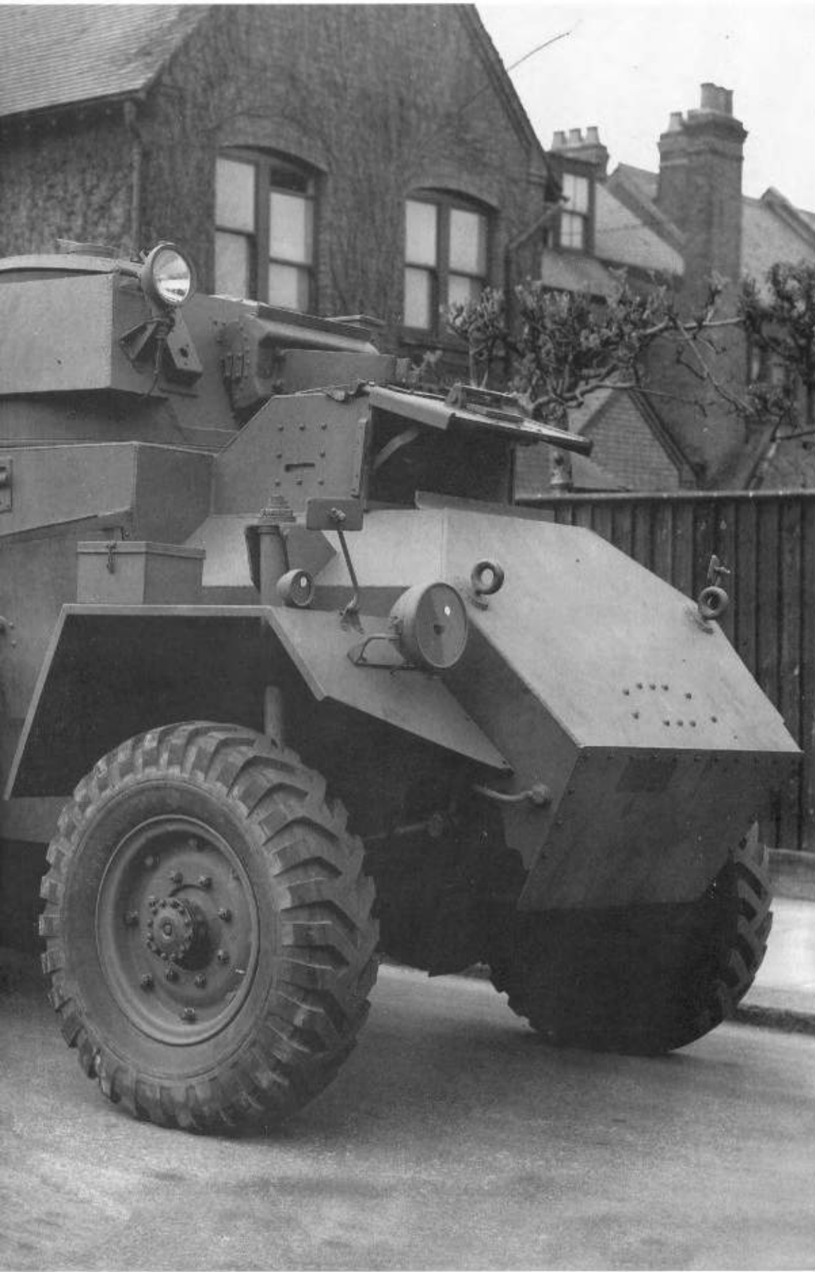
Left: The Humber Mki armoured car was designed using the pre-war Karrier KT4 artillery tractor chassis. (TM)
