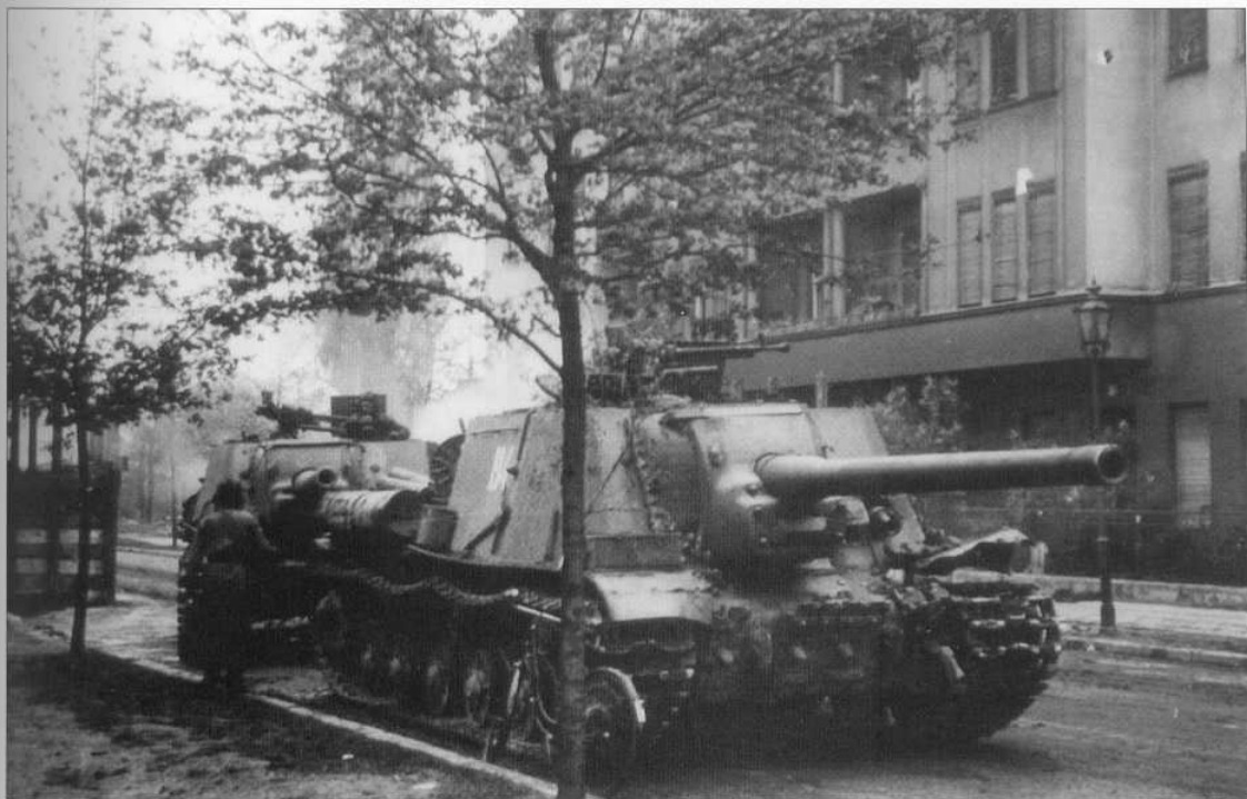
Soviet SU122 tank destroyers in a Berlin suburb. The SU tank destroyers were essentially turretless versions of tanks such as the T-34 and JS-2, in the same way the Germans produced tank-destroyer versions of their own tanks, such as the Jagdpanzer IV and Jagdpanther. (From the fonds of the RGAKFD at Krasnogorsk)
