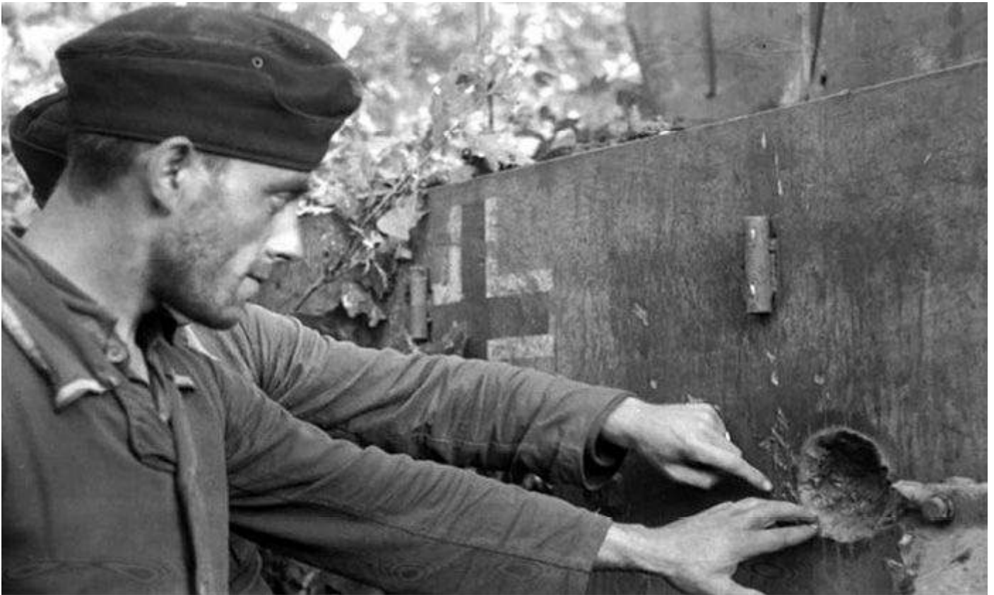
Panzer crewmen inspect the combat damage inflicted by enemy rounds which have just failed to pierce the strong side armour of the Tiger.
