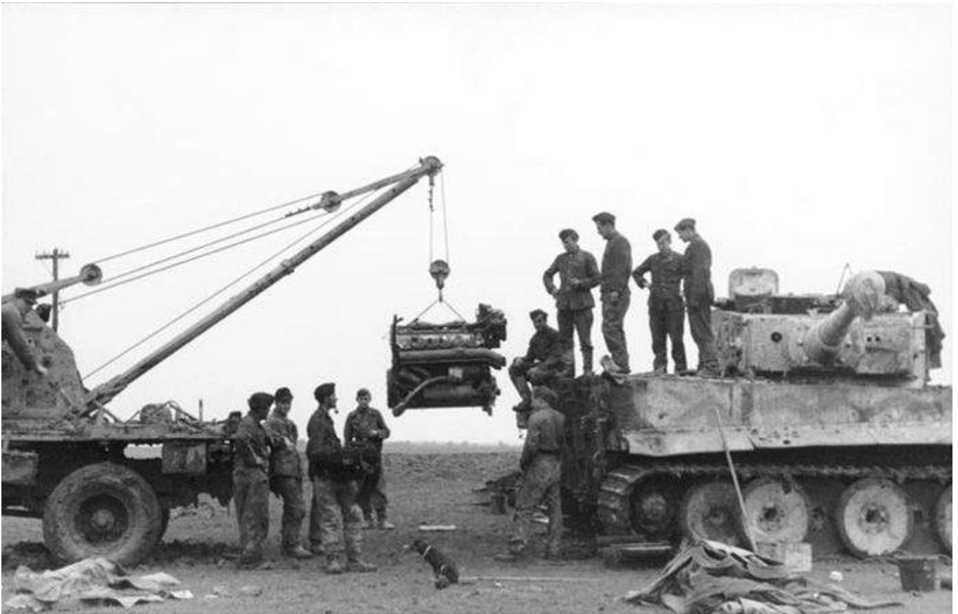
A Tiger I undergoing engine repair.
