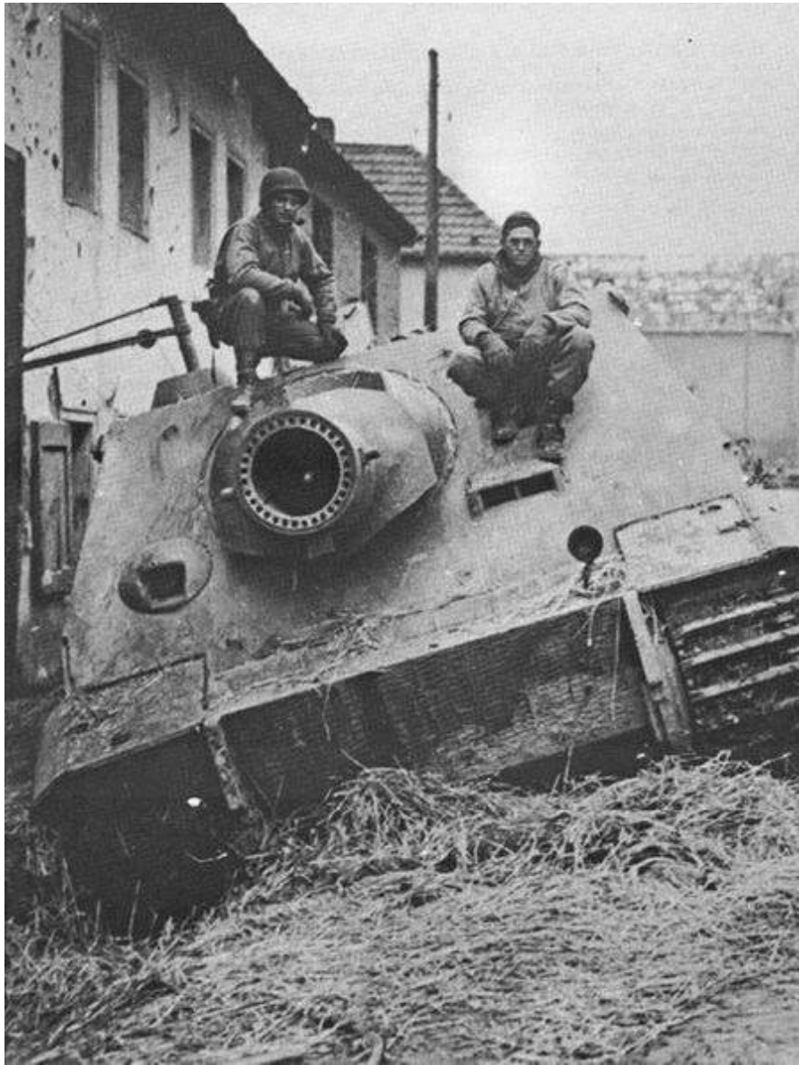
The Sturmtiger with its 15in howitzer protuding. This calibre was as great as many a battleship's big guns.
