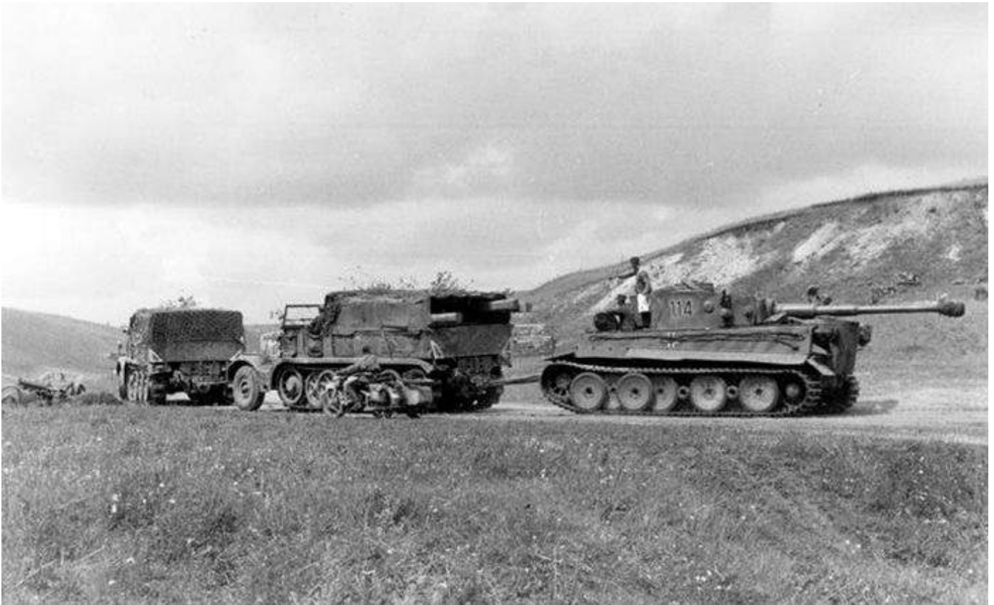
A broken down Tiger I being towed by two Sd.Kfz. 9. The convoluted arrangement was the only means by which a broken down Tiger I could be officially recovered.
