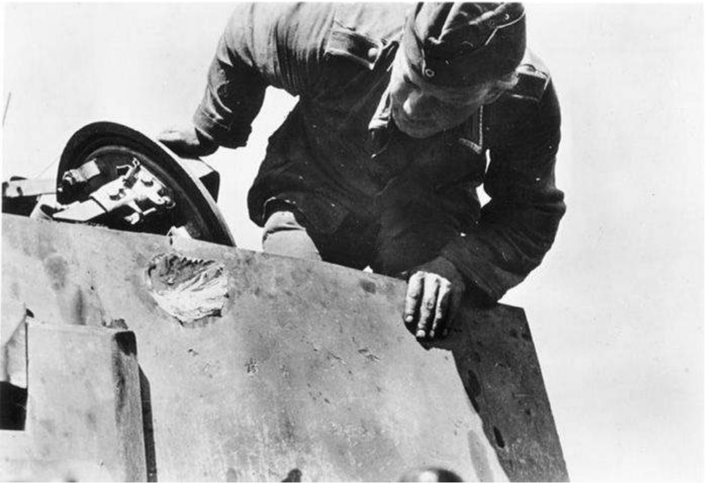
A tank man inspects the combat damage inflicted by enemy rounds which have failed to pierce the strong side armour of the Tiger tank turret.
