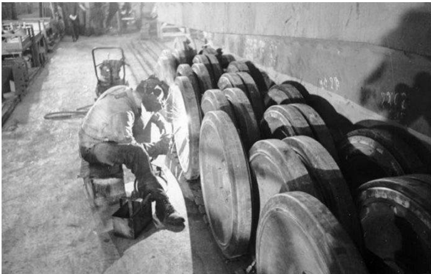
The cumbersome road wheel assembly of the Tiger I can be clearly seen in this photograph taken at the Henschel works. It is easy to understand why these wheels could become jammed solid with mud, ice or snow requiring huge efforts to repair.
