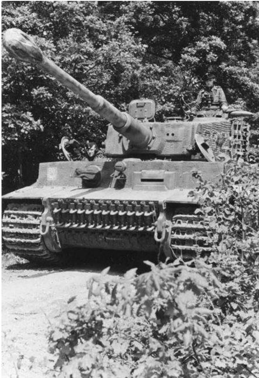
A Tiger which has received a coating of anti-magnetic Zimmerit coating designed to prevent the application of magnetic mines by tank hunting teams.
