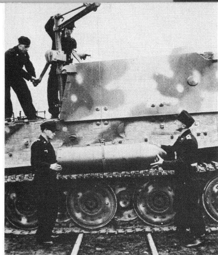
Loading ammunition into the Sturmtiger. The rocket is put down to the right of the launcher. After the packing material is removed, the sling of the loading crane is attached. The projectile is raised by using the hand crank of the crane and lowered into the interior through the opened ammunition loading hatch.
